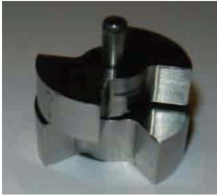
Figure 17.6. Close-up of straight rotor mini-siren.
