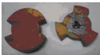
Figure 9.16a. Wood prototypes used for torque and erosion testing.
