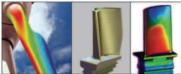
Figure 8.17c. Blade twist, aerospace designs (pressure variations in spanwise direction clearly evident).
