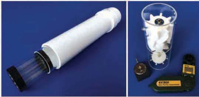
Figure 16.28a. Flow straightener, wind anemometer and force gauge.
