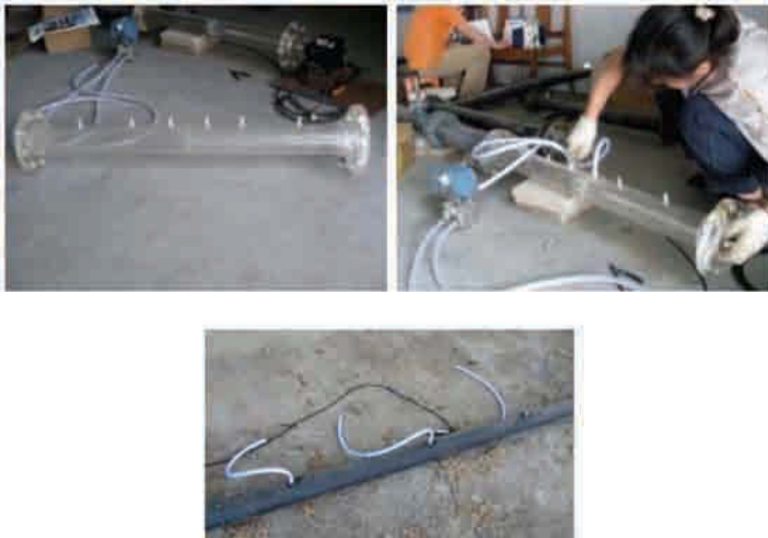
Figure 1.5n. Distant multiple transducer array setup.
