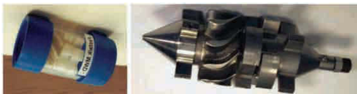
Figure 9.16b. Wind tunnel forerunner to turbosiren (U.S. Patent 5,831,177).
