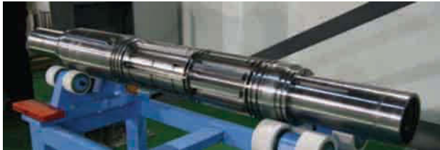
Figure 12.1-7. Near-bit measurement sub.
