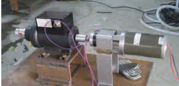
Figure 1.5j. Torque, position and rpm counter.
