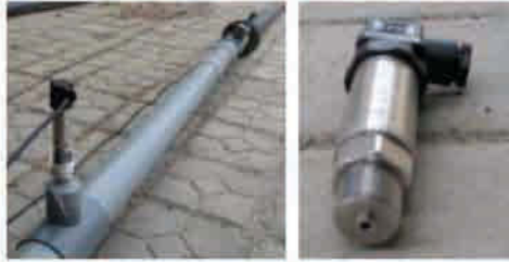
Figure 1.5m. Single piezoelectric transducer closest to siren for constructive interference and nonlinear harmonic generation study.
