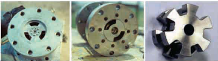
Figure 9.14. Siren test concepts, test section for both air and mud.
