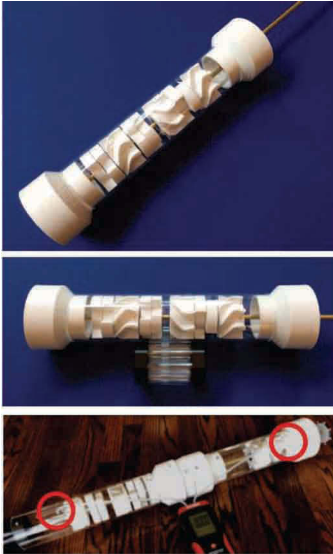
Figure 16.13. Three-stage turbosiren (pressure ports for \Delta p measurement circled at left and right).
