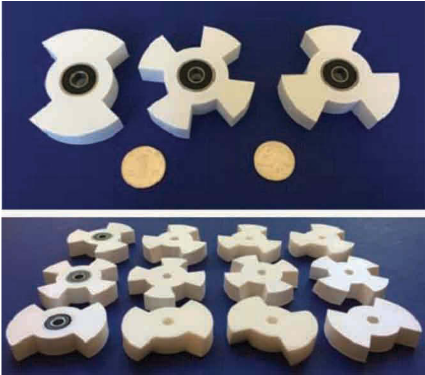
Figure 16.18. Rotors and stators with different lobe numbers and tapers (a Chinese yuan and a United States quarter, top).
