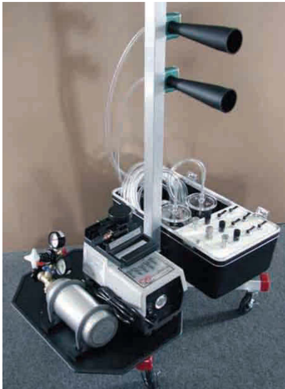
Figure 14.7. Neutrally buoyant helium-filled soap bubbles flow past tool prototype to visualize erosion-causing fluid paths – inexpensive modeling clay modifications are rapidly re-tested, useful fixes are identified, and refined hardware is shipped for more comprehensive field evaluation.
