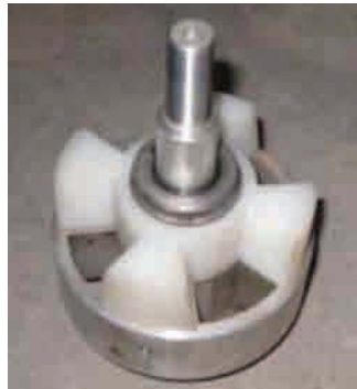
Figure 7.3. A “stable-closed” four lobe siren used in flow loop tests.
