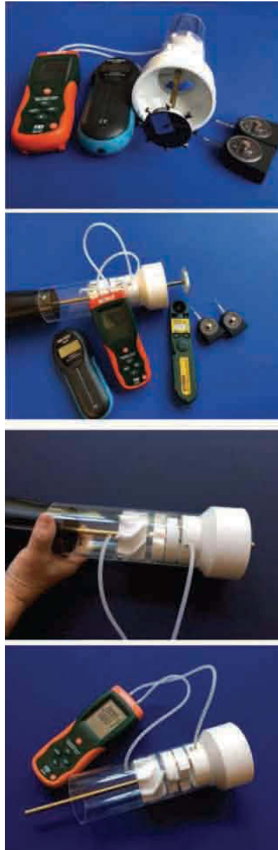
Figure 16.10. Differential pressure signal measurement.
