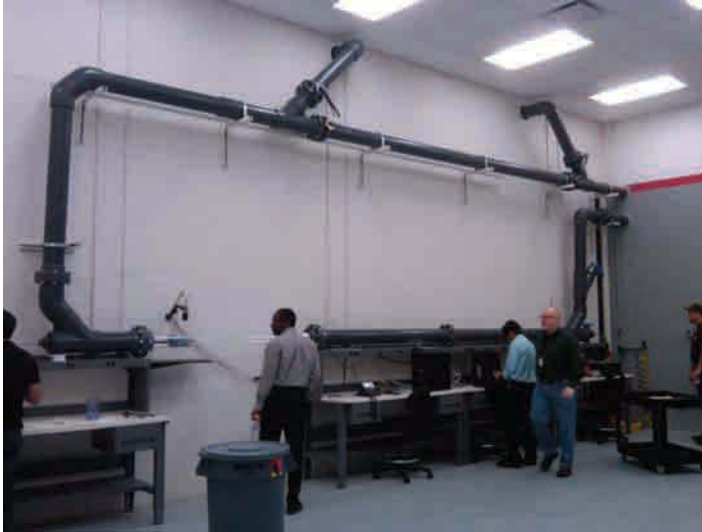
Figure 14.2. Short wind tunnel for torque, erosion and signal testing.
