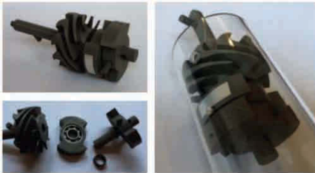
Figure 13.7. Disassembled turbosiren prototype (rotor reflective tape for optical tachometer measurements).
