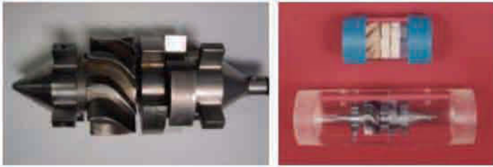
Figure 9.4c,d. Self-spinning “turbosiren” designed in wind tunnel and validated in mud flow loop (U.S. Patent 5,831,177).
