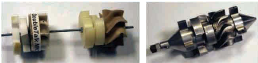
Figure 9.23. Turbosirens in series (U.S. Patent 5,831,177).
