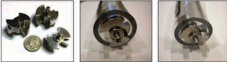
Figure 1.5e.1. Siren concepts, miniature sirens for slim tools (the United States quarter shown is similar to the one-yuan Chinese coin).
