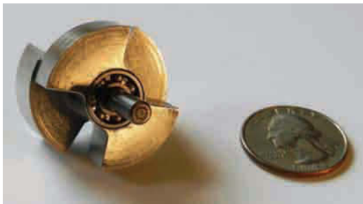
Figure 17.3. Mini-siren, about one inch across, with low friction bearings (the quarter is about the size of a Chinese yuan).
