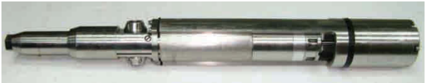
Figure 1.1a. Prototype single-siren tool (assembled).
