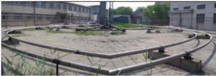
Figure 9.2b. Long wind tunnel system with pressure transducers (see Figure 1.5b.1 for additional photos).
