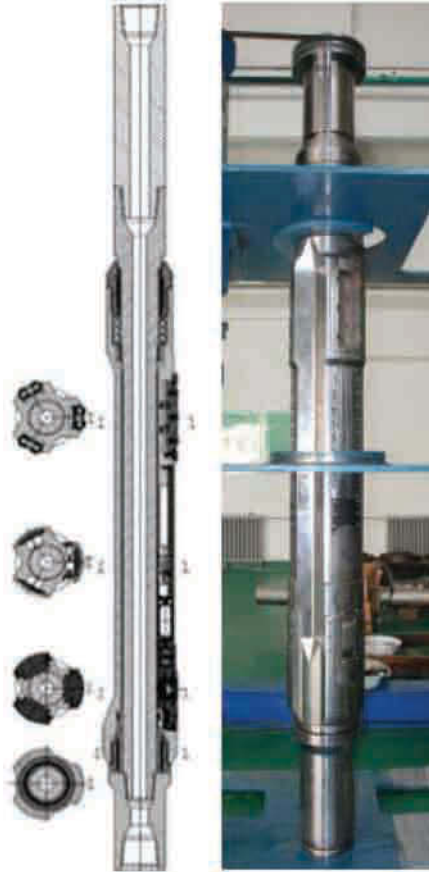
Figure 12.9-1. DRVDS-1 tool architecture and hardware.
