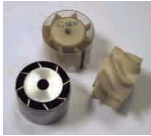
Figure 8.17b. Turbine prototypes with and without shroud.
