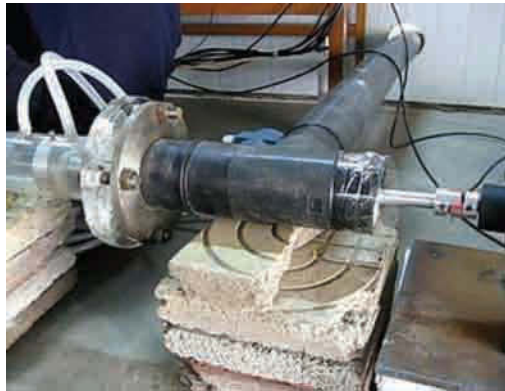
Figure 1.5s. Short wind tunnel, with long wind tunnel connection.
