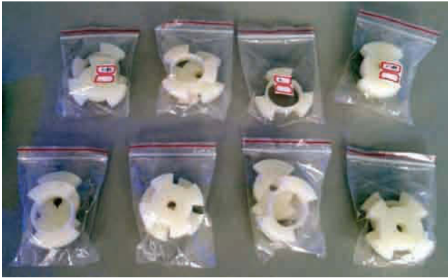
Figure 13.6. Sample rotor and stator prototype test pairs (two, three and four lobe designs shown).
