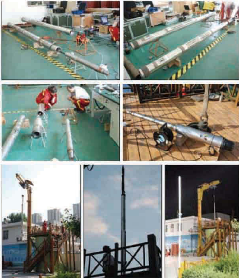
Figure 12.5-2. Well calibration -Indoor adjustments and tank test.
