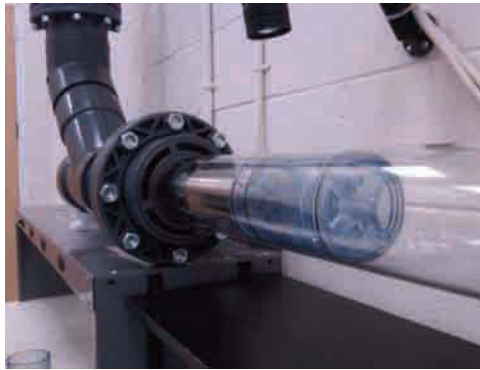
Figure 14.5b. Wind tunnel test section with test prototype.
