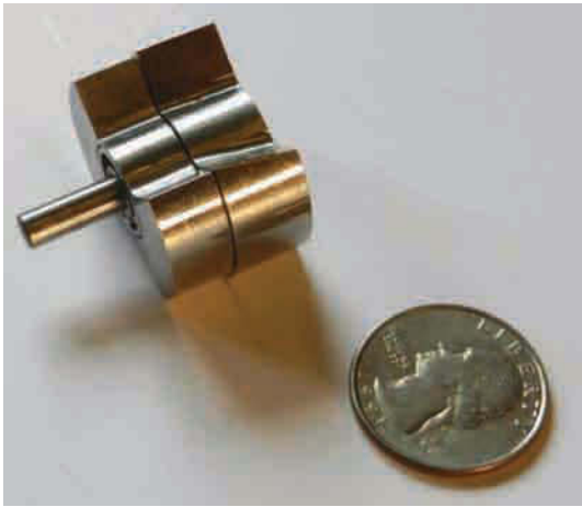
Figure 17.4. Downstream rotor with parallel tapers.
