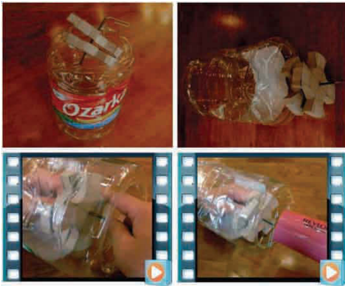
Figure 17.13. Siren installed in open plastic bottle, with hair dryer used to identify “stable closed” properties.
