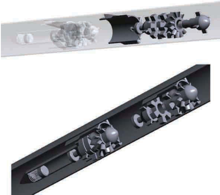
Figure 16.15. Two-stage turbosiren with pressure compensation module.
