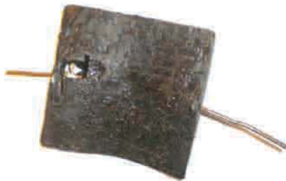
Figure 8.19. Flexible rubber airfoil with copper skeleton.
