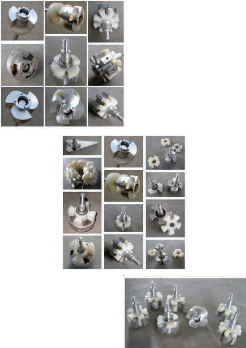
Figure 1.5d.1. Siren concepts tested in wind tunnel (standard size).
