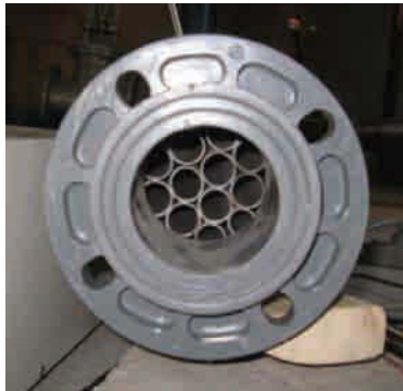
Figure 1.5f.1. Flow straighteners for upstream and downstream use.
