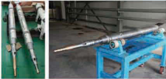
Figure 12.8-3. 6.75 in (left) and 4.75 in (right) downhole annular pressure measurement sub.
