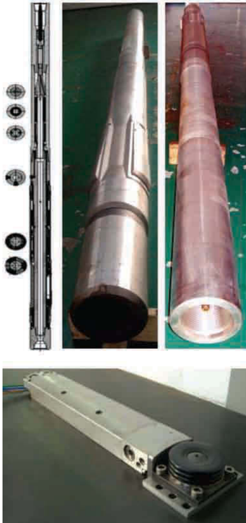
Figure 12.10-1. DRVDS-2 tool architecture and hardware.
