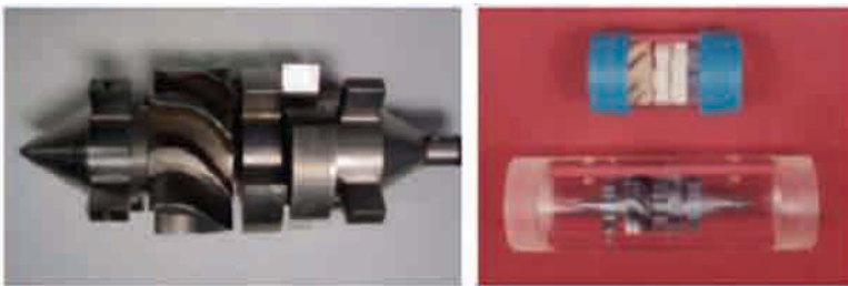
Figure 16.6. Turbosiren hardware and wind tunnel prototype.
