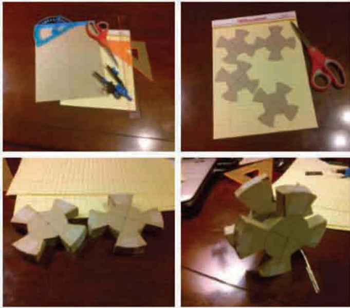
Figure 17.12. Cardboard siren with paper clip shaft.
