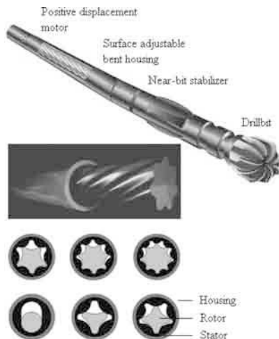
Figure 6.2a. Positive displacement motor (see noise spectra in Figure 6.8a).
