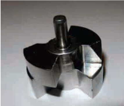
Figure 17.7. Close-up of notched mini-siren design.
