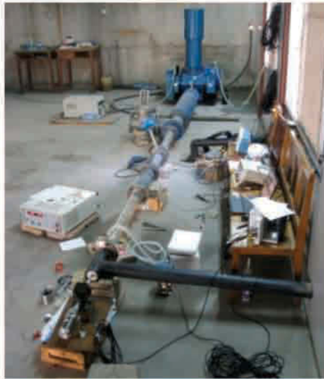
Figure 1.5a.1. Short “hydraulic” wind tunnel, or simply “short wind tunnel.”
