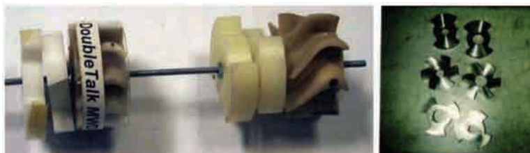
Figure 9.16c. Sirens in series (left) and “swept” rotors (right, middle).
