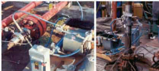
Figure 9.17. Wind test fixture used in mud and field tests (Gardner, 2002).
