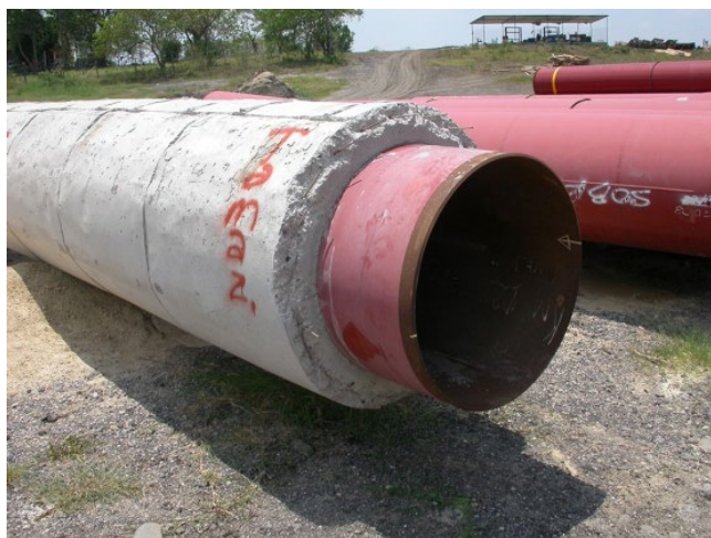
Figure 8.91 Concrete weight coating on the exterior of pipe intended for submerged service.
