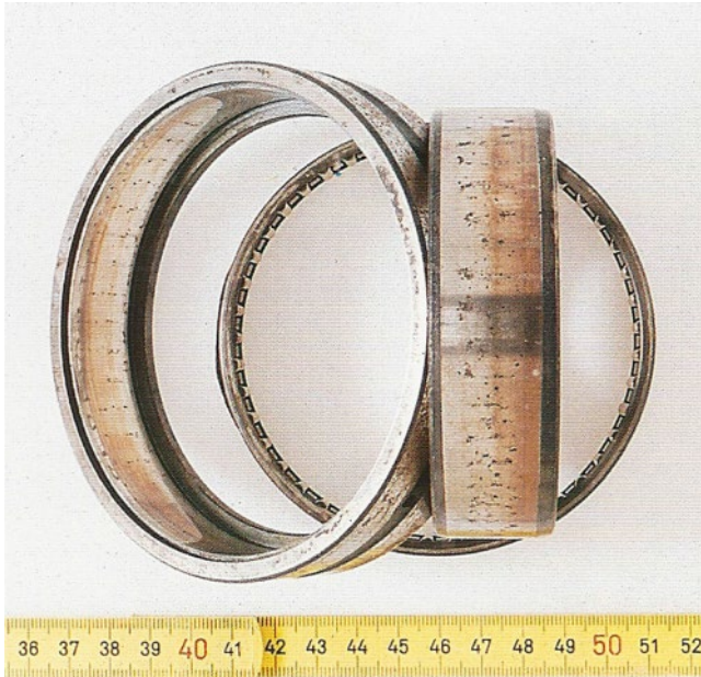
Figure 5.114 Fretting corrosion on roller bearing race. Source: Bogaerts [82]. Reproduced with permission of NACE International.
