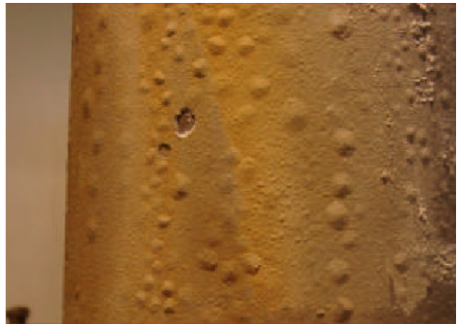
Figure 6.66 Blisters on heated unsealed TSA aluminum [82]. Source: Reproduced with permission of NACE International.
