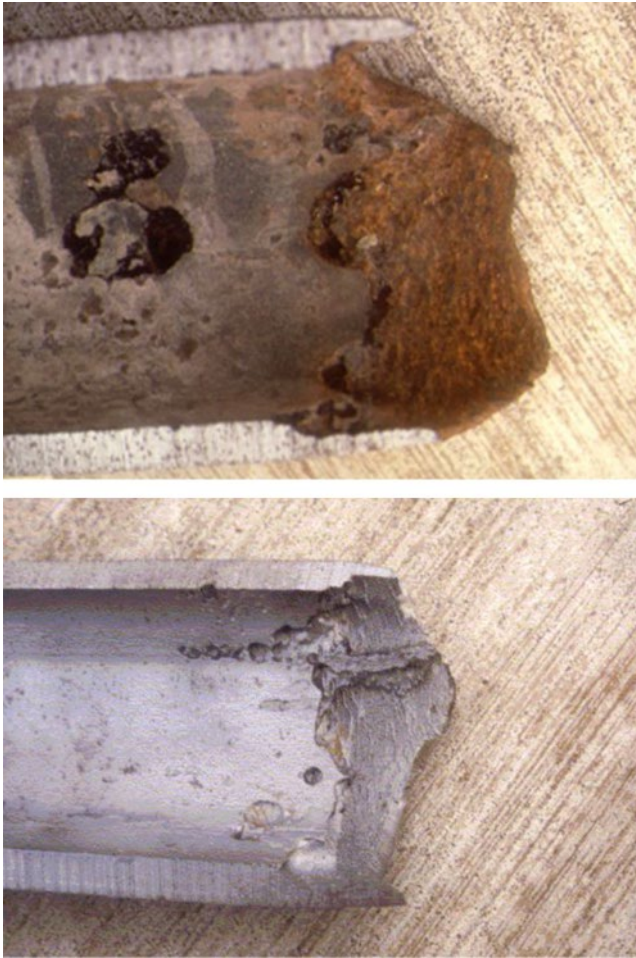
Figure 5.73 Eroded downhole tubing from an offshore production platform.
