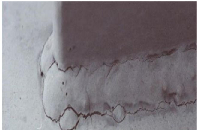
Figure 6.58 Typical mud cracking in thick coatings [73]. (a) Cracking starting at edges. (b) Cracking of thick coating at welded connection. Source: Reproduced with permission of NACE International. NACE CIP 1–5.
