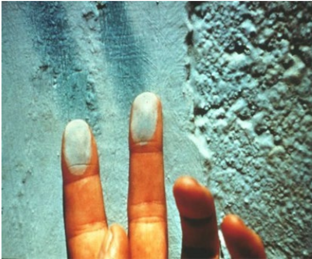
Figure 6.52 Superficial chalking on a coating surface. Source: Reproduced with kind permission of Brendon Fitzsimons, FITZ-COATINGS Ltd.
