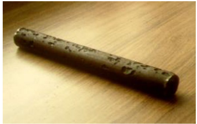
Figure 3.29 Mesa corrosion on a sucker rod.
