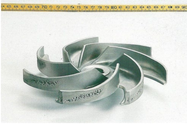
Figure 5.72 Erosion corrosion due to cavitation on a stainless steel pump impeller. Source: Bogaerts [82]. Reproduced with permission of NACE International.
