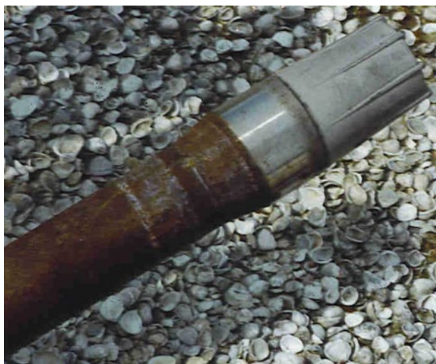
Figure 4.50 External corrosion of 13Cr L80Cr tubing stored outdoors for several years.
