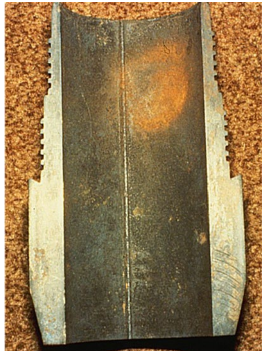
Figure 8.27 Wireline damage to the internal coating on drill pipe. Source: Byars [26]. Reproduced with permission of NACE International.
