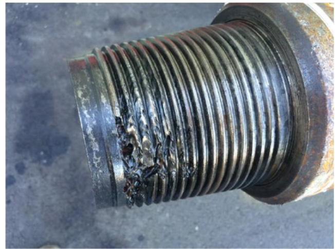
Figure 8.5 Washout near the threads on an oilfield drill pipe.
