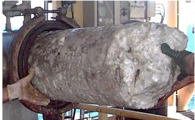
Figure 3.44 Hydrate plug removed from a subsea pipeline. Source: Photo courtesy Dendy Sloan, Colorado School of Mines.
