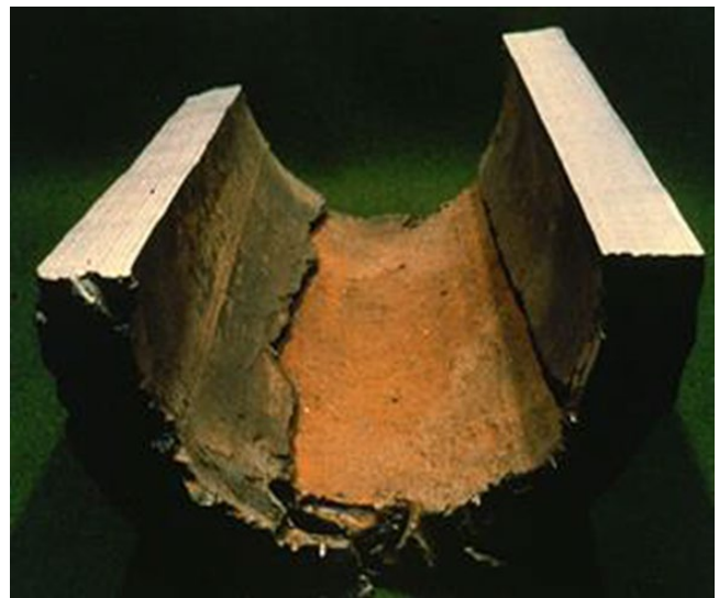
Figure 3.30 \text{CO}_2 channeling along the bottom of a horizontal gathering line.
