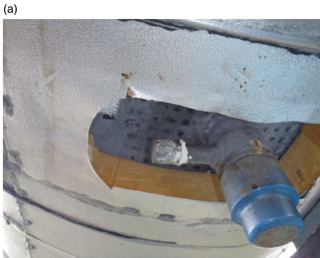
Figure 7.12 Markings where ultrasonic inspection readings have been made on crude oil piping. (a) At a corrosion inhibitor injection port. (b) After insulation has been removed on overwater piping at a marine terminal.
