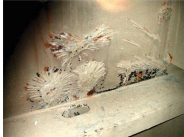
Figure 6.51 Protective coating cracks that radiate from the point of reverse impact and will eventually lead to corrosion [69, 70, 73].
