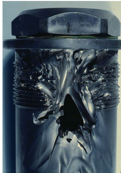
Figure 5.66 Eroded wellhead component. Source: Byars [9]. Reproduced with permission of NACE International.
