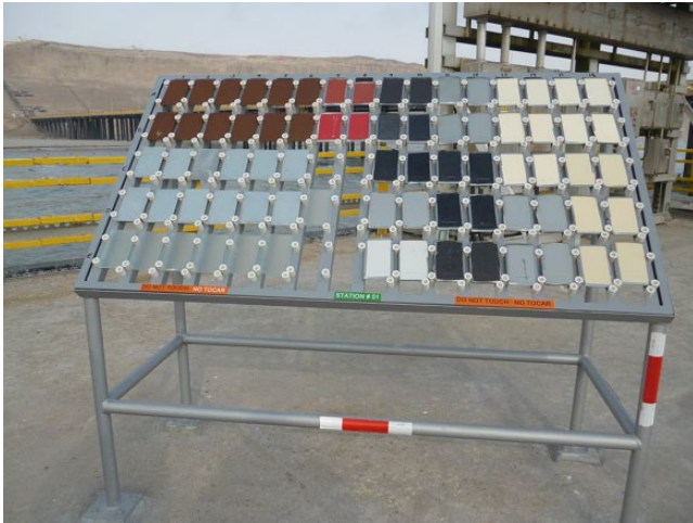
Figure 3.6 Atmospheric exposure panels at a large seaside petrochemical facility.
