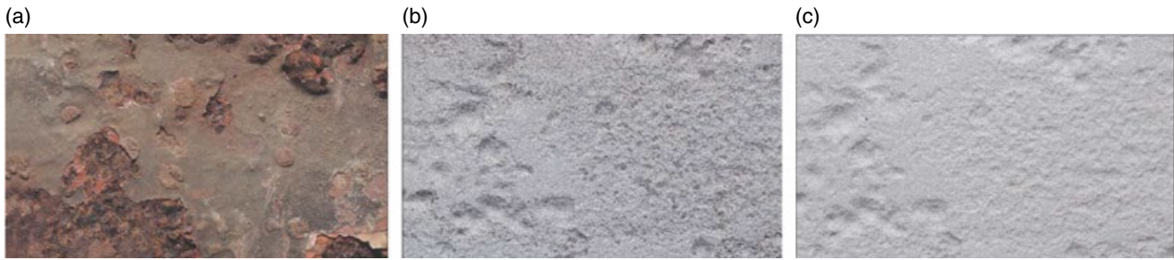
Figure 6.6 Standard images from left-to-right of deeply pitted steel surface. (a) Before dry abrasive blasting, (b) cleaned to near-white, and (c) cleaned to the white metal condition [16, 17].
