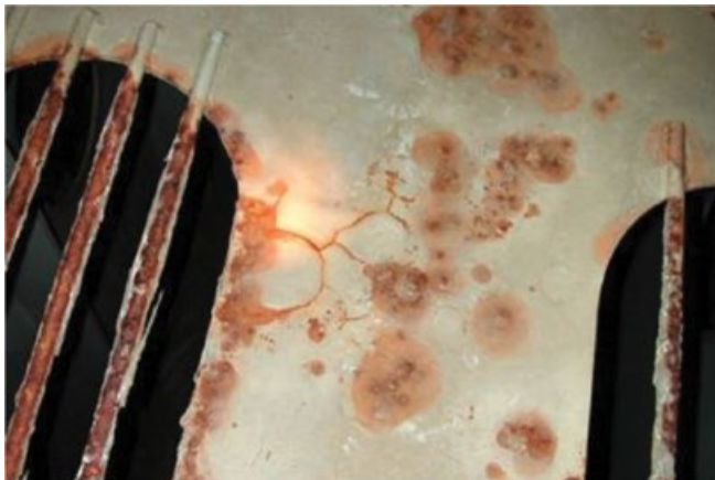
Figure 6.58 Typical mud cracking in thick coatings [73]. (a) Cracking starting at edges. (b) Cracking of thick coating at welded connection. Source: Reproduced with permission of NACE International. NACE CIP 1–5.
