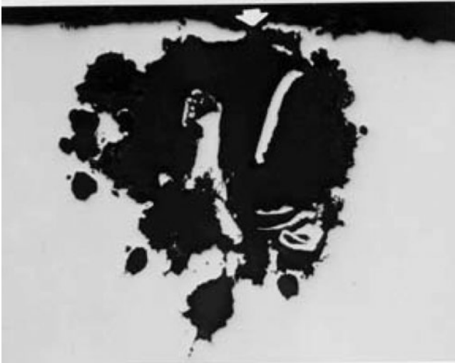
Figure 5.33 Pitting on stainless steel tubing. Source: McDanels [45]. Reproduced with permission of ASM International.
