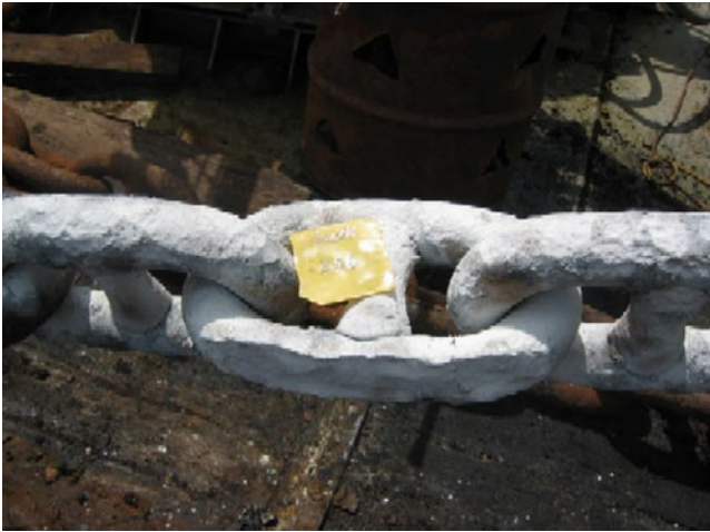
Figure 3.43 MIC on an ocean-bottom mooring chain [37]. Source: Reproduced with permission of Elsevier.
