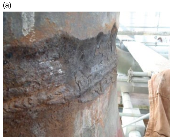
Figure 3.24 Corrosion at uncoated weld on the crude oil piping system shown in Figures 3.22 and 3.23. (a) Corrosion exposed when jacketing and insulation was removed. (b) Ultrasonic inspection markings indicating that greater than 75% wall loss had occurred in some locations.
