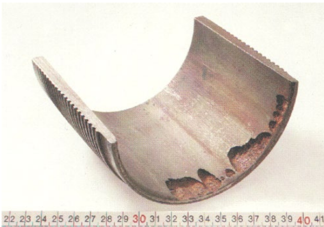
Figure 5.101 Mesa corrosion at a threaded connection on downhole tubing. Source: Bogaerts [82]. Reproduced with permission of NACE International.
