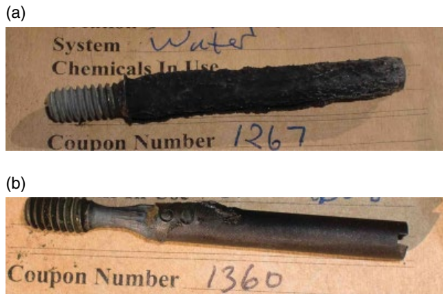
Figure 7.34 Iron sulfide (FeS) deposits on ER probes. (a) Probe with intact scale on the surface. (b) Different probes with scale removed to show extensive underdeposit corrosion.
