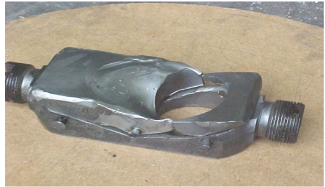
Figure 8.36 Erosion of a gate valve component producing loss of a sealing surface. Source: Photo courtesy of NACE International.
