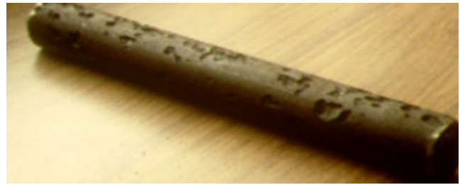
Figure 5.99 Mesa corrosion of a 9-chrome sucker rod.
