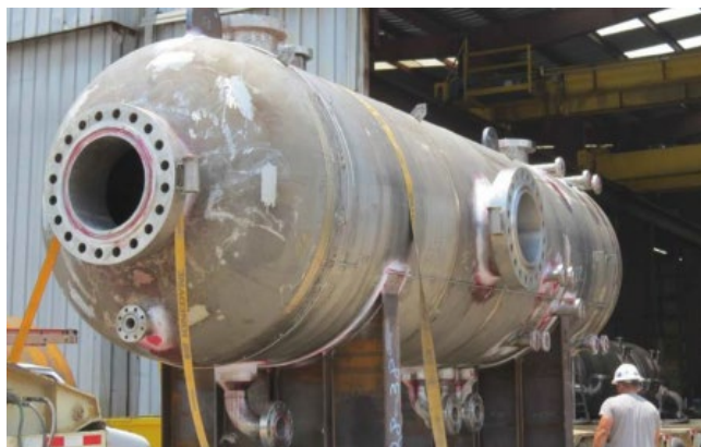
Figure 4.51 A 316 stainless steel separator to be used offshore in place of a clad vessel [90]. Source: Reproduced with kind permission of John R. Curry.
