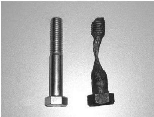
Figure 5.40 Crevice corrosion of a 10-year-old bolt on a water-control valve [55]. Source: Reproduced with permission of corrosionsource.
