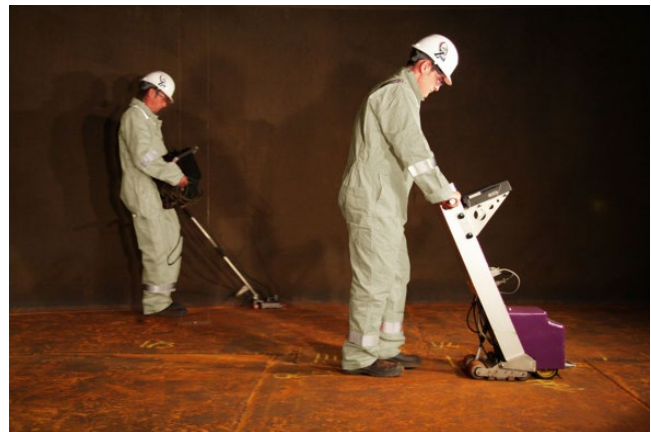
Figure 7.19 MFL inspection of a large aboveground storage tank floor. Source: Image courtesy Rosen Inspection.
