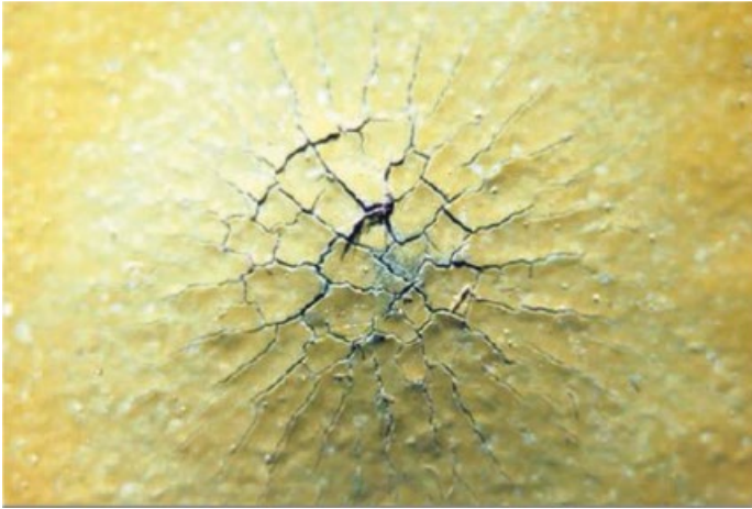
Figure 6.51 Protective coating cracks that radiate from the point of reverse impact and will eventually lead to corrosion [69, 70, 73].
