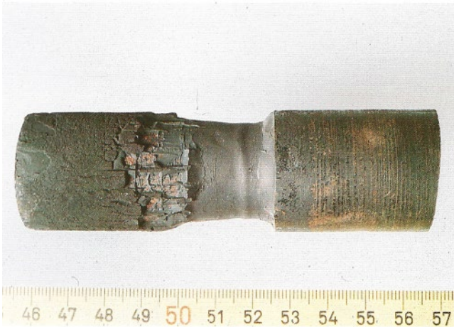
Figure 5.109 Alkali attack at crevice in boiler water system. Source: Bogaerts [82]. Reproduced with permission of NACE International.
