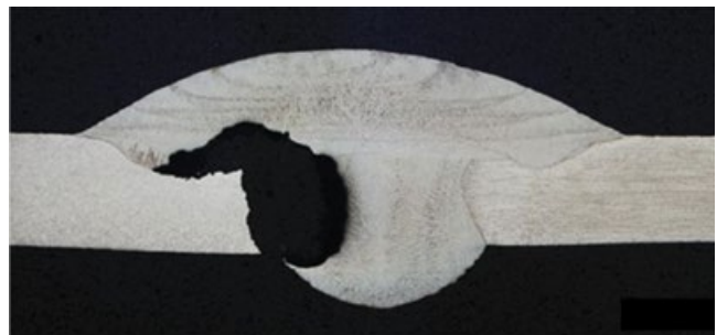
Figure 7.48 MIC pitting of stainless steel after hydrotesting in freshwater. (a) 304 stainless steel pitting at low spots that did not drain after only six weeks, and (b) weld in 316 stainless steel one year after freshwater hydrotesting.
