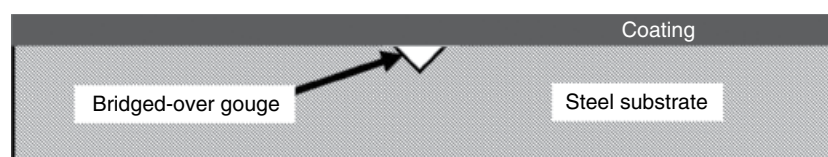
Figure 6.18 Gouge with bridged-over coating subject to moisture accumulation and corrosion.
