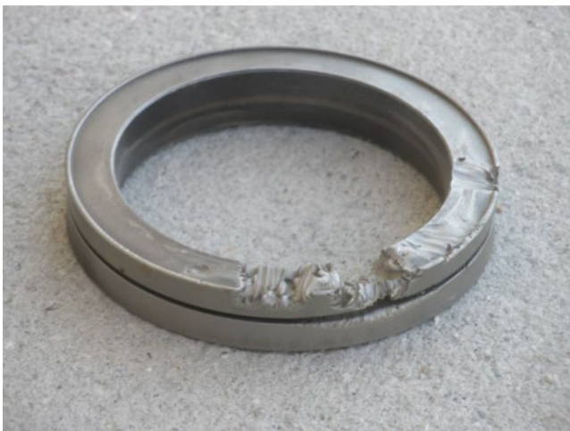
Figure 5.77 Erosion corrosion of a stainless steel seal in a steam line. Time to failure was hours.
