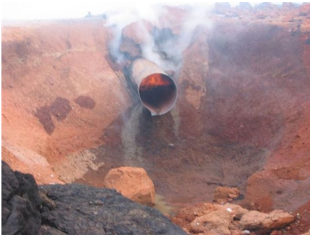
Figure 8.76 Crater caused by a natural gas pipeline explosion.
