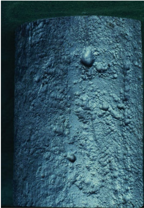
Figure 8.19 External pitting corrosion on oilfield casing.
