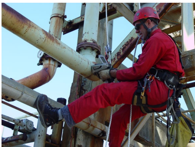
Figure 7.20 Handheld X-ray fluorescent spectrometer being used for positive materials identification. Source: Photo courtesy of Thermo Fisher Scientific.
