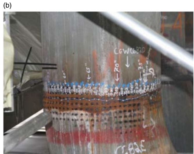
Figure 7.12 Markings where ultrasonic inspection readings have been made on crude oil piping. (a) At a corrosion inhibitor injection port. (b) After insulation has been removed on overwater piping at a marine terminal.
