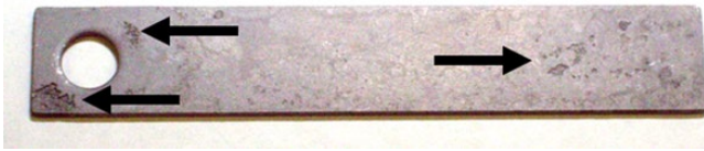
Figure 7.27 A typical weight-loss coupon after exposure to an oilfield environment for three months. Arrows indicate the three areas with pitting.
