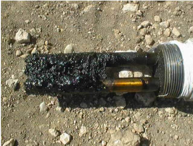
Figure 8.99 Galvanic corrosion monitoring probe removed from a crude oil pipeline. Note the paraffin and sludge deposits [231]. Source: Photo courtesy NACE International.
