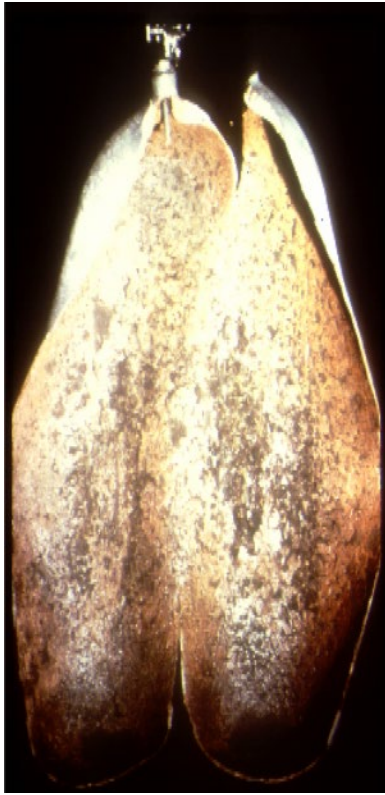
Figure 5.9 Galvanic corrosion of a scuba tank. Source: Photo courtesy NACE International.
