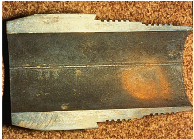
Figure 5.107 Wire line corrosion.
