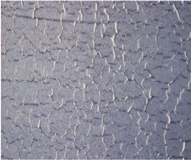
Figure 6.54 Wrinkled paint surface. Source: Reproduced with kind permission of Brendon Fitzsimons, FITZ-COATINGS Ltd.
