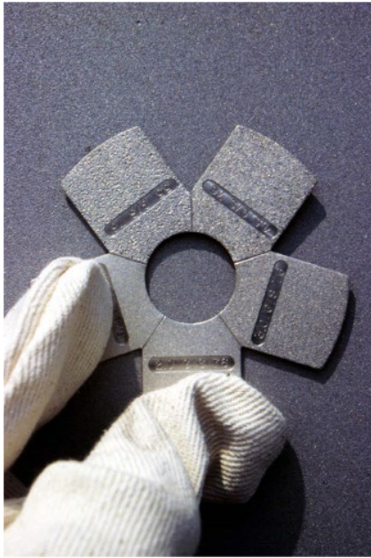
Figure 6.12 Keane-Tator surface profile comparator disc. Source: Photo courtesy of KTA-Tator, Inc., reproduced with permission.
