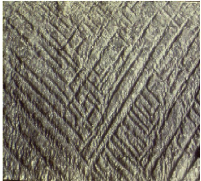
Figure 5.19 Close-up view of Lüders band corrosion on OCTG.
