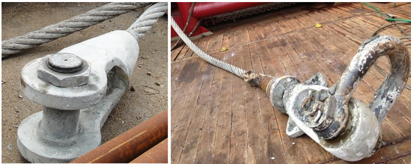
FIGURE 9.6 Open-end socket on a wire rope (left) and close-end socket on a wire rope (right).
