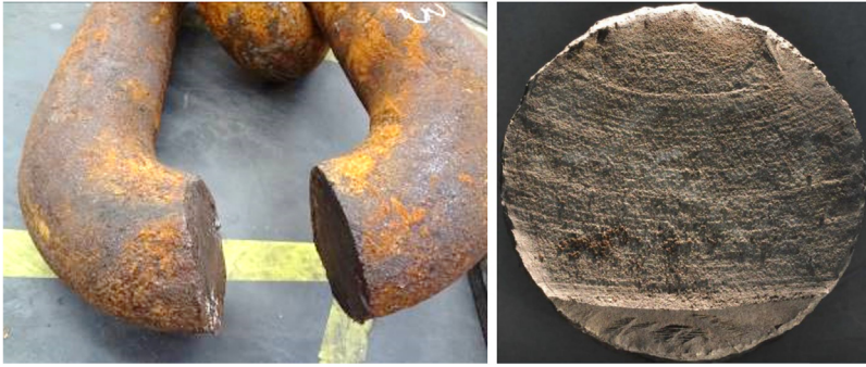
FIGURE 6.1 (Left) Chain link failed due to fatigue [6]. (Right) Broken surface showing beach marks. Courtesy: Sofec.
