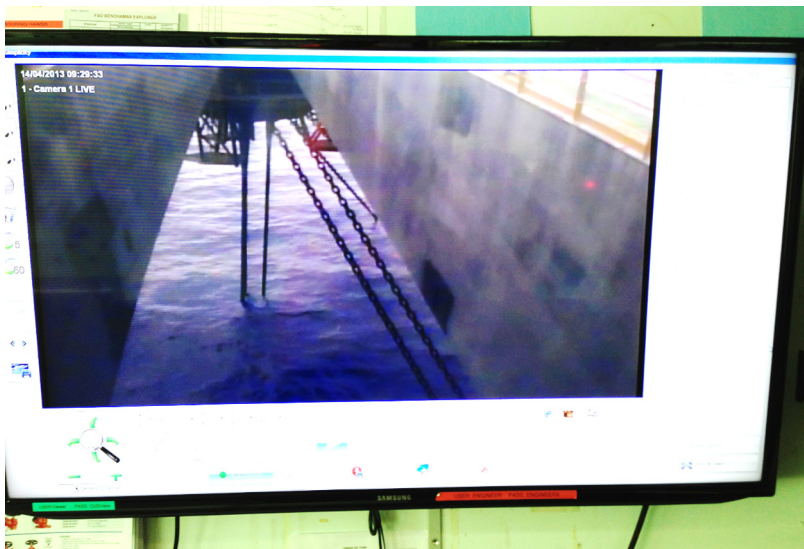
FIGURE 12.9 Monitor screen in the control room of an FPSO showing that risers and mooring lines are intact. FPSO , Floating production storage and offloading.
