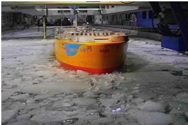
FIGURE 7.4 Ice tank test. Courtesy: SOFEC.
