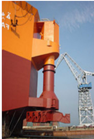
FIGURE 2.8 Submerged external turret system. Courtesy of SBM Offshore.
