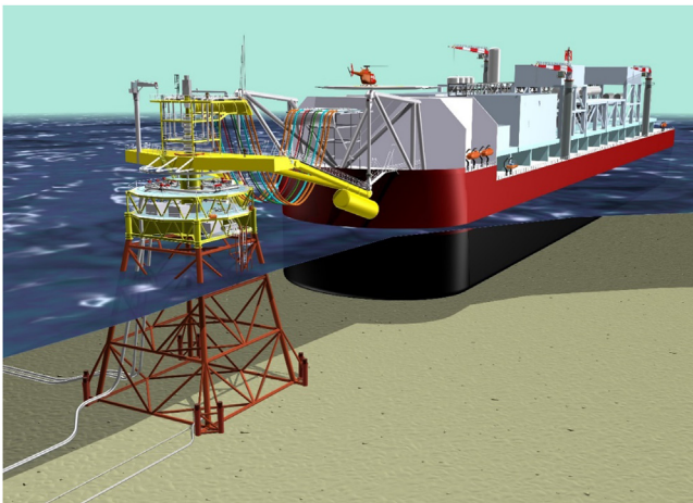
FIGURE 2.13 Tower yoke mooring system. Courtesy of Bluewater.
