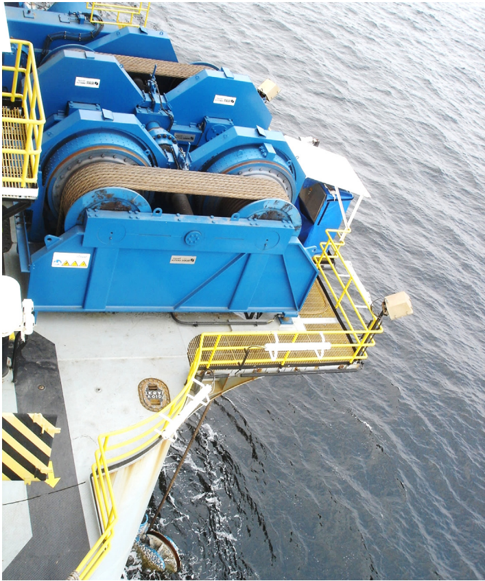
FIGURE 10.9 Two traction winch packages on a semisubmersible rig.
