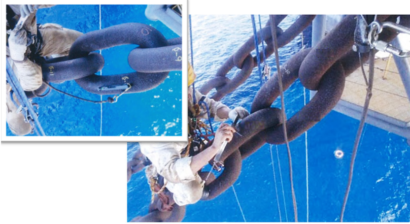
FIGURE 12.5 A rope-access specialist measures chain diameter using a caliper [9].
