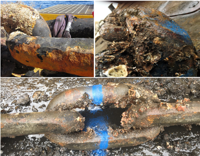
FIGURE 12.7 Ground chain and touch down chain with material loss on one side [9,12].
