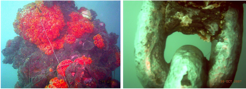
FIGURE 12.3 Marine-fouled chains before and after cleaning by a diver [7,8].
