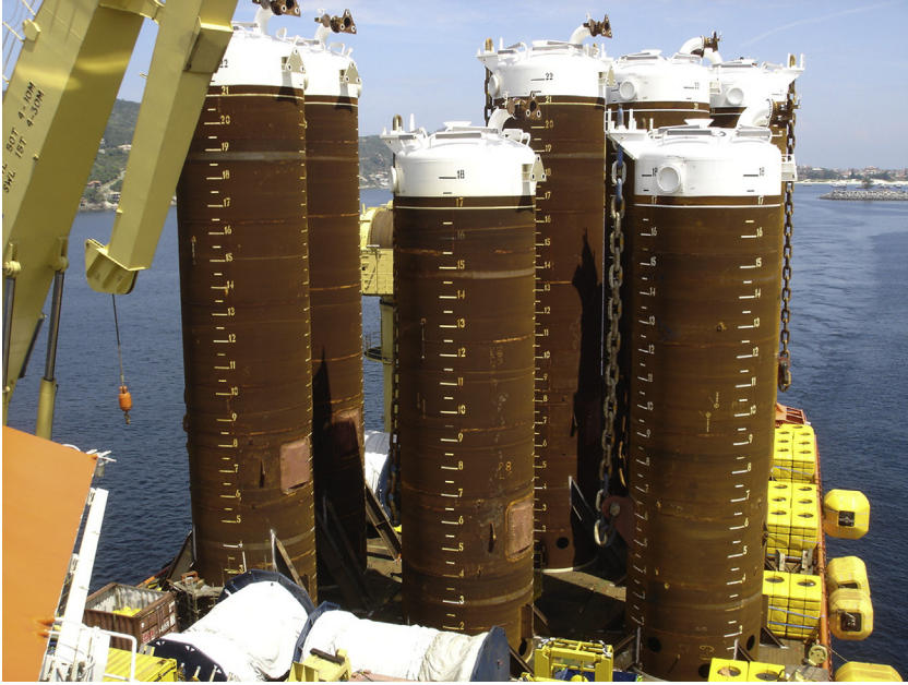
FIGURE 11.15 Large deck space on an AHV allows more mooring components to be carried. AHV, Anchor handling vessel.
