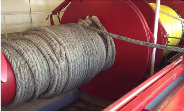
FIGURE 14.2 Unsheathed wire rope getting replaced by brand-new sheathed wire rope during a life extension campaign [10].
