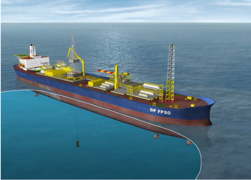
FIGURE 2.15 Dynamic Positioning System for an FPSO, with thrusters attached to the hull. Courtesy of SBM Offshore.
