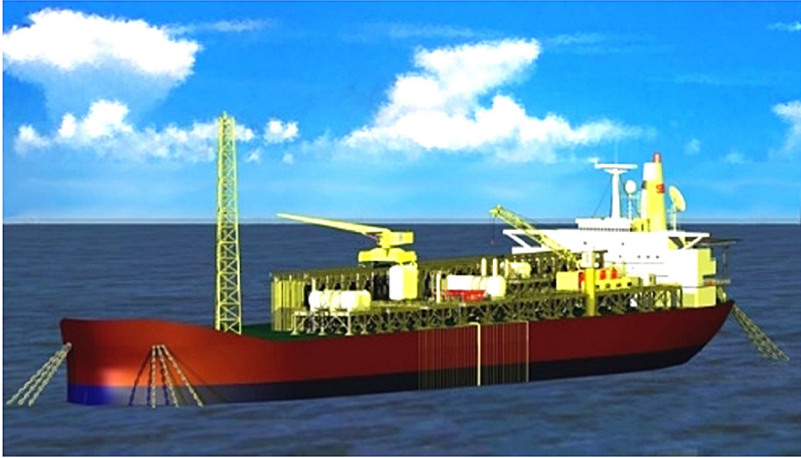
FIGURE 2.3 Clustered-spread mooring in 4 \times 3 (4 clusters with 3 lines in each cluster) pattern for an floating production storage and offloading. Courtesy of SBM Offshore.
