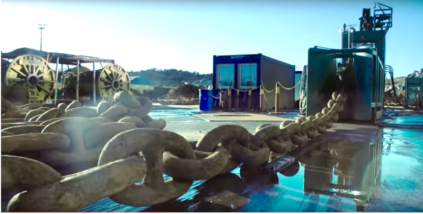
FIGURE 12.1 Dockside inspection method for MODU chain. MODU , Mobile Offshore Drilling Unit. Courtesy: Vryhof.
