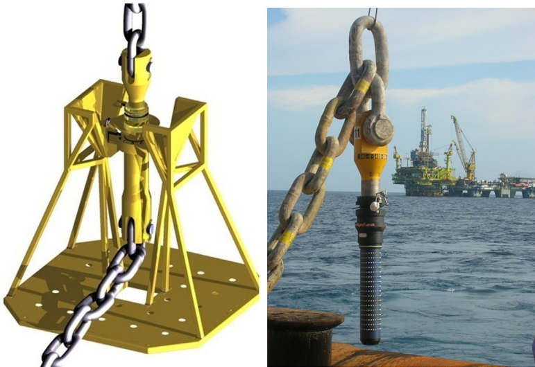
FIGURE 9.12 Subsea connector on a temporary mud mat (left); male part ready to be deployed (right). Courtesy: First Subsea.
