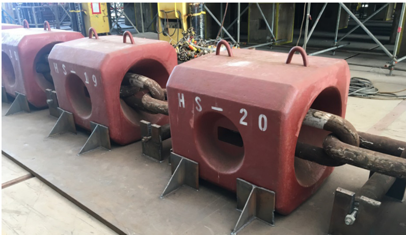
FIGURE 9.15 Clump weights of a mono-cast (single-shell) design fitted on chain.
