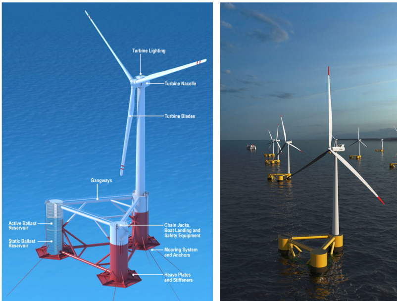
FIGURE 15.3 Semisubmersible-based wind turbine floaters. Courtesy of Principle Power.
