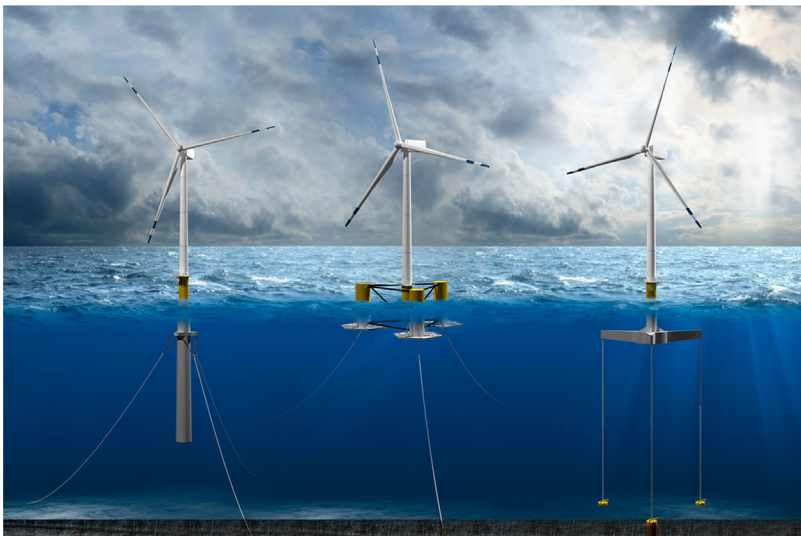
FIGURE 1.9 Floating wind turbines stationed by mooring systems. From Left to Right: Spar, Semi-submersible, and TLP. Illustration by Josh Bauer, National Renewable Energy Laboratory.
