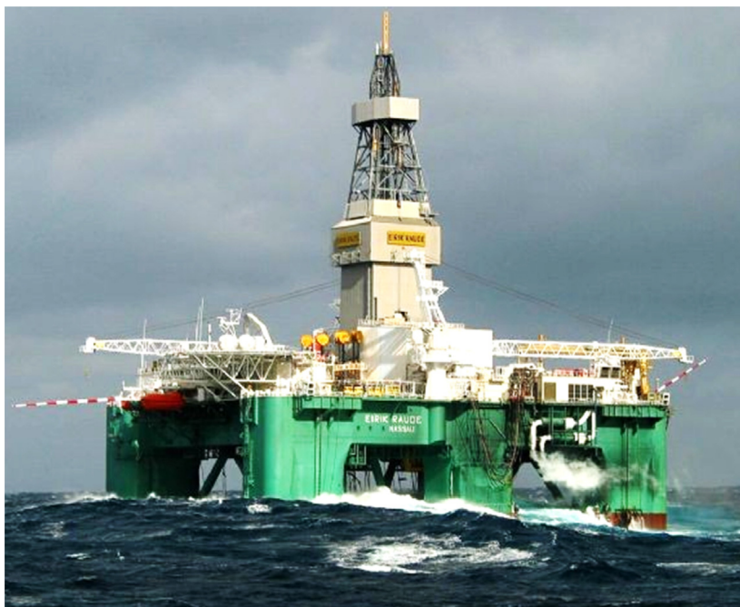
FIGURE 1.2 Fifth-generation drilling semisubmersible designed for deepwater exploration. Courtesy of Transocean.
