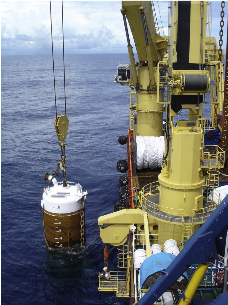
FIGURE 11.1 Suction pile anchor is lowered into the water by the crane of the AHV. AHV, Anchor handling vessel.
