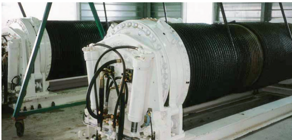
Fig 10.4.1.A Compact design of a high torque motor and winch (Courtesy of Hägglungs Drives)
