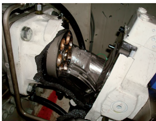
Fig 12.6.2.B Exploded hydraulic motor due to cavitation and the original section view of a new motor
