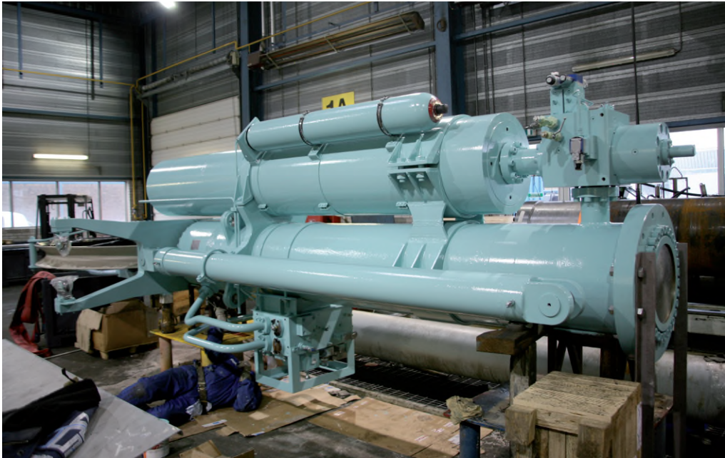
Fig 9.7.1.C Assembly of the main cylinder, two small active cylinders (one is shown at the front) and the medium separator on top, connected via a main manifold with cartridge valve (Courtesy of Huisman)
