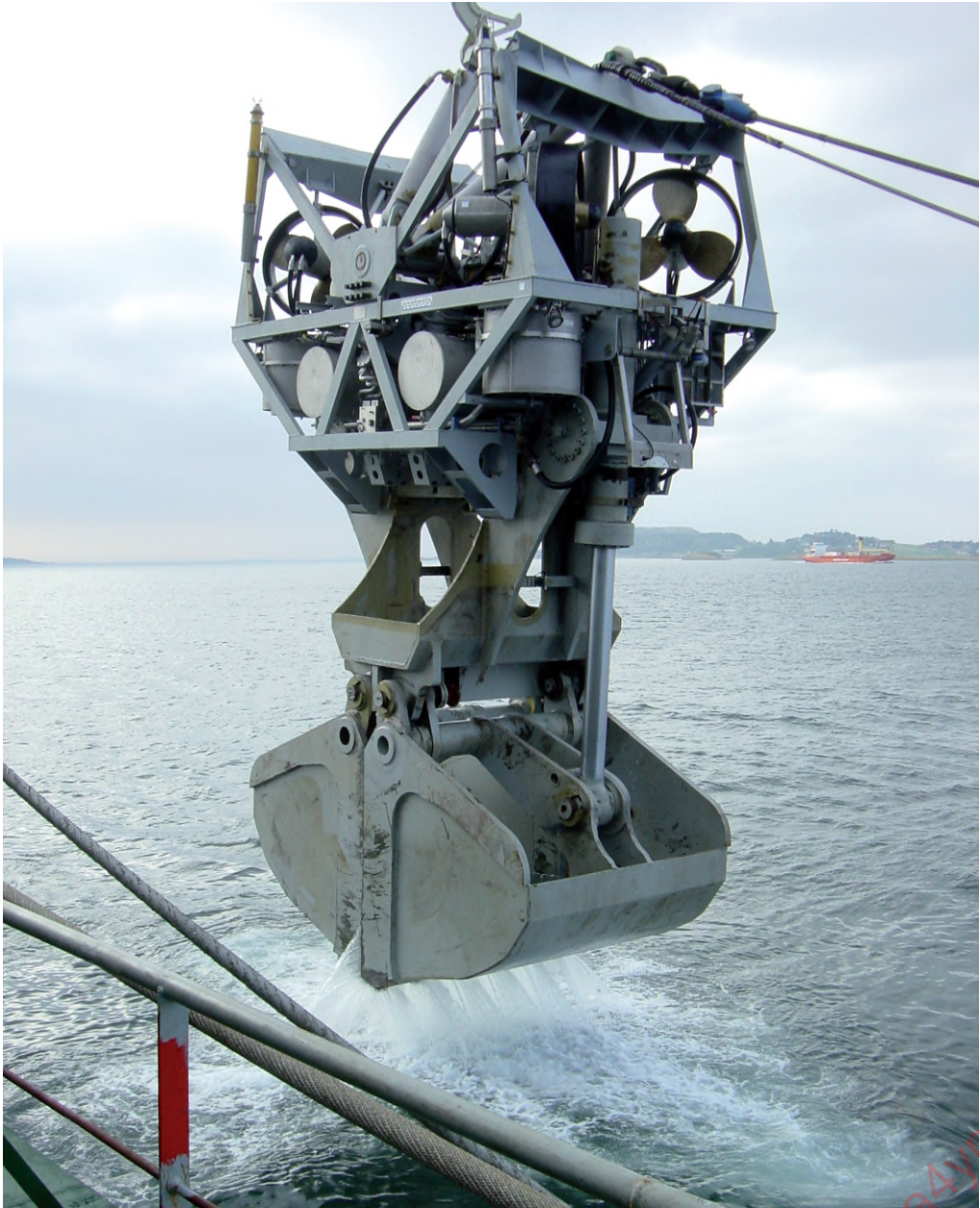
Fig 11.5.A The hydraulic driven grab during sea trials in 2001 (Courtesy of Seatools)
