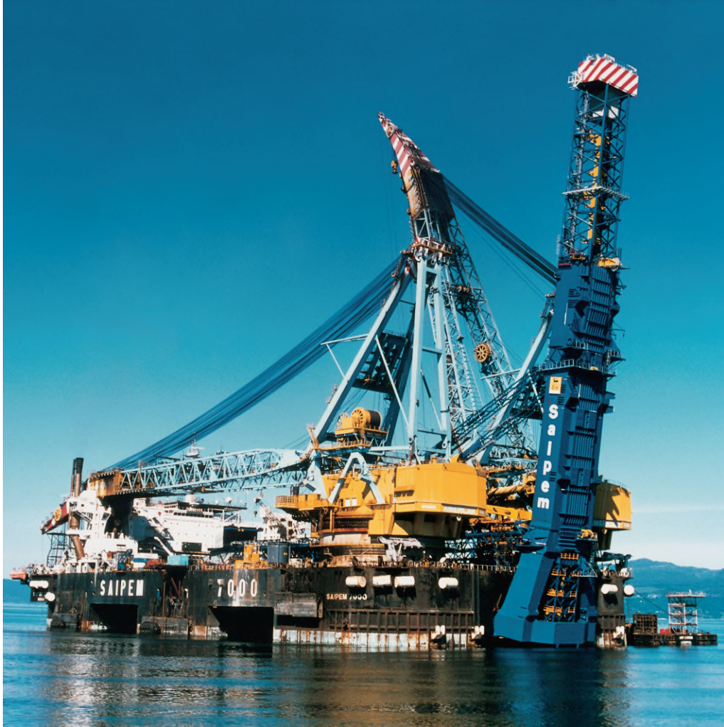
Fig 7.4.A J-Lay tower with adjuster system for the Saipem S7000 (Courtesy of Huisman)
