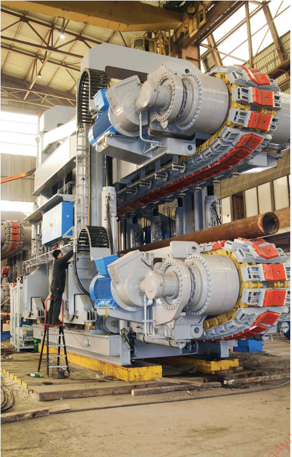
Fig 5 Two-Track tensioner for 350 mTon, each track is driven by an AC induction motor and frequency drive (Courtesy SAS)
