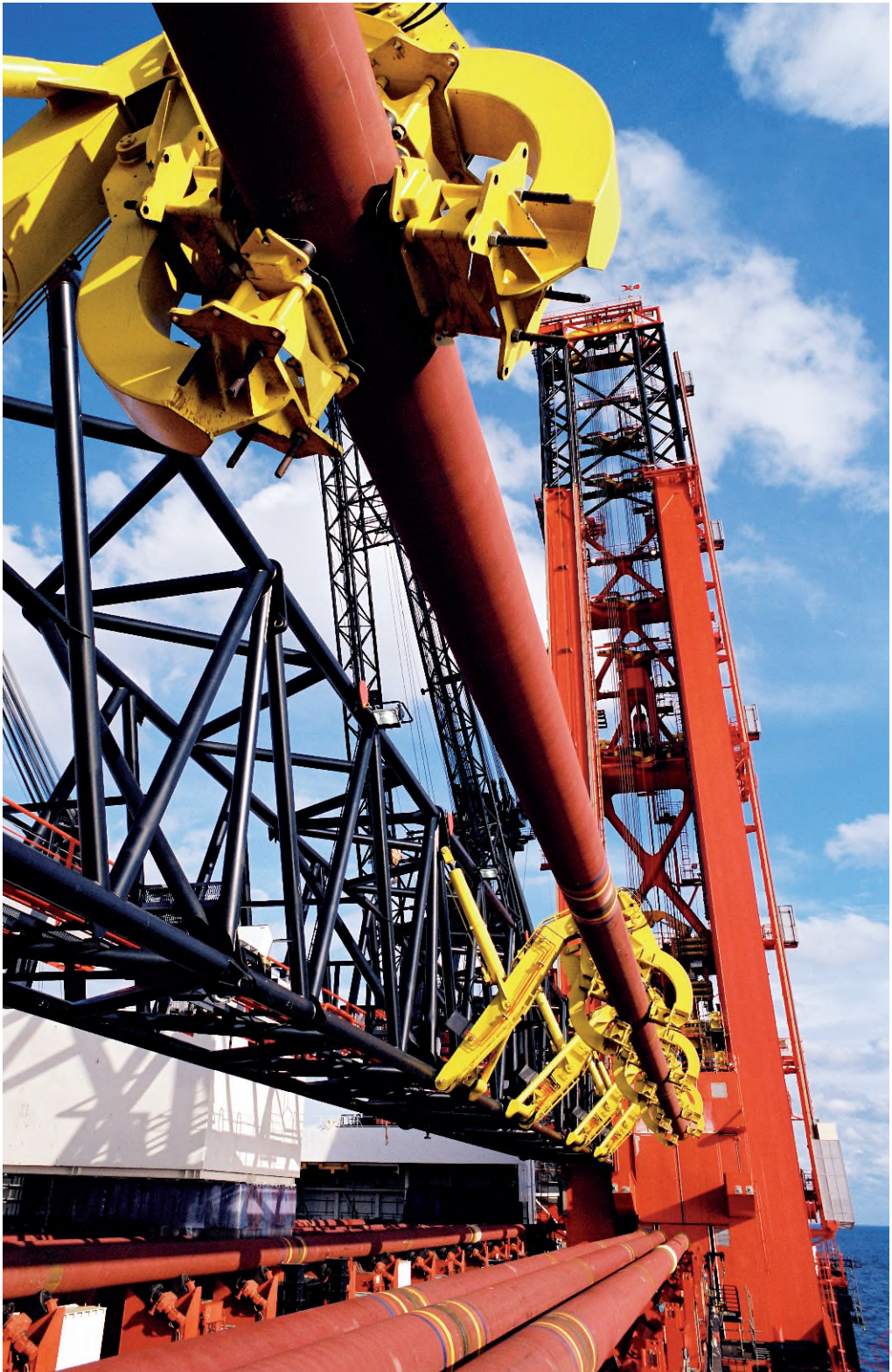
Fig 8.2.B Photo of the loader system (in black) with the loader arms (in yellow), where a new 48 meter long new pipe has just been lifted from the deck (Courtesy of Huisman)
