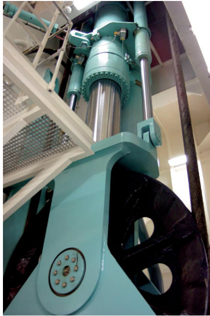
Fig 9.7.2 The active Heave Compensator in operation (Courtesy of Huisman)
