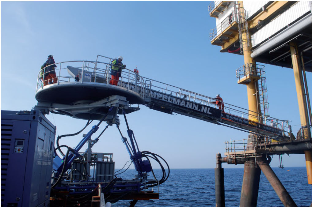
Fig 8.4.1 The active controlled platform Ampelmann in offshore operation (Courtesy of Ampelmann)
