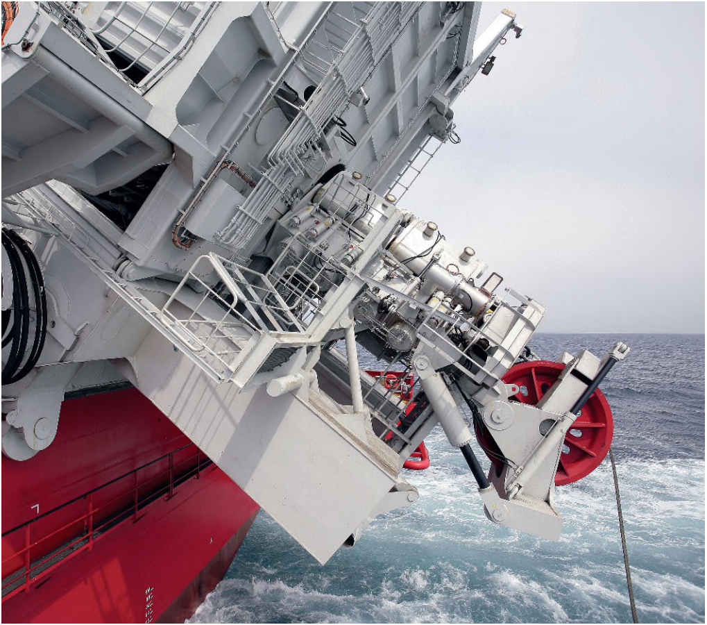
Fig 1.6.7.E Typical application of a cylinder with ceramic layer for the Abandonment and Recovery sheave on the Subsea7 Seven Oceans (Courtesy of IHC Vreemac)
