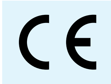
Fig 12.1.A CE mark for equipment that complies with the applicable Directive in the EEC
