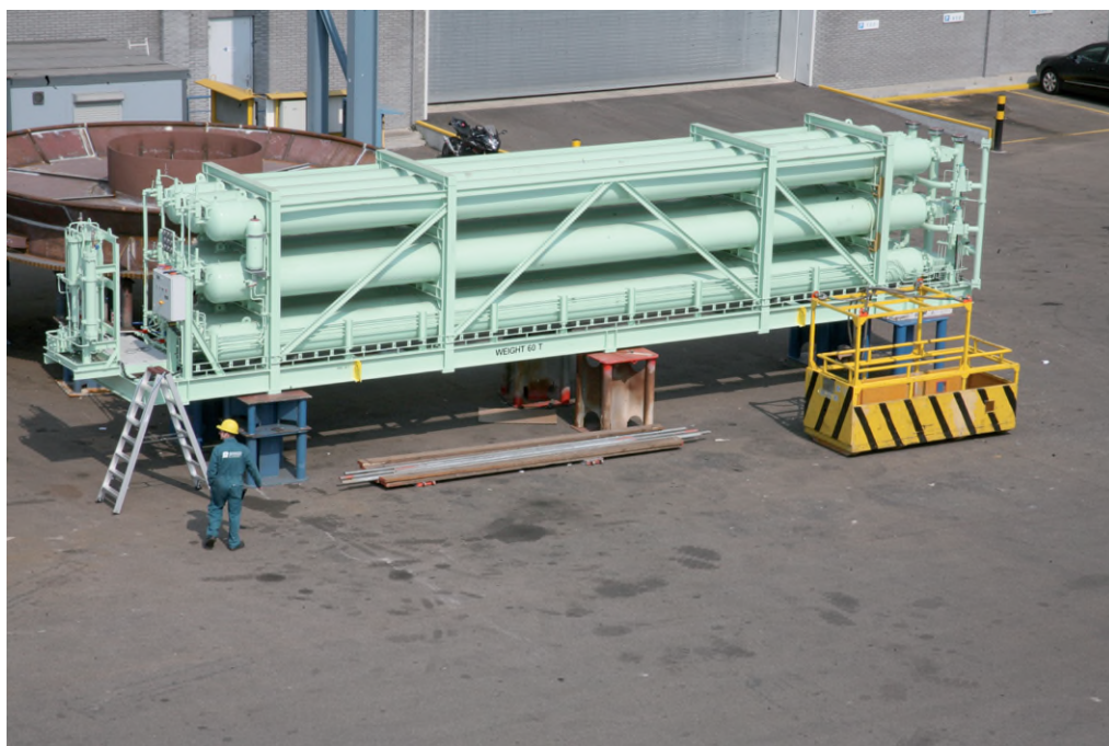
Fig 9.2.C A set of gas bottles, total volume 21600 dm 3 , with design pressure of 300 bar for a riser tensioner system (Courtesy of Huisman)
