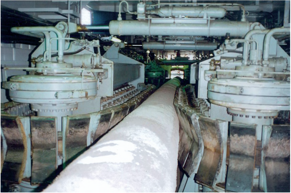
Fig 7.5.C A hydraulic driven pipe tensioner, with the two squeeze cylinders on top, note the small accumulator alongside the cylinders (Courtesy of SAS)
