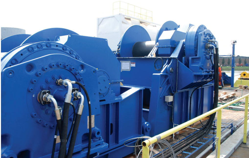
Fig 1.7 Application of a hydraulic driven winch. Here hydraulic motors have been used that can provide the high torque of the winch without the use of an intermediate gearbox..(Courtesy of Högglunds)
