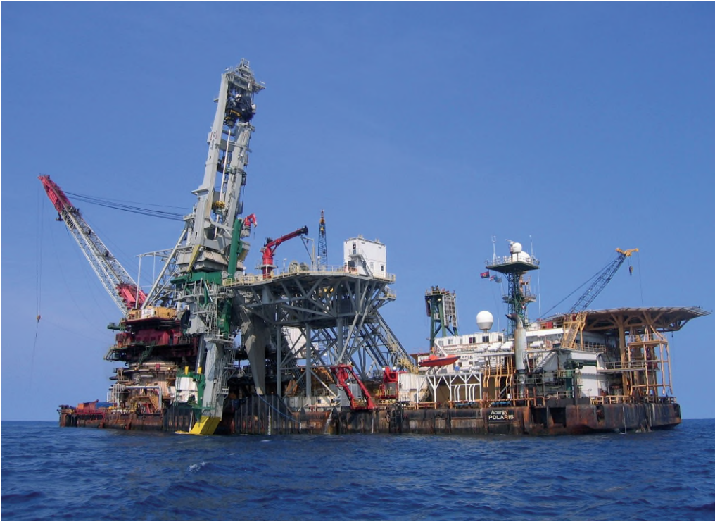
Fig 8.3.2 The J-lay tower with active roll and pitch control in operation on the Polaris of Stolt Offshore (Courtesy of Huisman)
