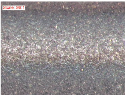
Fig 1.6.7.D Structure of a rod surface with ceramic treatment (Courtesy of Parker Hannifin, Symposium Delft /Holland 2004)
