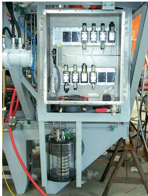
Fig 11.2.D Valve box with servovalves for subsea application. The box is covered with Plexiglas to enable easy inspection when the ROV is above water. Normally the box is internally filled with hydraulic fluid. (Courtesy of Seatools)
