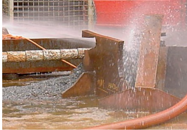
Fig 11.4.F Test of the hydraulic drives saw mechanism in Kirkenes, Norway, water is required to cool the saw. Under water sufficient cooling would be available of course.
