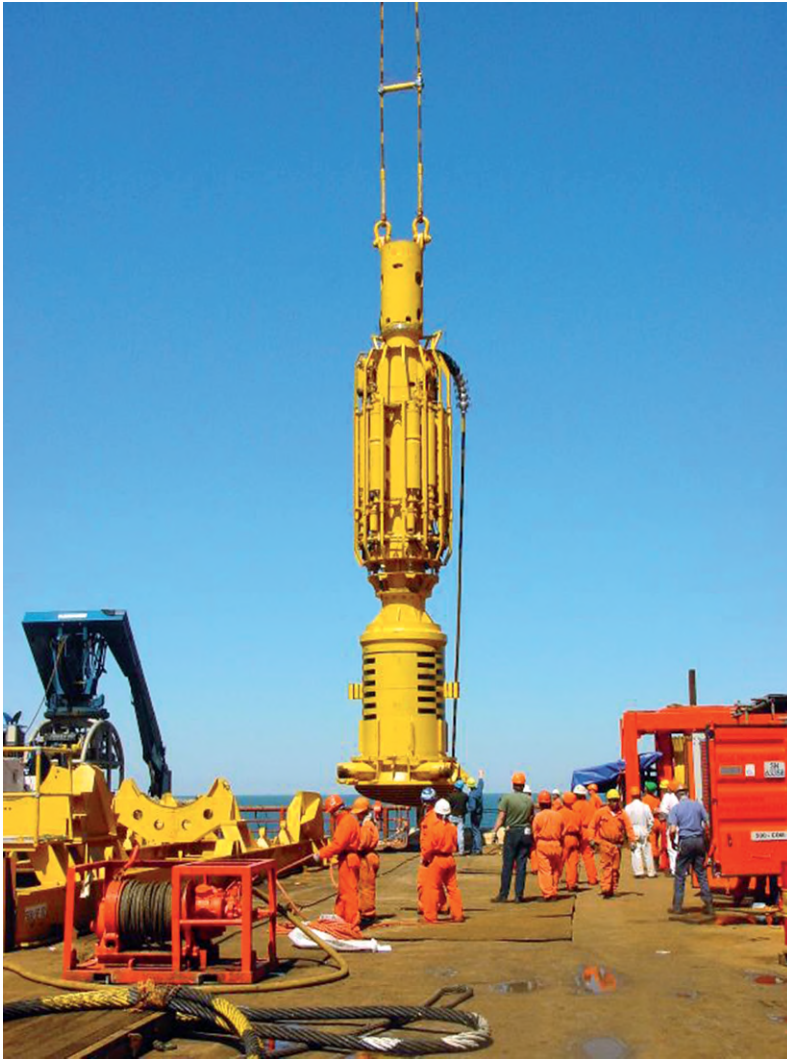
Fig 11.3.B Heerema's largest hammer from Menck with a hydraulic power unit built onto and around the hammer. The electrical power and control of the hammer is run via an umbilical. (courtesy of Heerema)
