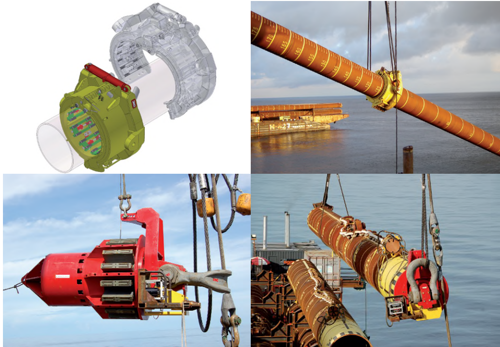
Fig 11.6.A Left above: Principle of an external lifting tool ELT, Right above: An ELT in use to handle the pile, Left below: Clamping can also be provided internally with the ILT, Right below: The ILT in use with an accupack for hydraulic power supply. (Courtesy of IHC)
