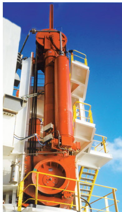
Fig 9.4.B Wire line tensioner (Courtesy of Bosch Rexroth)
