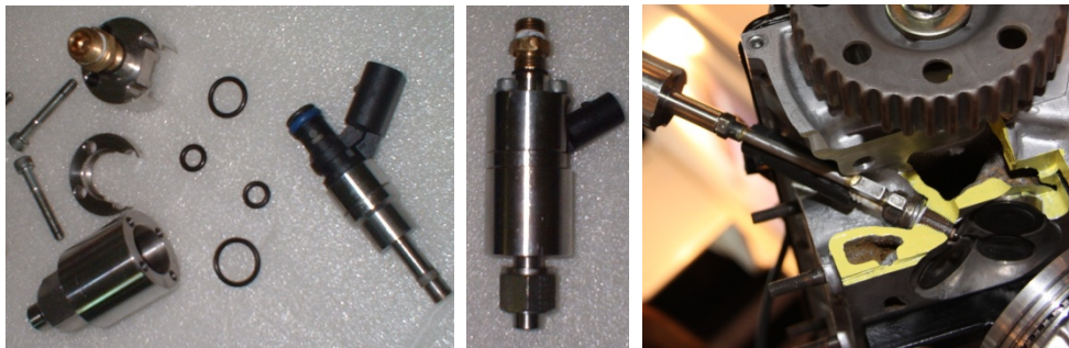
Fig. 3. DGI injector and enclosure component (left), DGI injector in the enclosure (center) and SPFI mounted on an engine (left)
