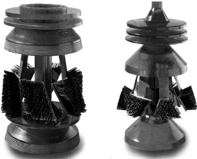
Figure 12–18 Some mandrel pigs used in pipeline pigging operations (Courtesy of T. D. Williamson, Inc.).
