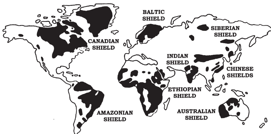
Fig. 2-9. Map of the world showing the location of shields in black where unproductive rocks for gas and oil occur on or near the surface
