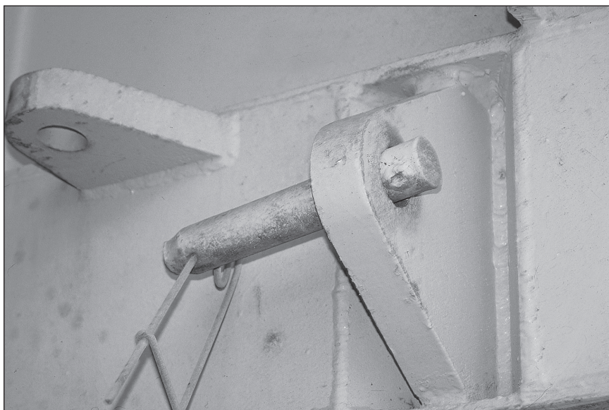
Plate 14-1. Pin with cotter pin used to secure drilling rig modules
