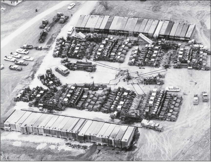
Plate 24–2. Aerial photograph of a massive frac job. The well is in the center with lines of pumping units and frac fluid trailers on either side. (Courtesy of Halliburton.)
