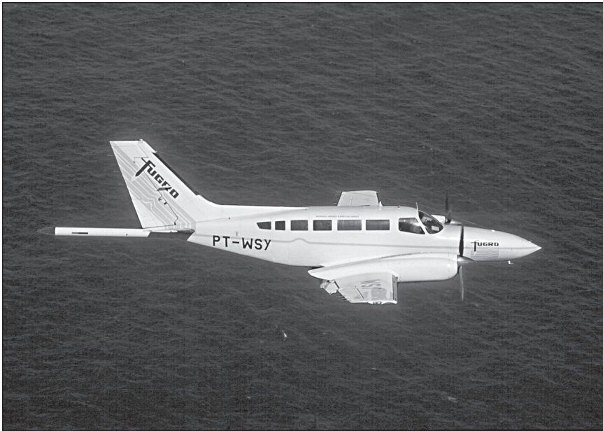
Plate 13–1. Aeromagnetics—the magnetometer is in the stinger behind the airplane. (Courtesy of Fugro.)
