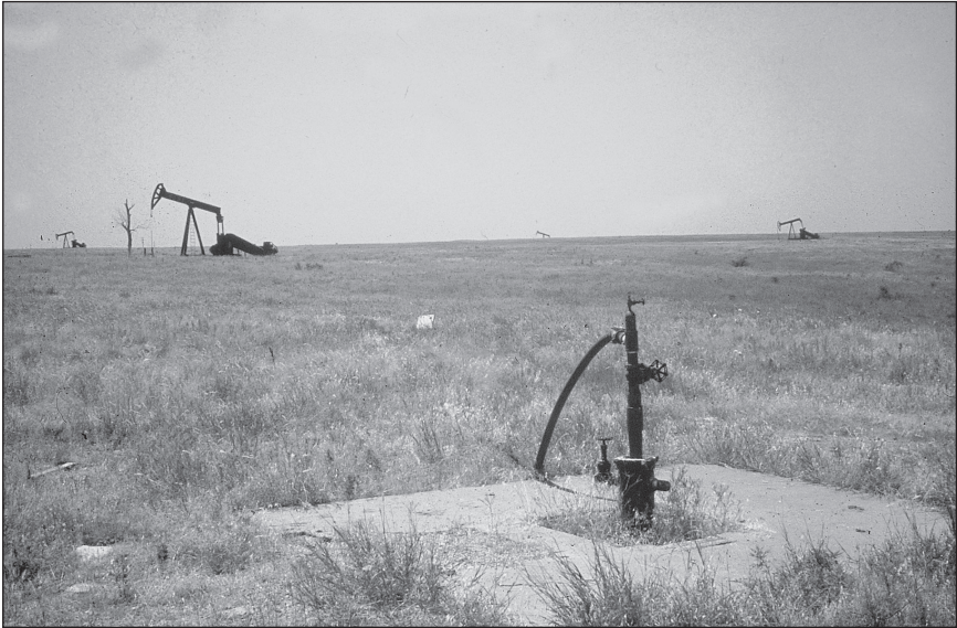
Plate 26-1. Water injection well, Burbank oil field waterflood, Oklahoma
