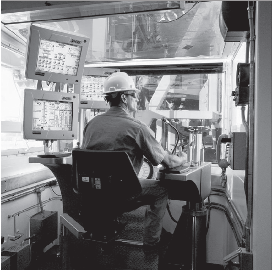
Plate 15–10. A driller's cabin overlooking the drill floor on a modern drilling rig. (Courtesy of Helmerich & Payne.)
