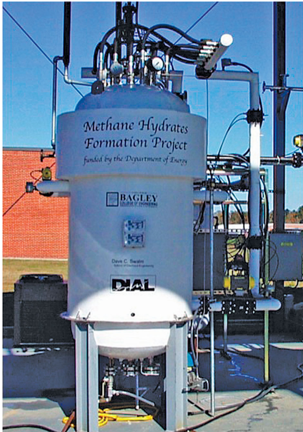
Figure 4.9 Photograph of hydrate formation vessel POC; chiller background left. Combustor, surge tank, bank of source gas not shown. (Courtesy MSU Hydrate Laboratory.)
