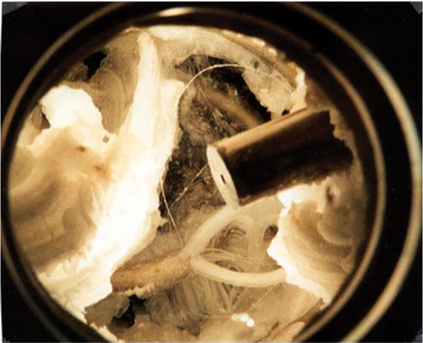
Figure 4.5 Nonsymmetrical slow growth of hydrates without SDS surfactant; after 5–10 days, chilled, under gas pressure. Hydrates above interfacial film barrier. (Courtesy MSU Hydrate Laboratory; Zhong and Rogers, 2000. )
