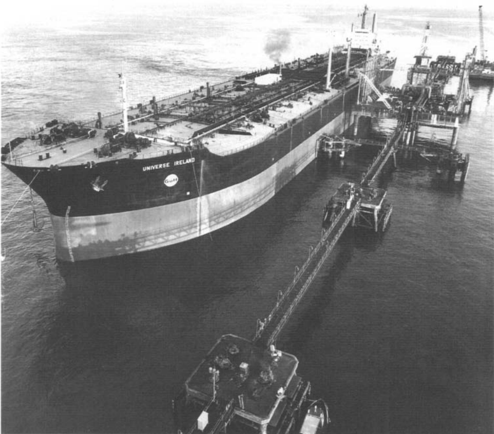
The 312,000 dwt Universe Ireland berthed at the Kuwait Oil Co.’s newly built sea island terminal. The tanker was on its maiden voyage in September 1968 loading crude to take to Bantry Bay, Ireland
