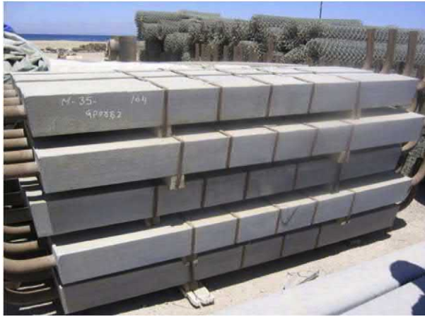
FIGURE 6.9 Cow horn anode weighing 189 kg.
