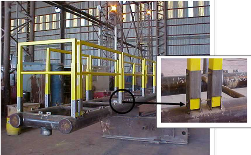
FIGURE 7.45 Handrail made from glass fiber-reinforced polymer (GFRP).
