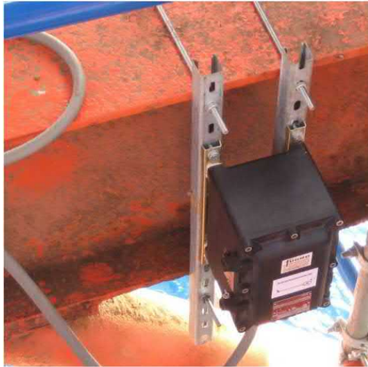
Figure 7.43 Vibration monitoring attached to the deck beam.
