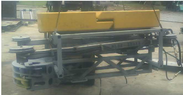
Figure 7.34 Notch the conductor machine.
