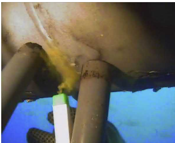
Figure 8.10 Close visual inspection (CVI) by the magnetic particle test (MPI) technique.
