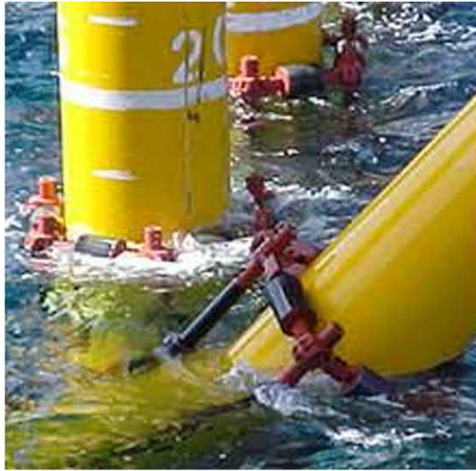
Figure 7.41 Marine growth remover fixation.
