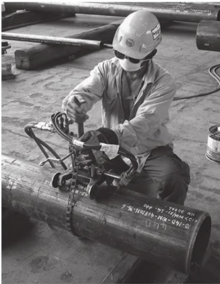
Piping Pre-fabrication: Gas cutting, welding
