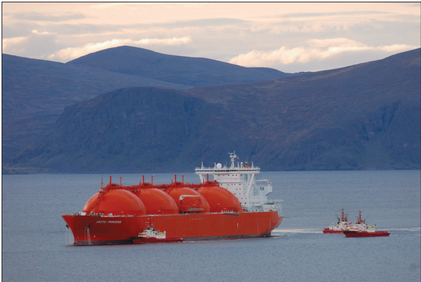
Fig. 10–6. Statoil’s Arctic Princess , an LNG tanker with Moss cargo tanks (Source: Statoil)
