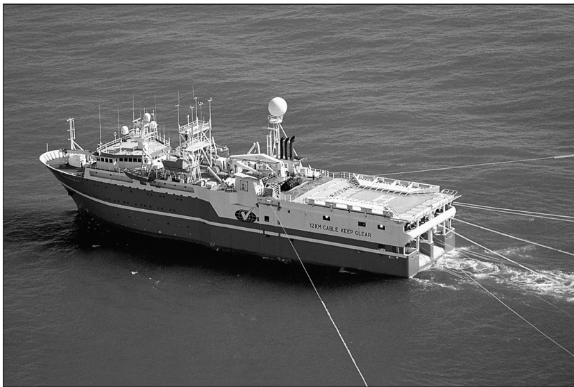
Fig. 4–7. Seismic survey vessel (Source: Leffler, Pattarozzi, and Sterling)
