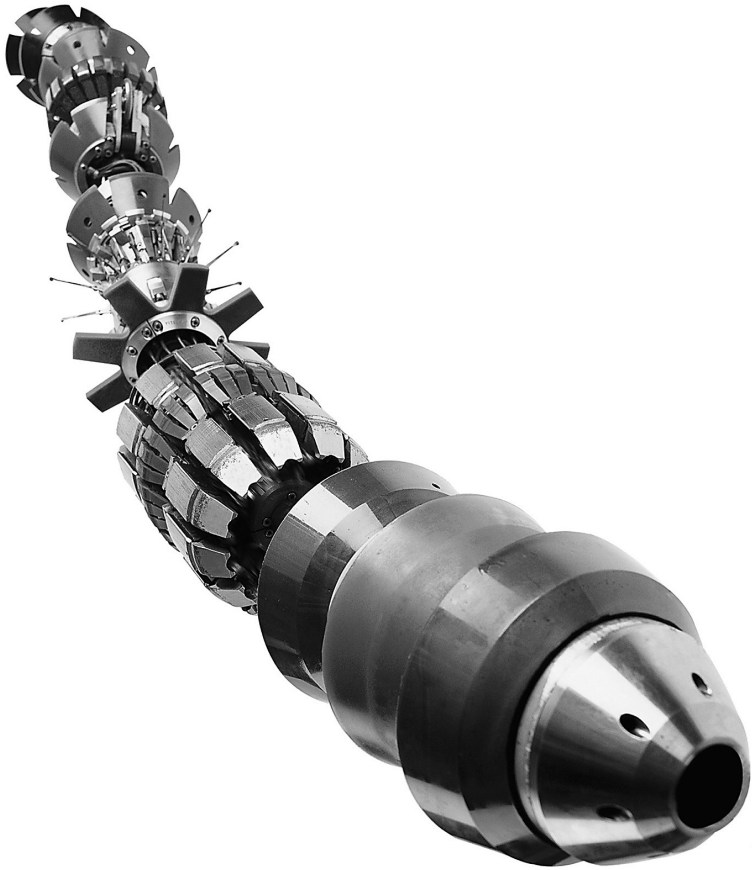
Fig. 8–9. Smart pig for pipeline inspection, capable of detecting both metal loss and mechanical damage ( Source: Miesner and Leffler )
