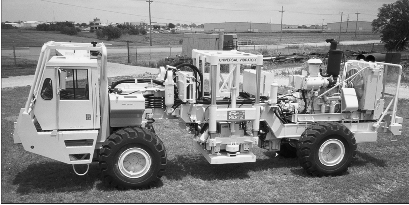
Fig. 4-3. Seismic survey vibrator truck (Source: Hyne, N. J.)
