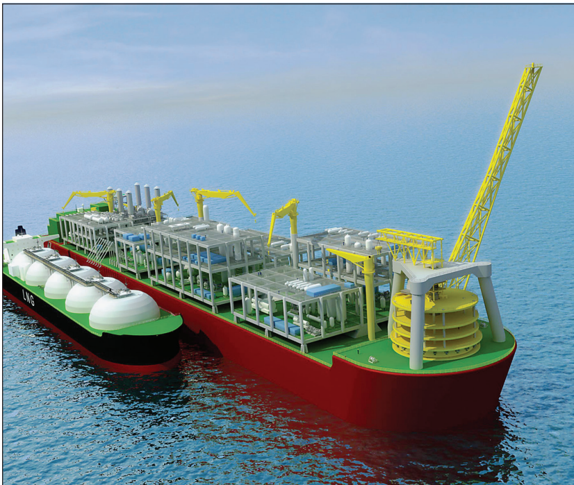
Fig. 10–5. Proposed Shell FPSO (FLNG vessel) for liquefaction offshore Australia (Source: Oil & Gas Journal )
