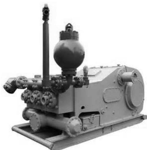
Fig. 1-14 A triplex mud pump with pulsation dampener
