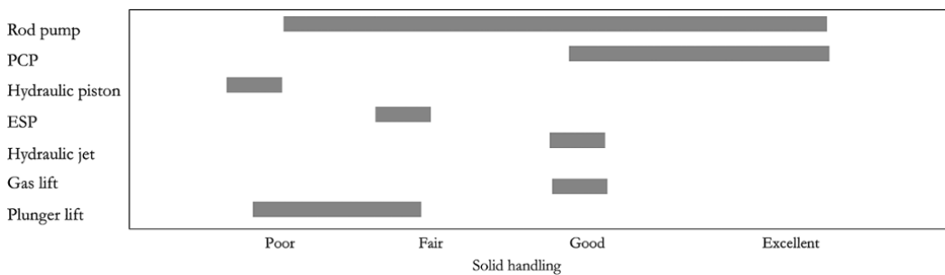
Figure 11.15 Solid handling capability for different artificial lift methods.
