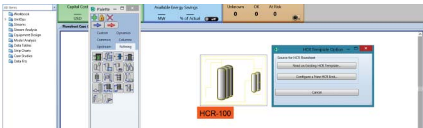
Figure 6.83 Hydrocracker reactor palette – F4 → Refining → Hydrocracker model → Configure a New HCR Unit → HCR configuration wizard.
