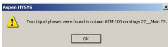
Figure 2.88 Additional warning to indicate that two liquid phases may be present.
