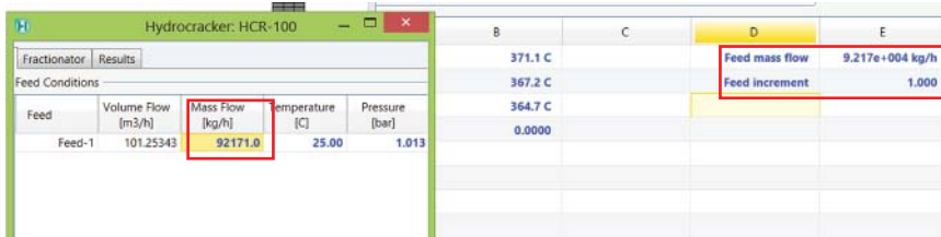
Figure 6.135 Export the feed flow into the spreadsheet.
