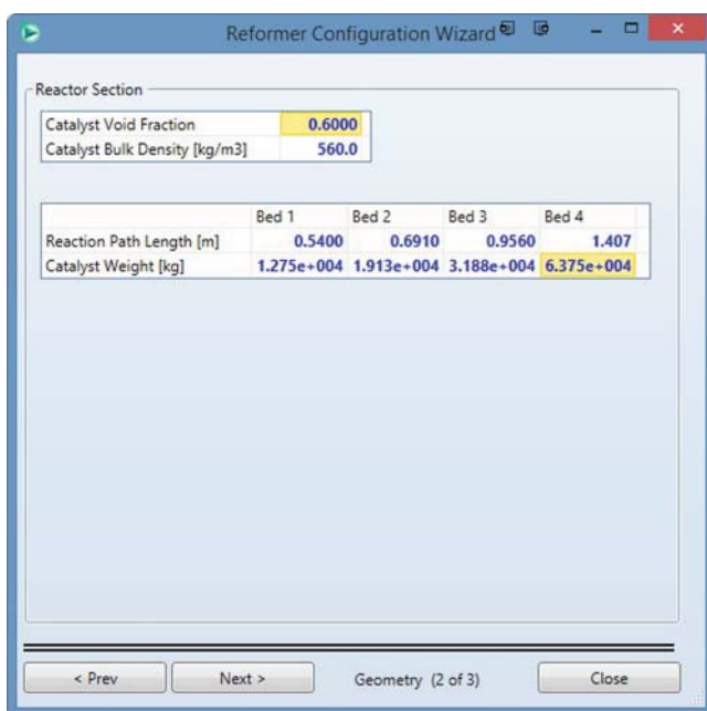
Figure 5.47 Reactor dimensions and catalyst loadings.
