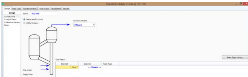
Figure 4.52 Enter the effluent stream, effluent, and delay entering feed stream and feed type to a later step.
