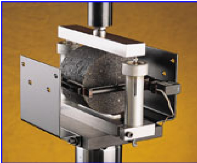
Figure 9.7 Brazilian tension test rig.
