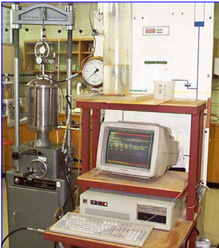
Figure 9.9 Triaxial test arrangement.
