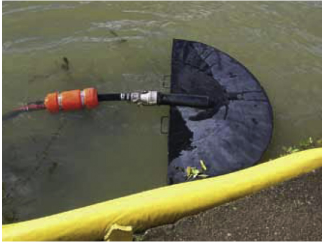
Figure 4.11 Skimmer head of a vacuum/suction skimmer (ITOPF, 2012).
