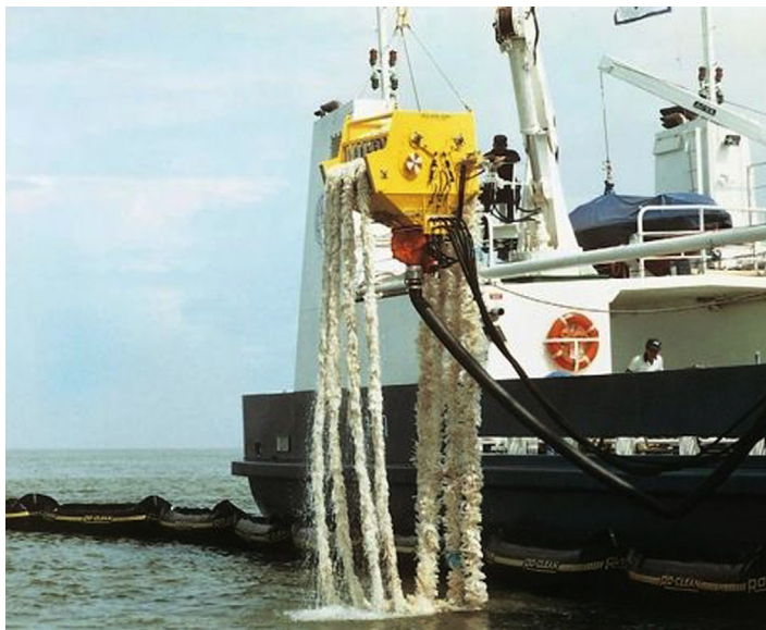
Figure 4.7 Vertical oleophilic rope-mop skimmer. Direct Industry, 2016. Products, Oil Skimmer for Offshore Applications, DESMI Pumping Technology A/S. [online] Available from: http://www.directindustry.com/prod/desmi-pumping-technology-s/product-21088-478363.html .
