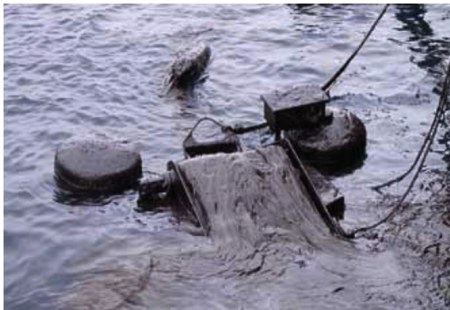
Figure 4.13 Belt adaptor incorporated to increase the capability of weir skimmers in highly emulsified fuel oil (ITOPF, 2012).
