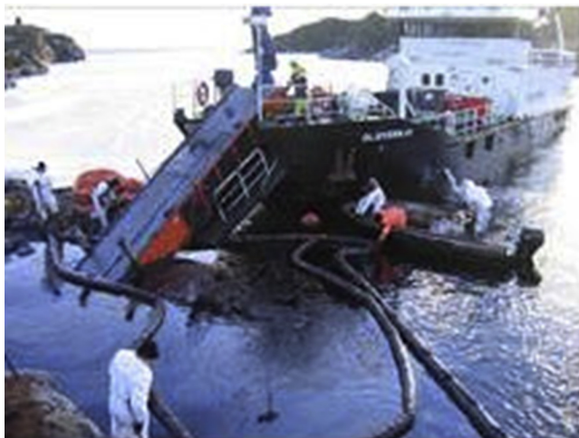
Figure 4.9 Belt skimmer. International Tanker Owners Pollution Federation (ITOPF) Limited. Belt Skimmer in Operation. [online] Available from: http://www.itopf.com/fileadmin/data/Documents/Image_Library/Belt_skimmer.jpg .
