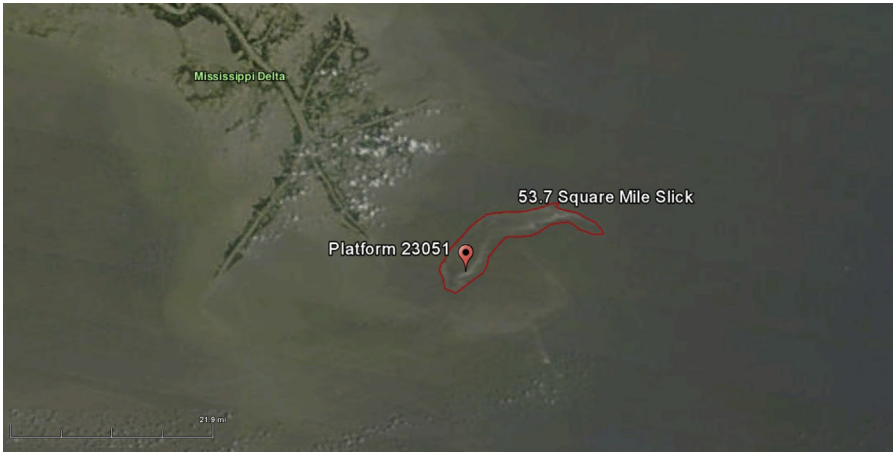
Figure 2.6 A suspected oil slick from site 23,051 in the Gulf of Mexico measuring 18 miles long and covering a surface area of 53.7 square miles.
