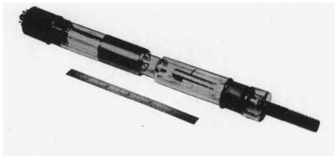
Figure A.38 Down-hole sealed particle accelerator tube (after Tittman and Nelligan, 1959).
