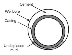
The degree of casing eccentricity in the wellbore is usually described by the *standoff*. Standoff is defined as follows:
