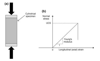
Fig. 2.3 Schematic illustration of a uniaxial compressive test (a) and stress-strain *curve* obtained in a such test (b). UCS is unconfined compressive strength
