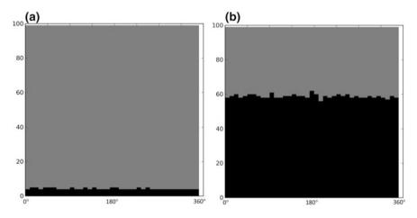
**Fig. 3.22** Fluid distribution in the annulus in simulation 5 (Table 3.2) after pumping 150 L (a) and 2250 L (b) of spacer. Flow rate 15 L/s. A 100-m interval is simulated. The annulus is shown unwrapped. Mud (fluid in place) is shown in *grey*. Spacer (injected fluid) is shown in *black*. The flow direction is upwards
