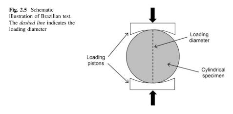
loading diameter is produced along a significant part of that diameter. The tensile stress is largest near the cylinder's axis and tends to split the cylinder into two halves. Compressive load is increased during the test up until the specimen breaks down. The maximum load,  $F_m$ , recorded during the test is then used to obtain the tensile strength of the material,  $T_0$  [12]:
