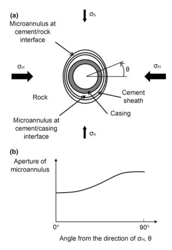
Fig. 5.8 Effect of in situ stress anisotropy on the aperture of microannuli around a vertical well.  $\sigma_H$  and  $\sigma_h$  are the maximum and minimum *horizontal* in situ stresses, respectively. Based on the simulation results by Gray et al. [14]
