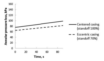
**Fig. 3.13** Annular pressure loss over a 100-m interval versus time in simulation C (Table 3.1, standoff 70 %) and a simulation with the same fluid properties and flow rate but a standoff of 100 % (centered casing)
