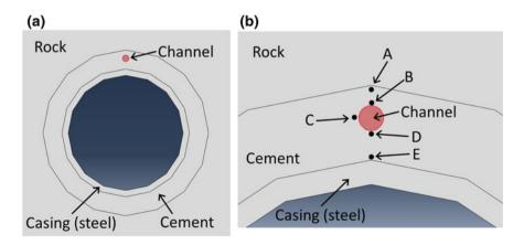
Fig. 5.7 Geometry of a cased and cemented well with a void channel left in cement
