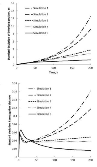
**Fig. 3.24** Standard deviation of mud-spacer interface position along the wellbore axis normalized by the average interface propagation distance versus pumping time. Settings of simulations 1 through 5 are given in Table 3.2
