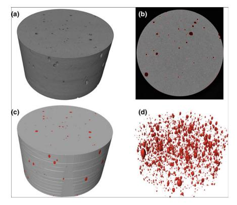
Fig. 4.1 3D cement volume imaged by X-ray micro computed tomography (CT). **a** A 3D visualization of the CT data, **b** cement pores are segmented and marked with *red color* in each of the stacked 2D images, **c** a 3D visualization of the segmented data, **d** a visualization of cement pores only. These type of 3D visualizations can be used to find sample porosity, pore size distributions, pore connectivity and pore morphology
