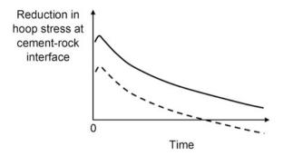
Fig. 6.1 Reduction in compressive hoop stress in cement near cement-rock interface for cements with different Young's modulus. *Solid line* stiffer cement. *Dashed line* softer cement. The Young's modulus of the rock is the same in both cases. Positive values of reduction mean that the hoop stress becomes more tensile
