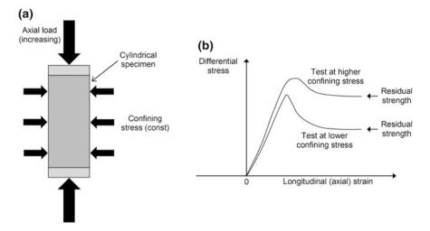
**Fig. 2.4** Schematic illustration of a triaxial compressive test (**a**) and stress-strain curves obtained in such a test (**b**). Differential stress is axial minus confining stress. Higher confining results in more ductile (less brittle) behavior
