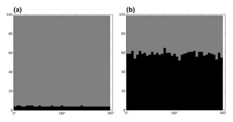
**Fig. 3.20** Fluid distribution in the annulus in simulation 3 (Table 3.2) after pumping 150 L (a) and 2250 L (b) of spacer. Flow rate 15 L/s. A 100-m interval is simulated. The annulus is shown unwrapped. Mud (fluid in place) is shown in *grey*. Spacer (injected fluid) is shown in *black*. The flow direction is upwards
