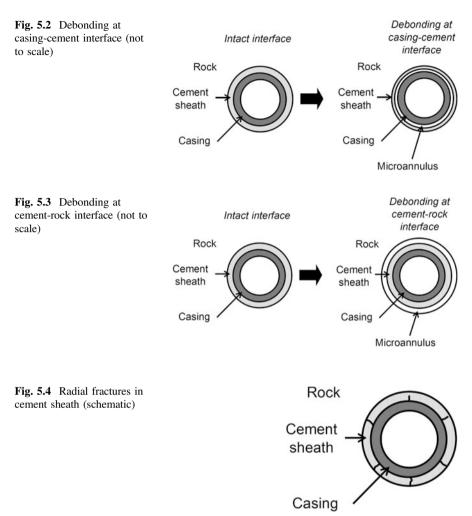
Shear failure of cement may develop if all the principal effective stresses are compressive and such that the shear strength of cement is exceeded. In theoretical analyses of cement failure, the Mohr-Coulomb failure criterion is often used to describe the shear strength, as discussed in Chap. 2. More complex failure criteria are available and have been used for well cement [5].
