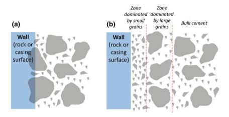
Fig. 4.3 Schematic illustration of the "wall effect", where the wall can be either the steel casing or the drilled rock surface in wells, based on [6]. a Representation of unphysical packing, since the wall cannot cut through cement grains. b Cement grains will have to pack in a different way close to the wall, giving rise to the ITZ
