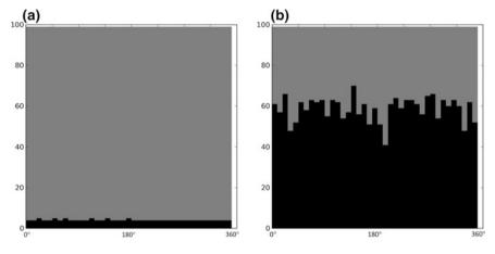
**Fig. 3.18** Fluid distribution in the annulus in simulation 1 (Table 3.2) after pumping 150 L (a) and 2250 L (b) of spacer. Flow rate 15 L/s. A 100-m interval is simulated. The annulus is shown unwrapped. Mud (fluid in place) is shown in *grey*. Spacer (injected fluid) is shown in *black*. The flow direction is upwards
