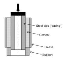
In addition to the bonding strength, *hydraulic bonding* properties of an interface can provide a valuable estimate of the bond quality with respect to possible leakage. Laboratory tests have been designed that quantify hydraulic bonding by applying fluid pressure at the interface in a compound cement-steel or cement-rock specimen [4].
