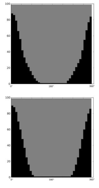
**Fig. 3.9** Fluid distribution in the annulus in simulation D (Table 3.1) after pumping 1275 L of spacer. Mobility ratio 1.87; flow rate 15 L/s. A 100-m interval is simulated. The annulus is shown unwrapped. Mud (fluid in place) is shown in *grey*. Spacer (injected fluid) is shown in *black*. The flow direction is upwards
