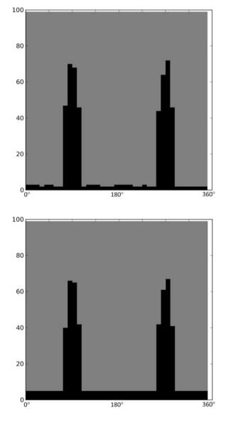
**Fig. 3.31** Fluid distribution in the annulus in simulation B3 (Table 3.3) after pumping 750 L of cement. Mobility ratio 0.87; flow rate 15 L/s. A 100-m interval is simulated. The annulus is shown unwrapped. Mud (fluid in place) is shown in *grey*. Spacer (injected fluid) is shown in *black*. The flow direction is upwards
