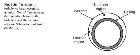
(Fig. 3.36). This will compromise mud displacement from the narrow side of the annulus since the displacing fluid will create a channel on the wider side. Uneven borehole walls and the presence of hardware in the annulus (centralizers, etc.) can complicate the issue of flow regime even further.
