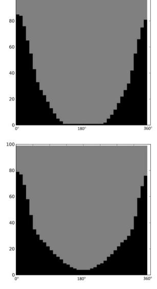
**Fig. 3.11** Fluid distribution in the annulus in simulation F (Table 3.1) after pumping 1275 L of spacer. Mobility ratio 0.47; flow rate 15 L/s. A 100-m interval is simulated. The annulus is shown unwrapped. Mud (fluid in place) is shown in *grey*. Spacer (injected fluid) is shown in *black*. The flow direction is upwards
