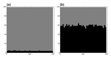
**Fig. 3.21** Fluid distribution in the annulus in simulation 4 (Table 3.2) after pumping 150 L (a) and 2250 L (b) of spacer. Flow rate 15 L/s. A 100-m interval is simulated. The annulus is shown unwrapped. Mud (fluid in place) is shown in *grey*. Spacer (injected fluid) is shown in *black*. The flow direction is upwards
