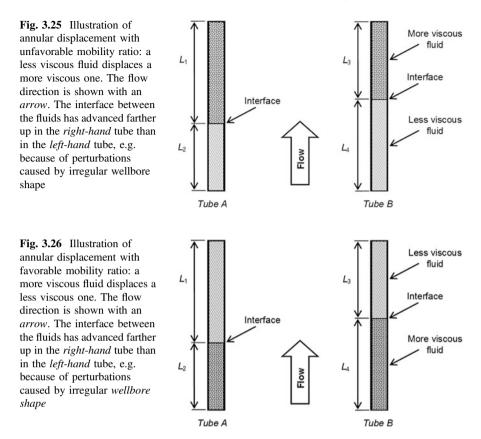
Hence, a small difference in the interface positions in the tubes, once created by e.g. irregular wellbore profile, will be increasing as the flow continues. The annular flow is thus unstable in this case since a small fluctuation in the shape of the mud-spacer interface will increase over time.
