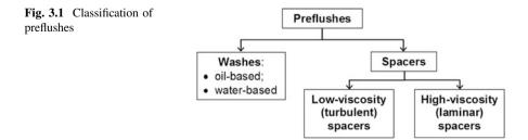
base oil, or a chemical solution. Fresh water can be used, e.g., in a wellbore drilled with water-base mud. Washes may contain dispersants and surfactants for more effective cleaning, in which case they are known as *chemical washes*. Diesel oil or a mixture of water, mutual solvents, and surfactants can be used in a well drilled with a non-aqueous fluid (oil- or synthetic-base mud) [2].
