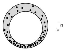
Breakouts are usually more common in deviated and horizontal wells since the in situ-stress anisotropy in the plane normal to the wellbore axis is greater in such wells (at least in an extensional tectonic environment). Breakouts result in cement channeling through breakouts, as we saw in Sect. 3.4. A keyhole-shaped cross-section, created by the drill pipe action, has a detrimental effect on cementing quality, too.
