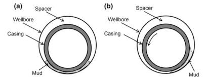
Fig. 3.37 Effect of pipe rotation on mud displacement in the annulus: **a** no rotation; **b** rotation facilitates mud removal from the narrow part of the annulus
