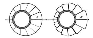
Fig. 3.3 Slice of annulus discretized into sectors (*left-hand panel*) and equivalent sectors replacing the original sectors (*right-hand panel*). The equivalent sector A' has same area and the same inner radius as the original sector, A
