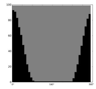
Fig. 3.8 Fluid distribution in the annulus in simulation C (Table 3.1) after pumping 1275 L of spacer. Mobility ratio 0.94; flow rate 15 L/s. A 100-m interval is simulated. The annulus is shown unwrapped. Mud (fluid in place) is shown in *grey*. Spacer (injected fluid) is shown in *black*. The flow direction is upwards
