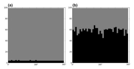
**Fig. 3.19** Fluid distribution in the annulus in simulation 2 (Table 3.2) after pumping 150 L (a) and 2250 L (b) of spacer. Flow rate 15 L/s. A 100-m interval is simulated. The annulus is shown unwrapped. Mud (fluid in place) is shown in *grey*. Spacer (injected fluid) is shown in *black*. The flow direction is upwards
