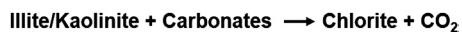
FIGURE 2.31 Mechanism for thermal decomposition of carbonates in argillaceous sandstone and shale. As proposed by Smith, J.T., Ehrenberg, S.N., 1989. Correlation of carbon dioxide abundance with temperature in clastic hydrocarbon reservoirs: relationship to inorganic chemical equilibrium. Marine and Petroleum Geology 6, 129–135.
