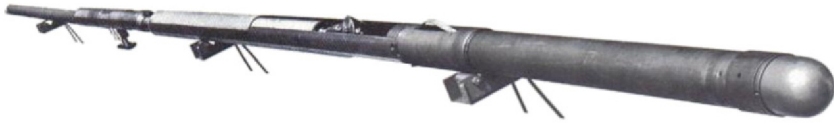
FIGURE 3.1 Schlumberger mechanical coring tool from the 1970s. The two diamond saws that cut a triangular core from the borehole wall can be seen in the middle of the tool.
