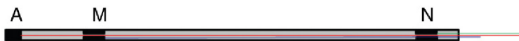
FIGURE 14.6 Schematic of a deep-reading resistivity tool. Current is passed from electrode A to a fourth electrode at or near the surface. The resulting voltage drop is measured between electrodes M and N. The ratio AM/AN varies from 0.1 to 0.5.
