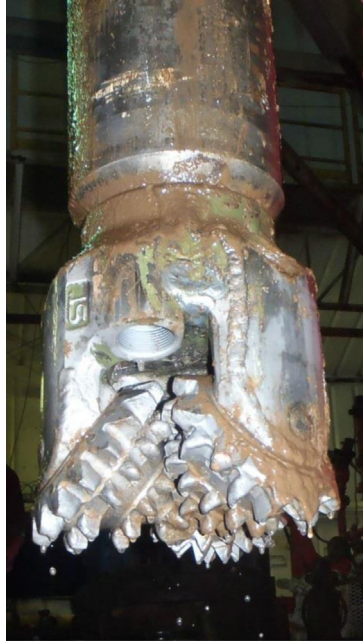
Figure 2.12 Rock bit coming out of hole. Note nozzles have been removed.
