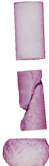
Figure 4.8 Carthage marble tests. Pretest (top), brittle (middle), and malleable (bottom). Courtesy: IADC.
