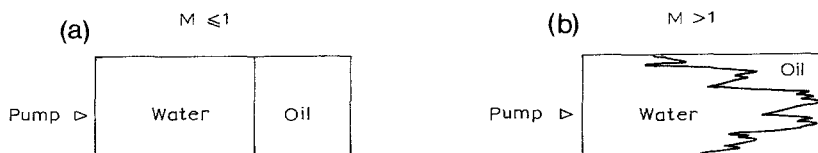
Fig. 5.3. One-dimensional waterdrive experiment in a homogeneous core plug.
