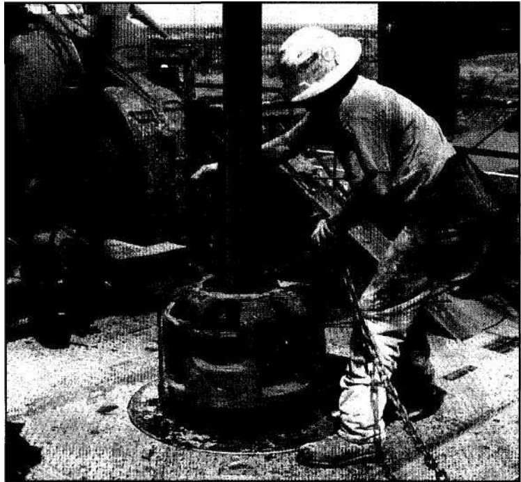
Figure 151. The kelly drive bushing is about to engage the master bushing.
