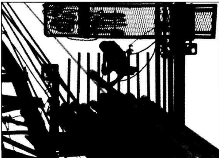
Figure 155. The derrickman has just placed the upper end of a stand of drill pipe between the fingers of the fingerboard.
