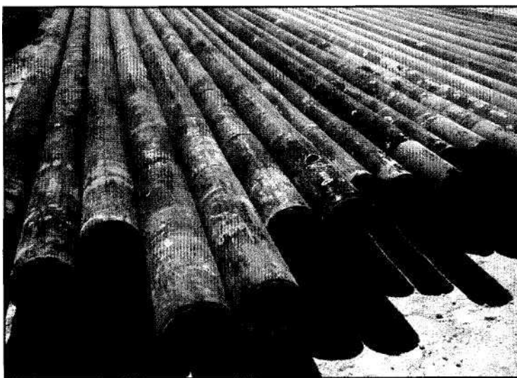
Figure 113. These drill collars are laid out on a rack prior to being run into the well.
