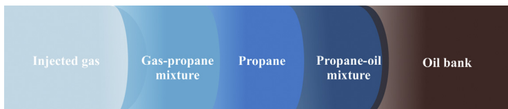
Figure 10.18 Oil displacement scheme for the liquid propane supported flooding.
