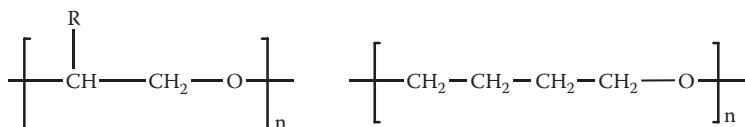
FIGURE 11.2 Structures of polyalkylene oxides (left) and polytetrahydrofuran (right). R = H (EO), R = Me (PO), R = Et (BO).
