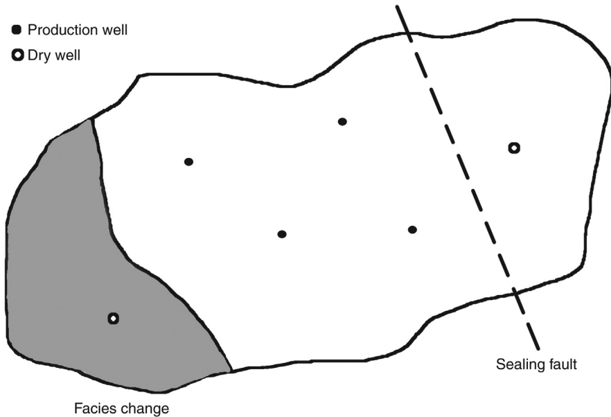
Figure 7.2 Reservoir delineation with fault and facies change as newly drilled wells provide detailed information.
