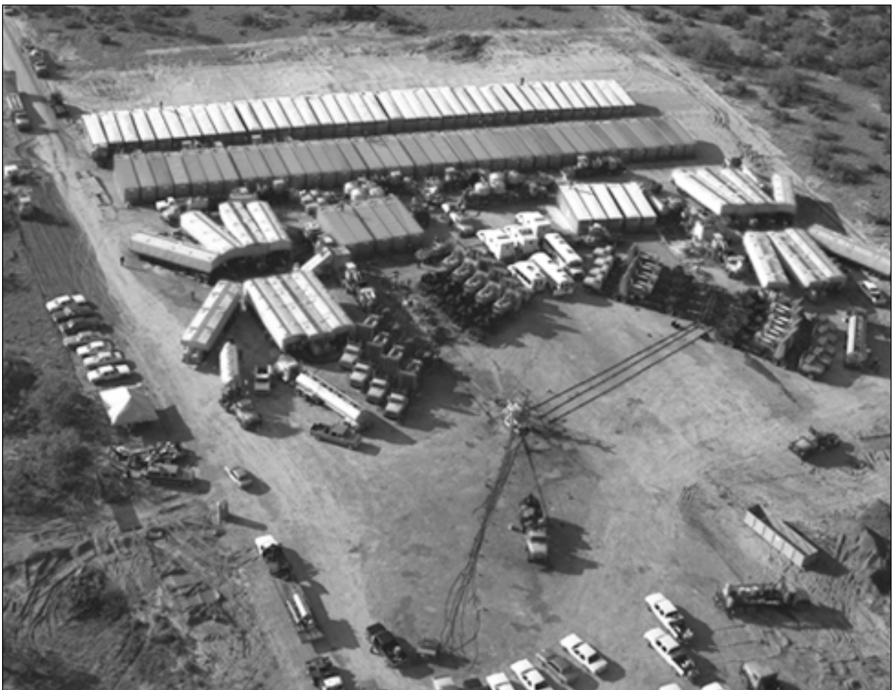
Figure 11-7. Fracturing equipment on a large fracturing treatment.
