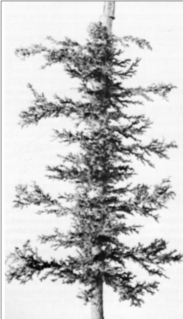
Figure 17-2. Cast of a wormhole pattern in radial geometry (Daccord and Lenormand, 1987).
