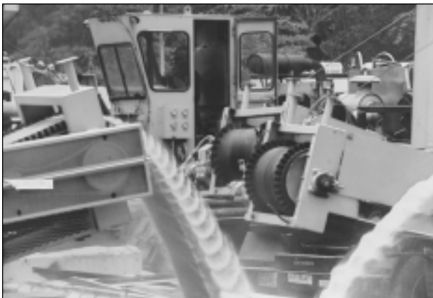
Figure 1-25. For this fracturing treatment, propping agent was introduced into the fracturing fluid via conveyors to the blender. The blender added the propping agent to the continuously mixed fracturing fluid (creating a slurry) and discharged the slurry to the high-pressure pumping equipment.
