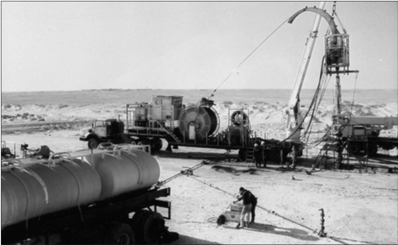
Figure 1-22. Matrix stimulation treatment using a coiled tubing unit, pump truck and fluid transport.
