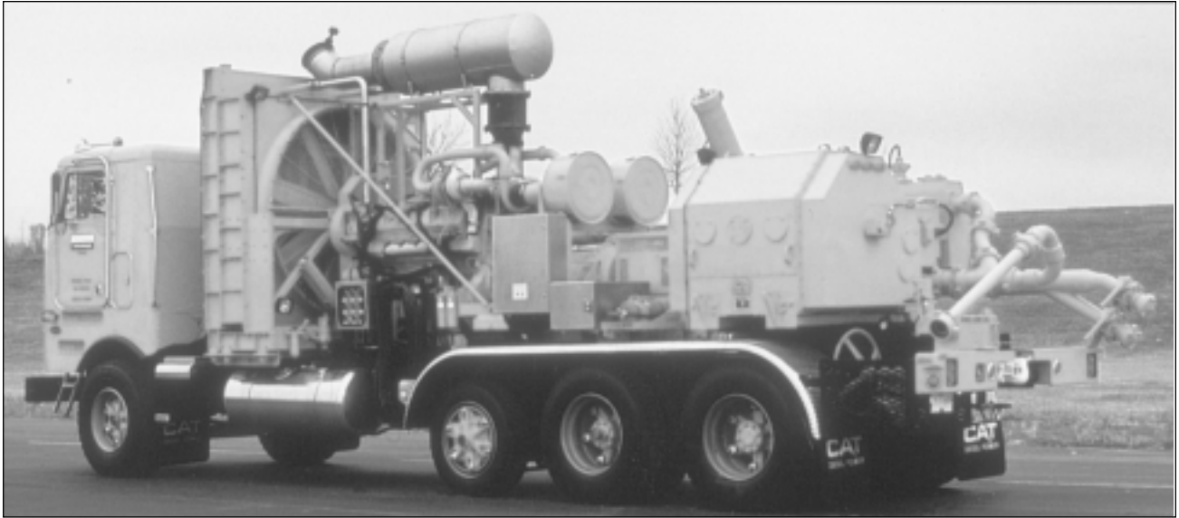
Figure 1-24. One thousand hydraulic horsepower pumping unit.
