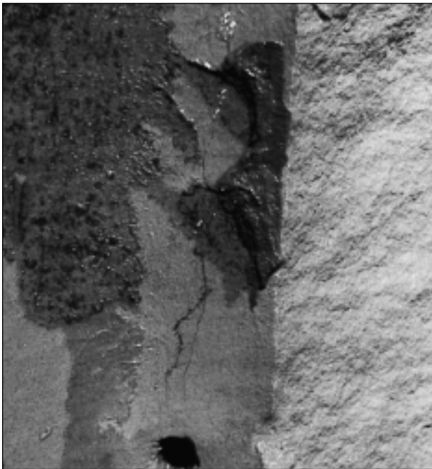
Figure 11-2. Disruption of the cement/sandface bond (fracture test) (Behrmann and Elbel, 1992). The dark areas are fracturing fluid that flowed around the wellbore annulus.
