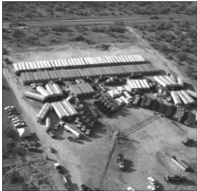
Figure 1-23. This large fracturing treatment used 25,000 hydraulic horsepower and 1.54 million gal of fracturing fluid to place 6.3 million lbm of propping agent. The job lasted 11 hours.
