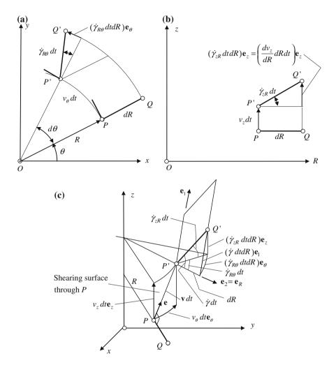
Fig. 4.18 Helix flow. Construction of shear rate and shear direction
