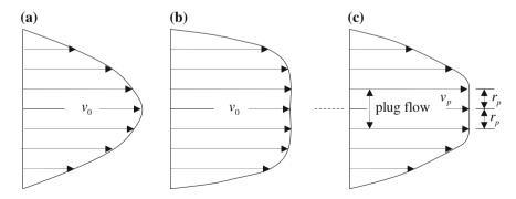
**Fig. 3.13** Velocity profiles in pipe flow. **a** Newtonian fluid, **b** power law fluid n = 0.2, **c** Bingham fluid
