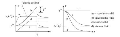
Fig. 1.13 Solid and fluid response in creep and relaxation
