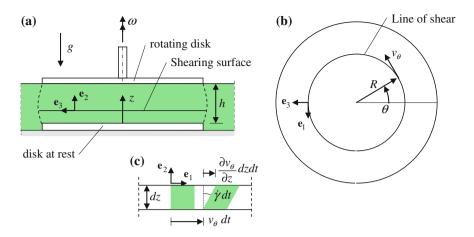
Fig. 4.16 Torsion flow between two parallel circular disks
