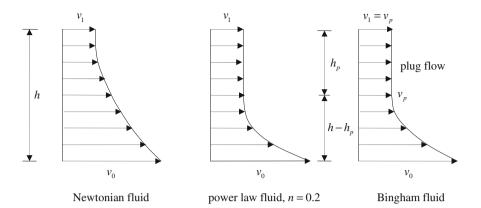
Fig. 3.15 Velocity profiles for film flow
