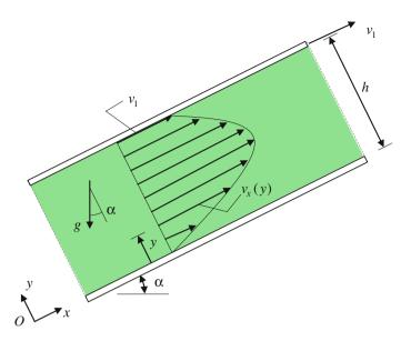
Fig. 3.9 Flow between parallel planes
