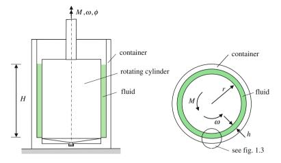
Fig. 1.2 Cylinder viscometer
