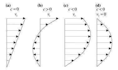
Fig. 3.10 Velocity profiles for a Newtonian fluid
