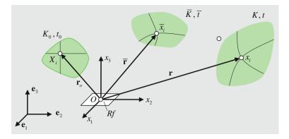
Fig. 3.1 Reference Rf, coordinate system Ox, configurations  $K_o, \bar{K}$ , and K, and base vectors  $\mathbf{e}_1, \mathbf{e}_2$ , and  $\mathbf{e}_3$
