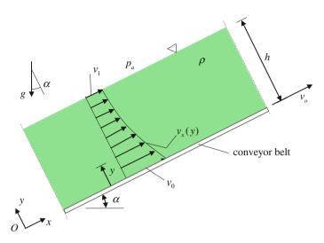
Fig. 3.14 Film flow on a conveyor belt
