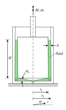
viscometer may be used to find the *viscosity function*  $\eta(\dot{\gamma})$  of the fluid. The rotating cylinder is subjected to a constant torque *M* and rotates with a constant angular velocity  $\omega$ .
