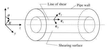
Fig. 4.13 Axial annular flow. Steady pipe flow
