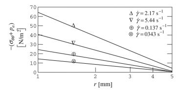
Fig. 5.8 Pressure measurements from a cone-and-plate viscometer. The fluid is 2.5 % polyacrylamide solution. The data are adapted from Bird et al. [3]
