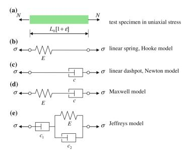
Fig. 7.4 Mechanical models
