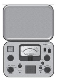
FIGURE 6.7.42 AM field strength meter.
