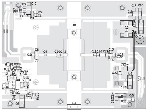
FIGURE 2.10.3 Circuit layout of a UHF amplifier.
