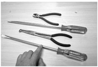
FIGURE 6.2.6 Oversized screwdrivers with a dull flat blade can be used to pry wires without damage. A special plier with provisions for grasping and fishing a wire out from deep in a tight bundle is especially valuable, but hard to find.
