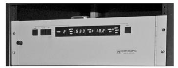
FIGURE 6.7.41 Typical AM antenna monitor, which measures the phase and ratio for each tower in a directional array.
