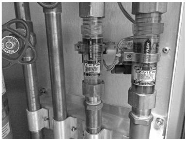
FIGURE 6.7.33 Flow gauges inside a transmitter.
