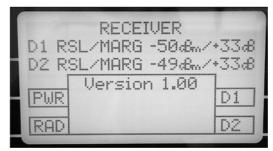
FIGURE 6.7.28 STL signal strength readout.
