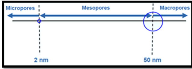
Figure 2.18 Size of pores (IUPAC Standard) [34].
