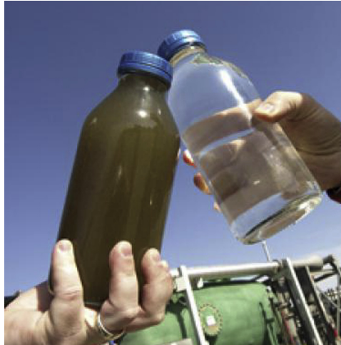
Figure 10.12 Produced water (left) and treated water from an evaporator [42].
