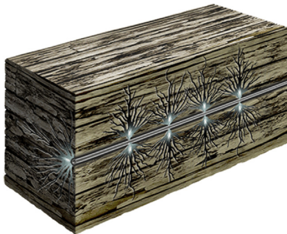
Figure 3.15 Crack propagation within rock formation [29].
