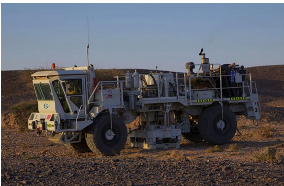
Figure 3.3 Nomad 90 seismic vibrator [4].
