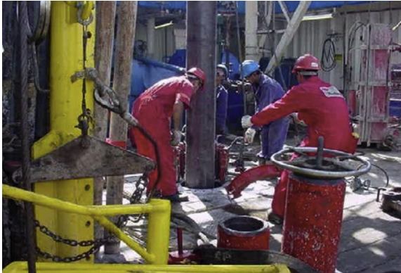
Figure 3.8 Onshore personnel stacking drill string to be lowered into a well.
