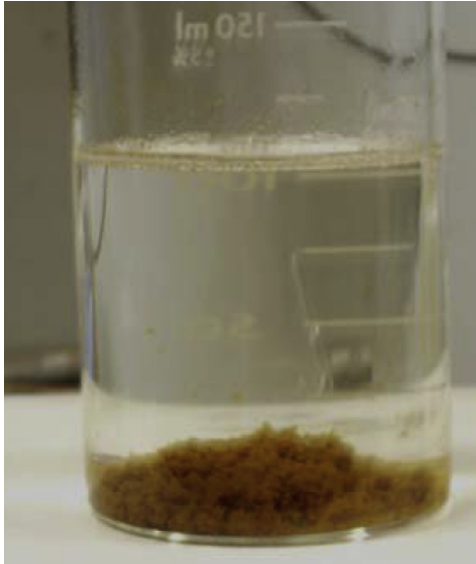
Figure 10.13 Barium precipitate from Marcellus Shale produced water [38].
