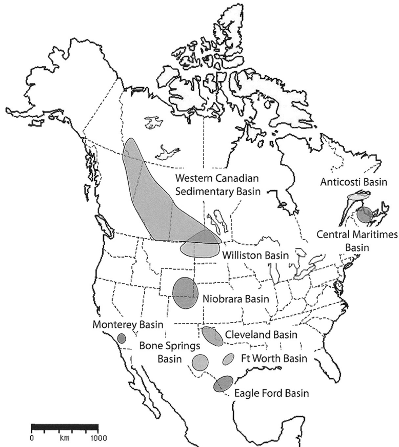
FIG. 10.2 Major basins with the potential for tight oil development. Source: Adapted from US EIA, 2012. Energy Information Administration, United States Department of Energy, Washington, DC.
