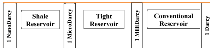
FIG. 1.2 Representation of the differences in permeability of shale reservoirs, tight reservoirs, and conventional reservoirs.
