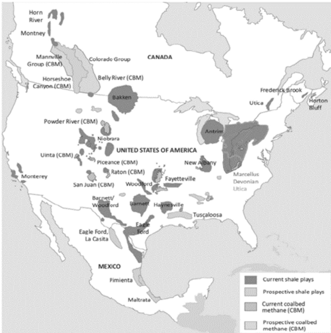
FIG. 2.3 Shale gas resources (shale gas plays) in the contiguous United States, Canada, and Mexico. Adapted from US EIA (2012). Energy Information Administration, United States Department of Energy, Washington, DC.
