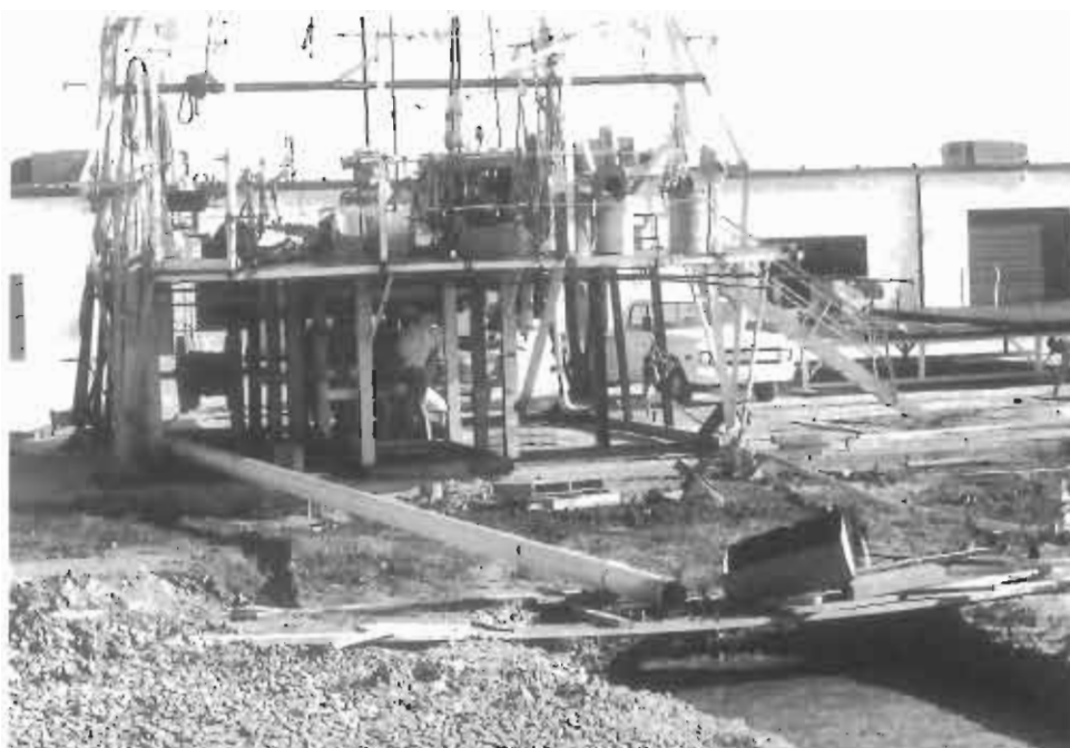
Earthen Mud Pits. A drilling rig in East Texas drilling a 2,800-foot well using earthen mud pits. Cuttings, for geological examination, were collected on a piece of hardware cloth at the end of the flow line. Solids control equipment was not used on this well.
