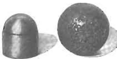
Left: "K" Monel drop valve after 14 months' service in oil well, pumping corrosive crudes, salt water, and hydrogen sulfide. Spherical ball to its right shows the effect of the same crude on a steel ball after 3 days. Maximum life in this field for materials other than "K" Monel is approximately 43 days.
