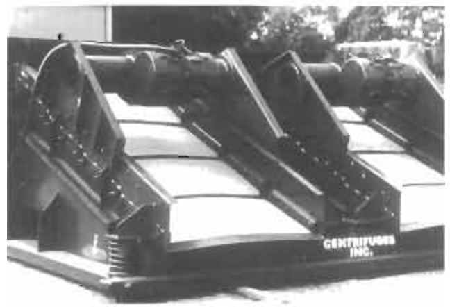
Centrifuge Inc. unbalanced elliptical motion shale shaker.
