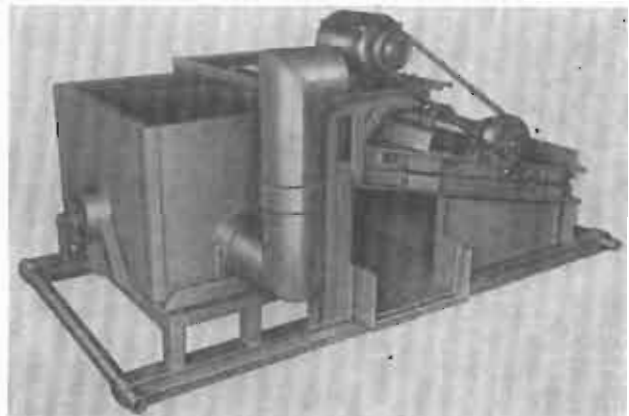
This rear and side view of both large and small model shakers shows the collar welded in the back of the mud tank to which the 8 1/2" O.D. 8 V thread flow line from the well is to be connected. This design saves building mud troughs and a lot of rigging-up time. The mud by-pass is shown in the up position to run the mud over the screen cloth.
