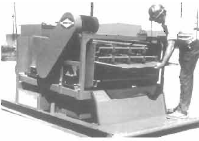
IMCO triple-deck shale shaker. Designed by Louis Brandt prior to starting The Brandt Company where he designed the Brandt double-deck shale shaker.
