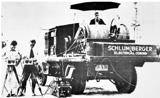
Fig. 13.12 Early Schlumberger logging unit in the California Desert (from [13.10], courtesy of SPWLA)
