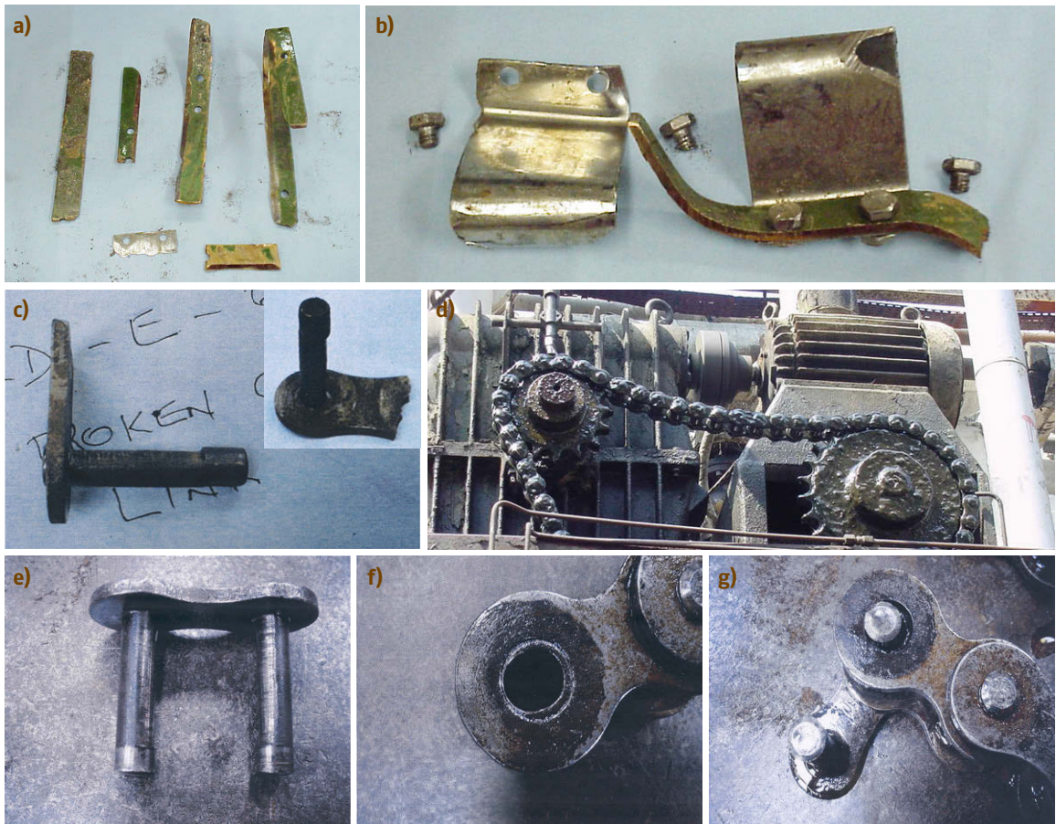
Fig. 33.44a-g Examples of damages in SSEs. (a) Damaged scraper blades, (b) damaged scraper leaf springs and blades, (c) broken chain link, (d) chain drive, (e) chain link wear, (f) bushing wear at chain link, (g) link and pin slack
