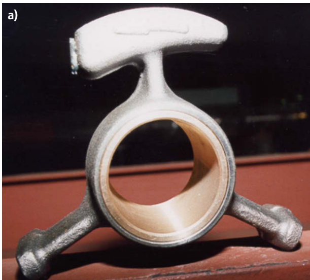
Fig. 33.37a,b Intermediate bearing design in an SSE. Side view of intermediate bearing (a), top view of intermediate bearing (b) (Photo courtesy of BORSIG)
