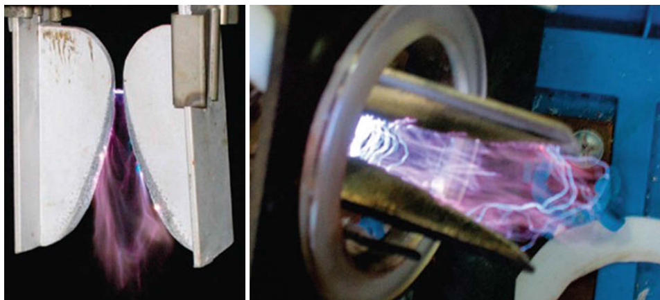
Fig. 41.1 Images of plasma processes. Gliding arc plasma discharge over water. Reprinted with permission from [41.59]. Copyright (2008) American Chemical Society
