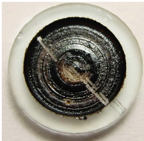
Fig. 6.10 All asphaltene sample is volatilized in L 2 MS experiments. The desorption IR laser track going from upper left to lower right establishes that bare metal remains after desorption. Reprinted from [6.35], Copyright 2015 American Chemical Society
