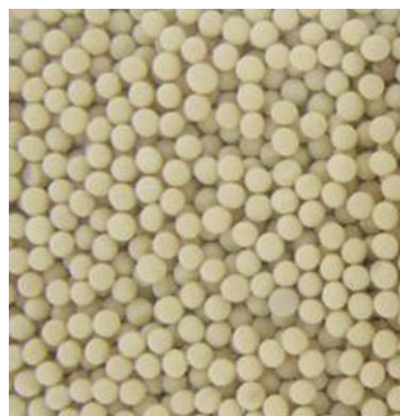
Fig. 18.41 Typical picture of an oxychlorinated catalyst
