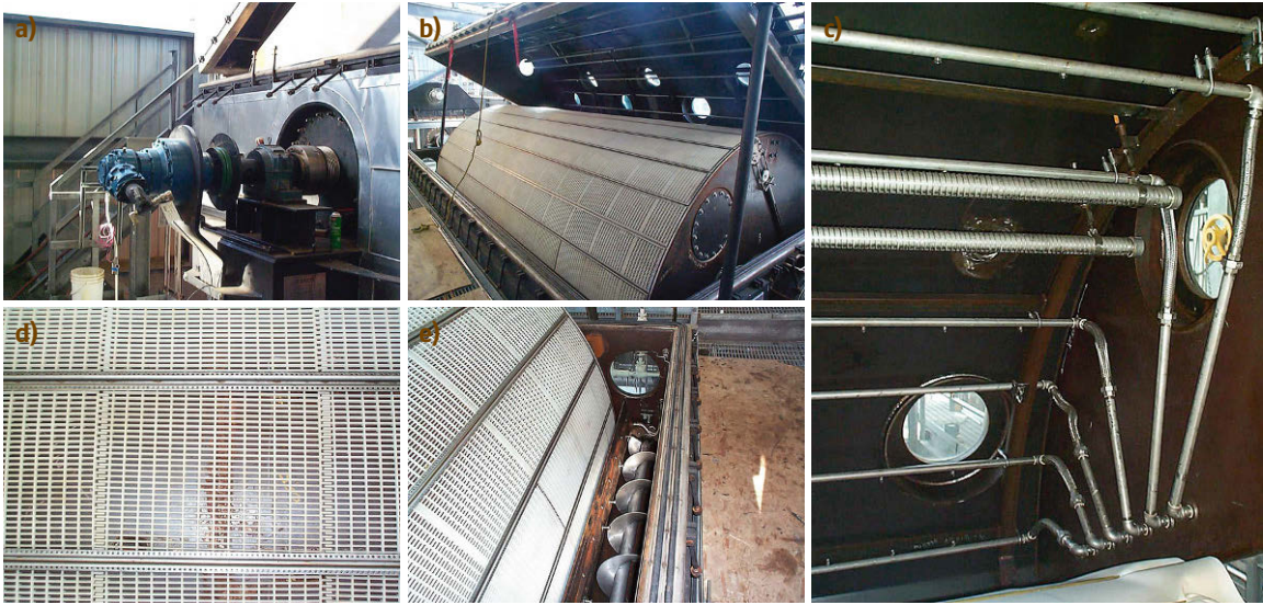
Fig. 33.47a–e Typical rotary vacuum filter. (a–b) Filter drum (c) solvent wash sprays and drip pipe (d,e) support grid and wax scroll. (Photos by B.E. Beasley, courtesy of ExxonMobil Process Research)
