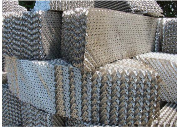
Fig. 16.6 Structured packing for distillation (© Luigi Chiesa)
