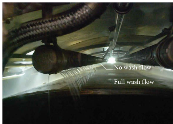
Fig. 33.51 Example of poor filter cold wash distribution. (Photo by D.S. Sinclair, courtesy of ExxonMobil Process Research)
