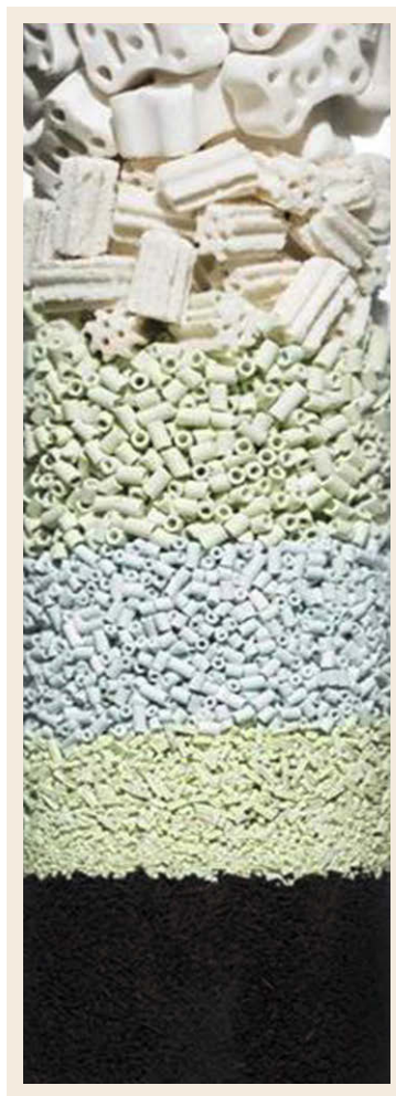
Fig. 22.27 Catalyst grading scheme for the first bed of a fixed-bed catalytic hydrotreater (courtesy of Haldor Topsøe A/S)
