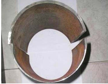
Fig. 33.42 Tube damage resulting from spider bushing failure. (Photos courtesy of Armstrong)
