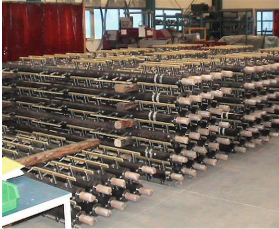
Fig. 33.35 Scraper shafts ready for packing. (Photo courtesy of BORSIG)
