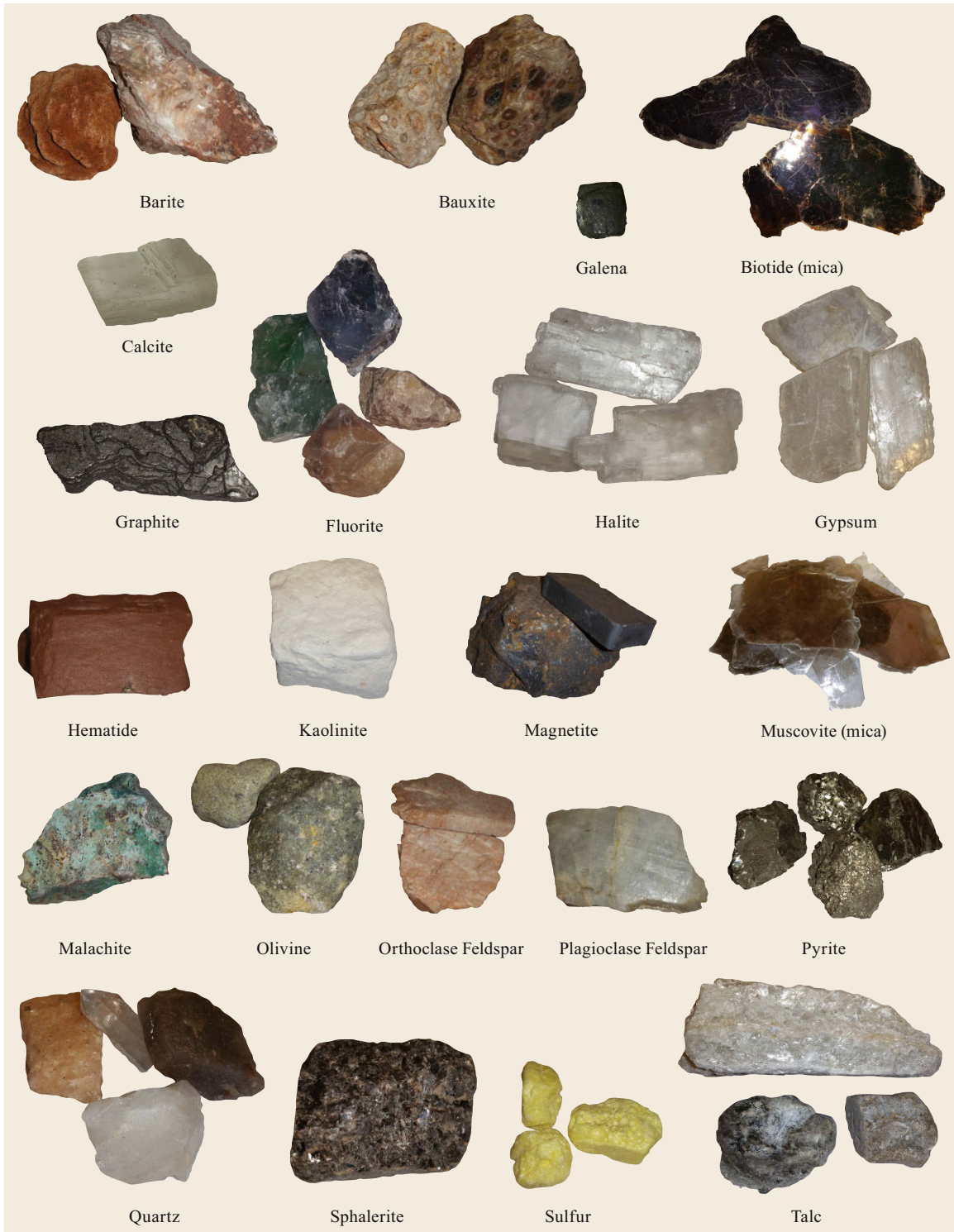
Fig. 9.8 Examples of common minerals: Note the colors and distinctive appearance of some of the minerals
