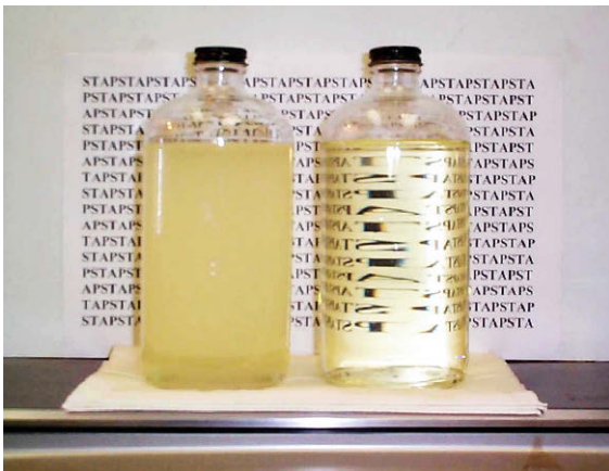
Fig. 33.22 Comparison of immiscible and miscible filtrates. (Photo by B.E. Beasley, courtesy of ExxonMobil Process Research)
