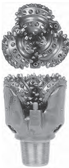
FIGURE 4.7.2 Typical roller cone bit cutting structure.
