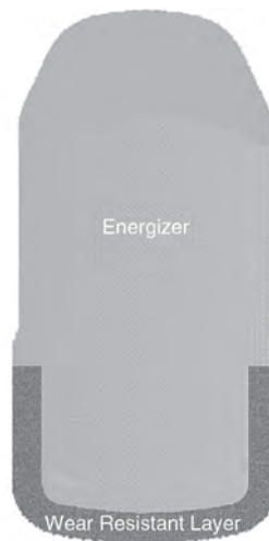
FIGURE 4.7.43 Cross-section of modern bi-material seal.
