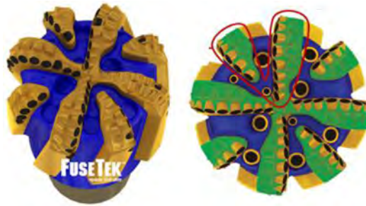
FIGURE 4.7.91a Hybrid Bit (FuseTek) - combination of PDC and impregnated diamond material (courtesy of ReedHycalog – NOV).
