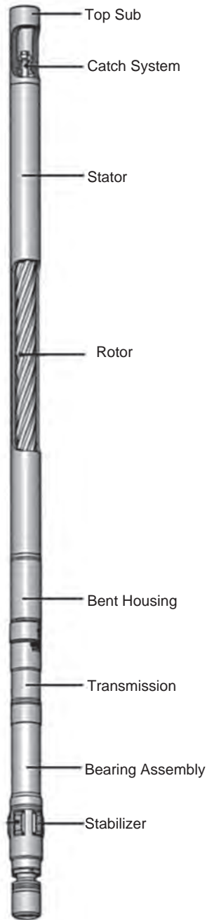
FIGURE 4.12.12 Downhole positive displacement motor ( Courtesy of Archer Directional ).
