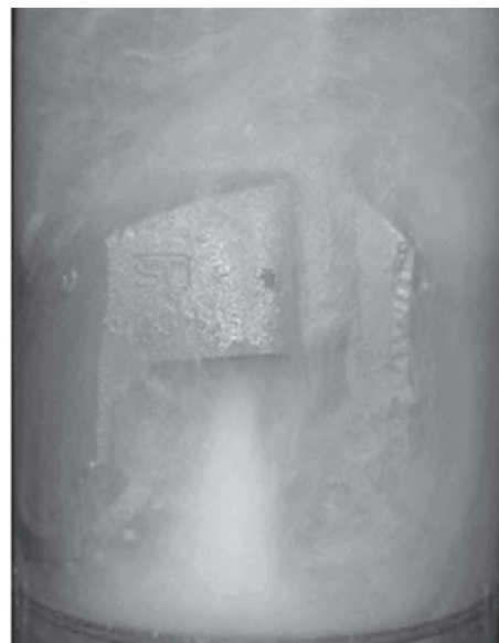
FIGURE 4.7.4 Hydraulic flow around bit body.
