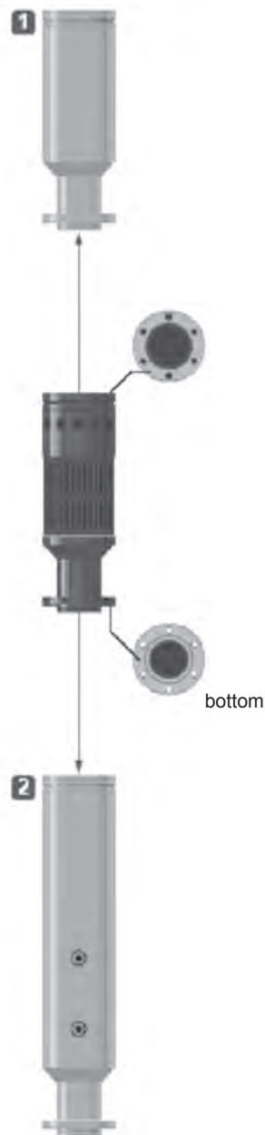
FIGURE 6.4.69 Typical ESP installation.
