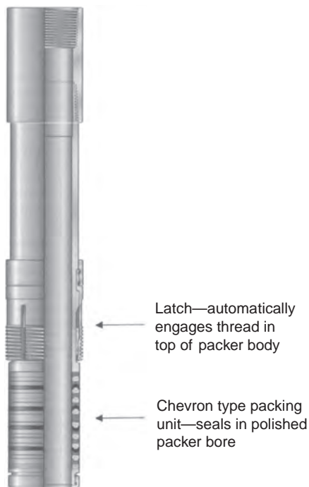
FIGURE 4.9.4 Latching seal assembly [2,3; Figure 2.11, p. IV-55, PEH].
