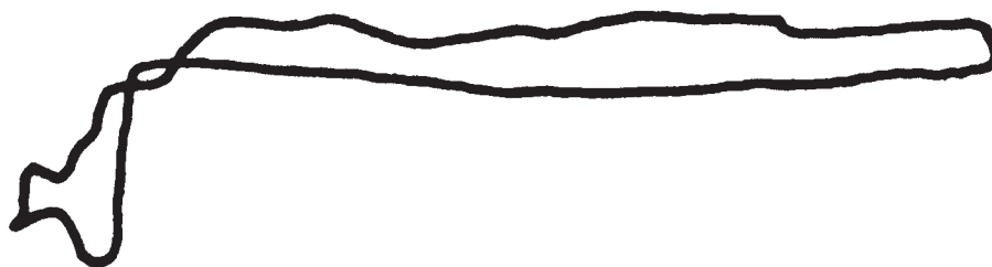
FIGURE 6.4.22 Severe case of fluid pound [2].
