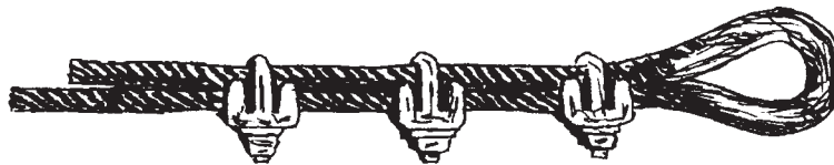
FIGURE 4.2.68 Correct method of attaching clips to wire rope [3].
