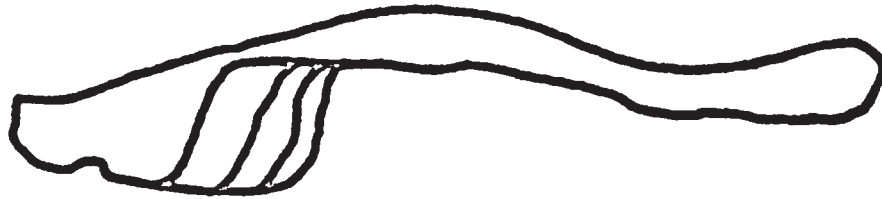
FIGURE 6.4.24 Example of well pumping off [2].
