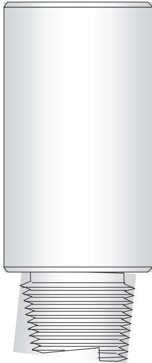
FIGURE 4.15.7 Cutlip Screw in Sub. (Courtesy Weatherford International).
