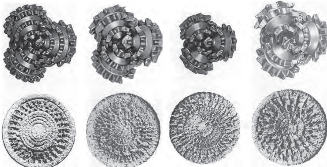
FIGURE 4.7.27 Soft and hard formation cutting structures.
