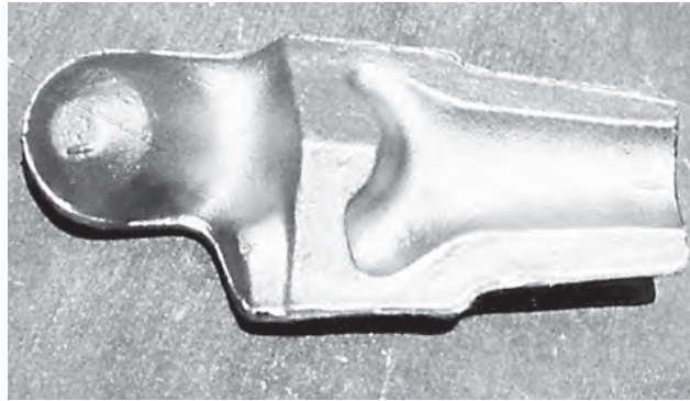
FIGURE 4.7.19 Roller cone bit leg forging (three required).
