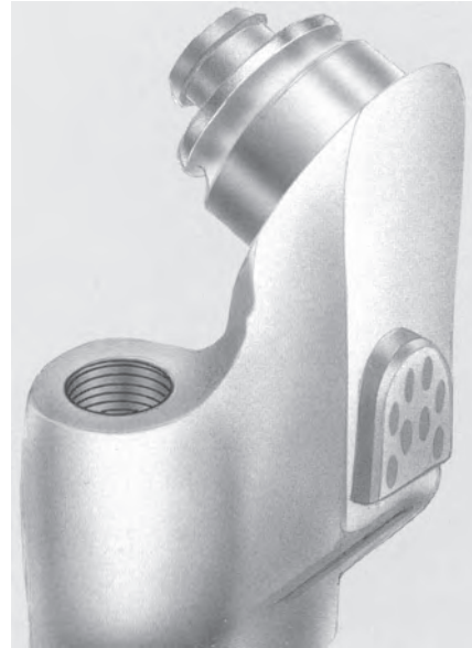
FIGURE 4.7.48 Typical lug pad with tungsten carbide inserts.
