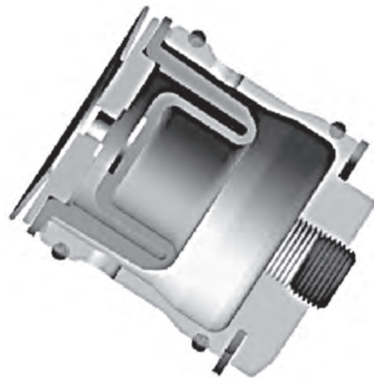
FIGURE 4.7.45 Typical roller cone bit lubricant reservoir.
