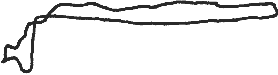
Figure 6-132. Severe case of fluid pound [61].
