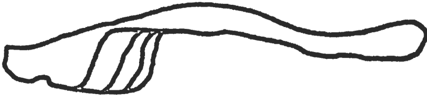
Figure 6-134. Example of well pumping off [61].
