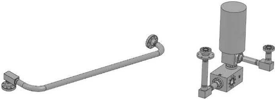
Figure 25-7 Crossover Loop (Left) and Production Loop (Right).
