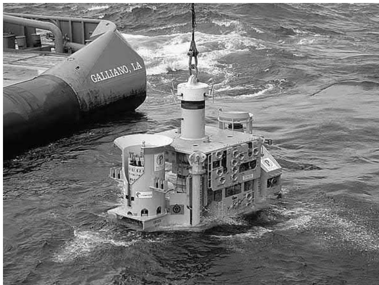
Figure 6-12 A Subsea Tree Being Deployed [5].
