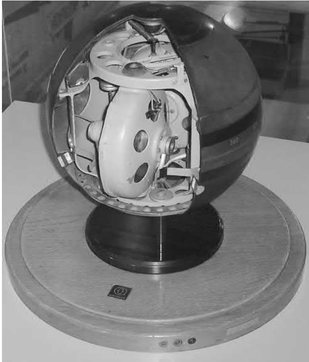
Figure 4-2 Cutaway of Anschütz Gyrocompass [2].
