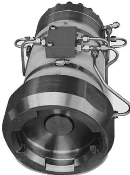
Figure 27-22 Linear Actuator Override Tool. Courtesy of Subsea 7 Inc. [8].
