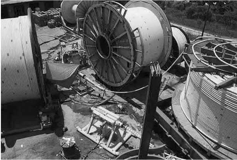
Figure 28-9 System Integration Testing of Control Umbilical.
