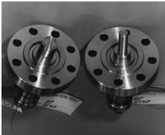
Figure 7.21 Temperature Transducers (TT).
