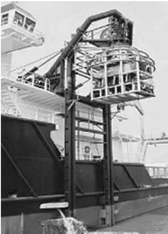
Figure 27-7 Guide Rail System [10].
