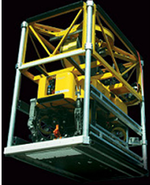
Figure 23-9 Side Entry (Garage) Type TMS with ROV Parked (Courtesy of SMD Robotics Ltd. [12])
