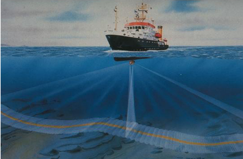
Figure 4-3 MBES Working Model [5]
