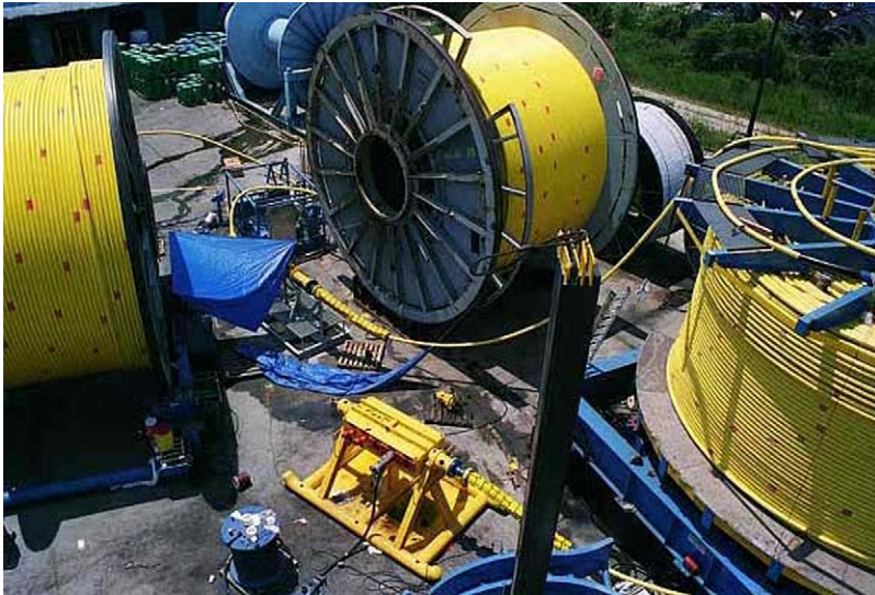
Figure 24-9 System Integration Testing of Control Umbilical
