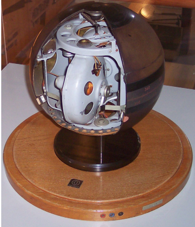
Figure 4-2 Cutaway of Anschütz Gyrocompass [2]
