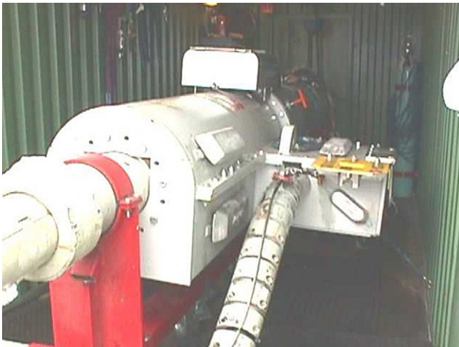
Figure 3-4 Umbilical Termination Head (UTH) [2]
