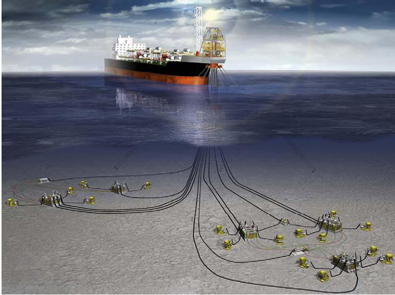
Figure 2-7 Subsea Tie-Back to FPSO [2]
