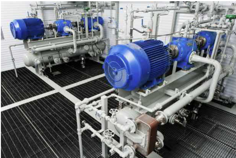
Fig. 7.7 Typical vane rotary compressor.
