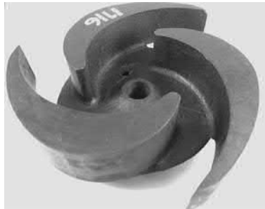
Fig. 3.76 Open impeller with partial shroud.
