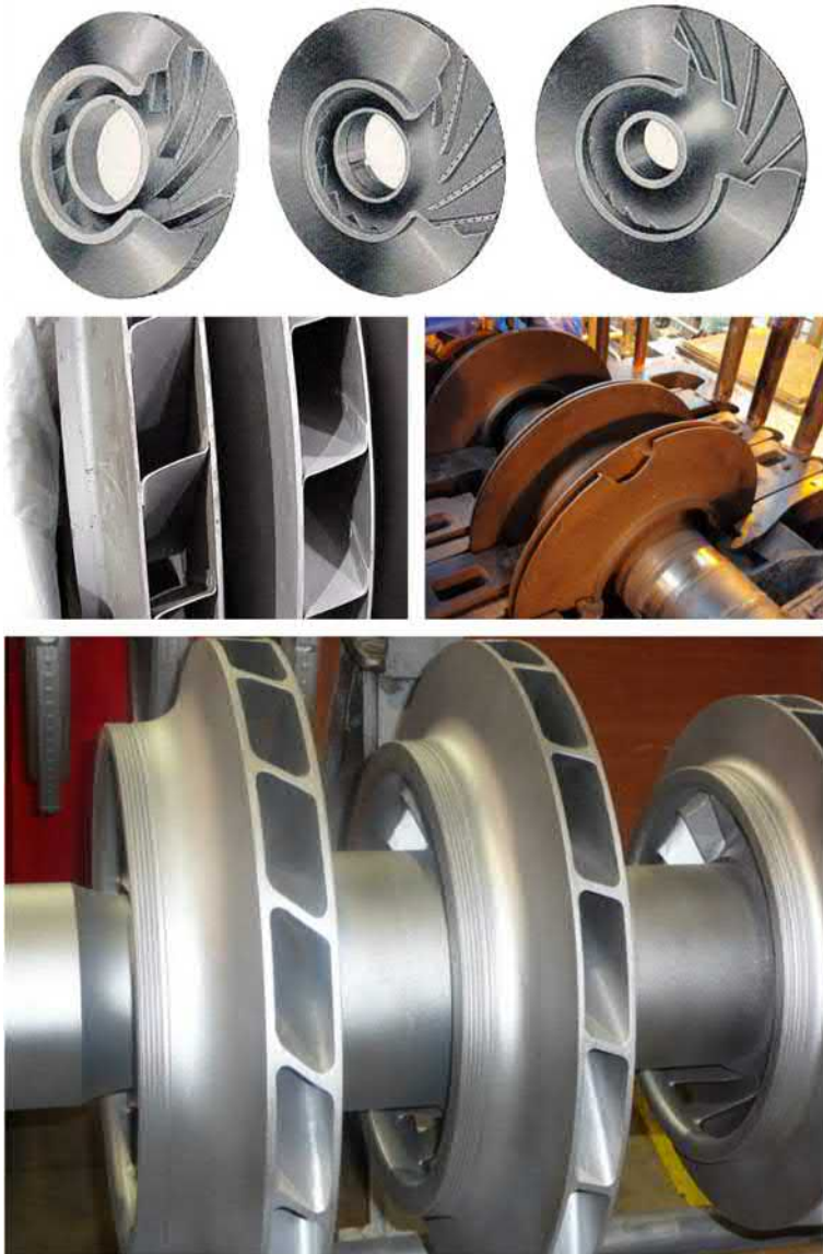
Fig. 8.22 Top: Welded, riveted, and milled impellers; Center: Left-riveted impellers, Right-damaged riveted impeller; Bottom: Fillet-welded closed impellers.
