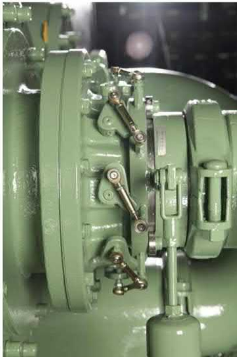
Fig. 8.104 Inducer blades (adjustable guide vanes).
