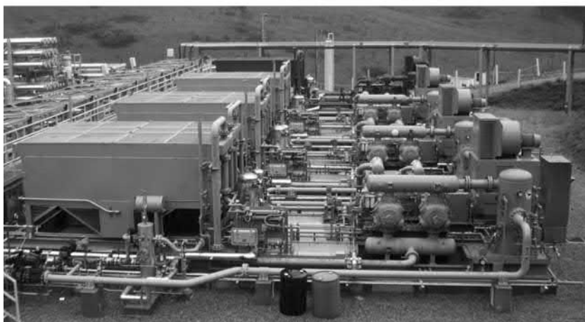
Fig. 7.4 Examples of high-speed reciprocating compressor packages. Courtesy of Dresser Rand Co.
