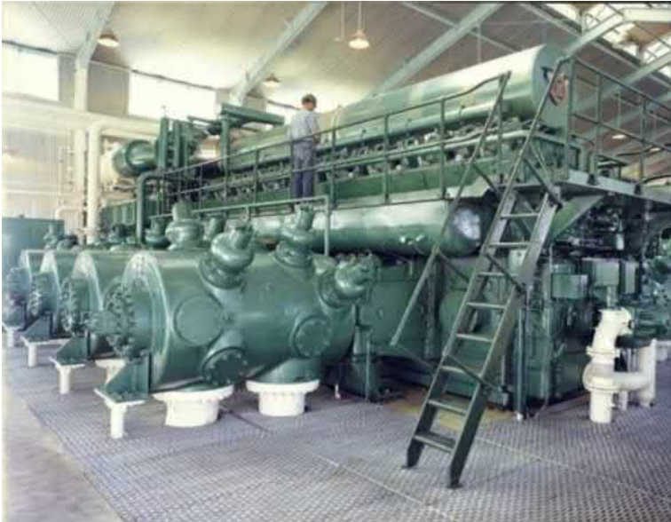
Fig. 7.6 Low-speed integral engine compressor. Courtesy of Cooper Industries Energy Services Group.
