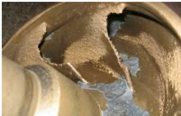
Fig. 3.50 Cavitation damage as a result of low flow recirculation.
