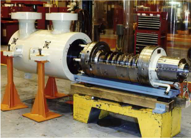
Fig. 7.10 Radially split centrifugal compressor.
