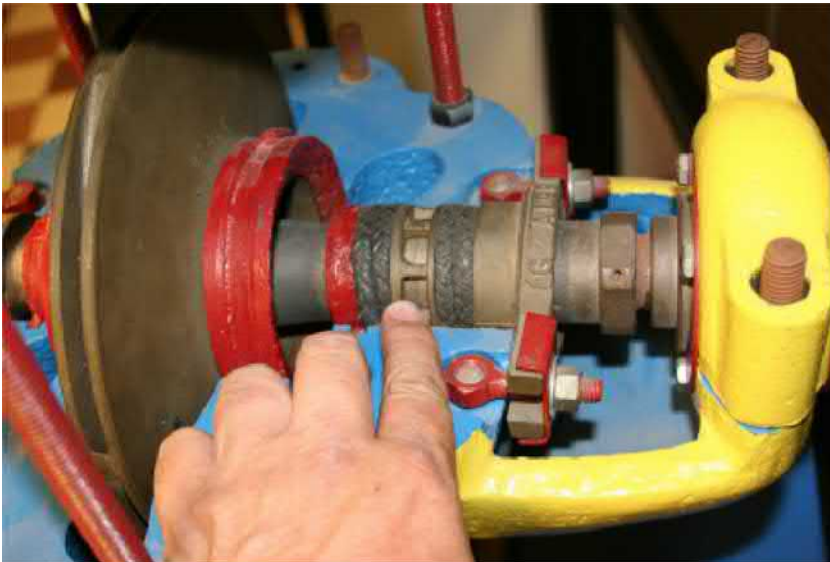
Fig. 3.95 (Top) Lantern ring-Lantern ring; (bottom) lantern ring installed in stuffing ox.
