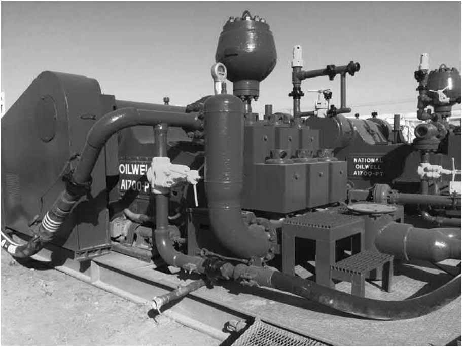
Fig. 4.60 Example of a quintuplex pump installation showing a liquid surge suction and discharge dampener.
