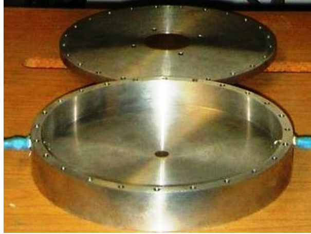
Figure 3.54 The opened resonant cavity.
