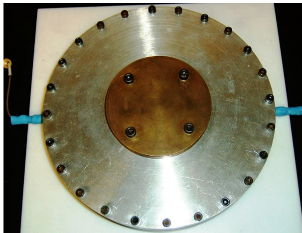
Figure 3.53 The actual resonant cavity.
