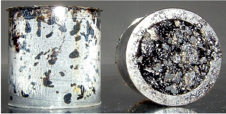
Figure 3.58 The asphalt sample and its sample holder.
