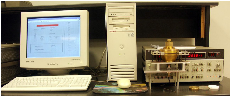
Figure 3.27 Workstation for the low-frequency measurement (the HP4275A LCR Meter).
