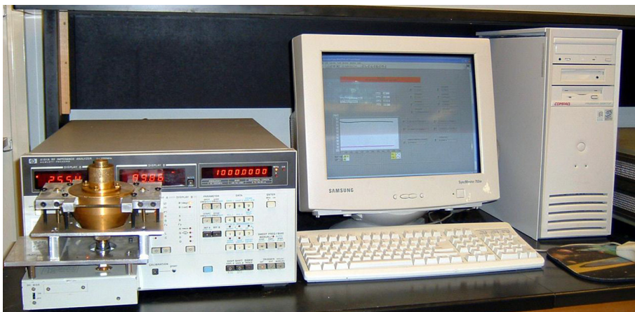
Figure 3.28 Workstation for the high-frequency measurement (the HP4191A RF Impedance Analyzer).
