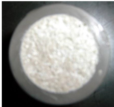
Figure 3.59 The mortar sample and its sample holder.
