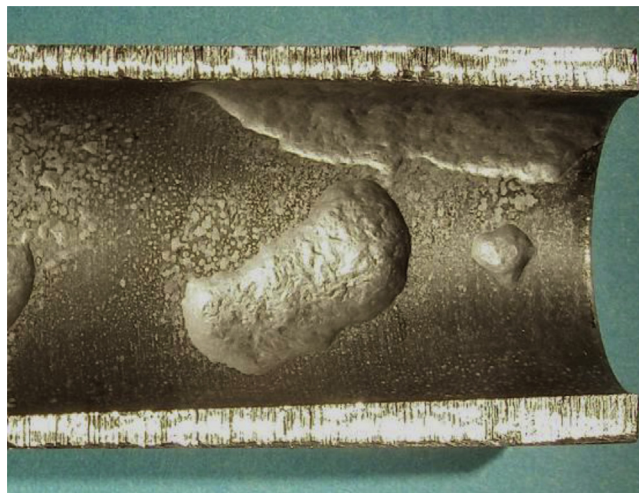
Figure 6.4 Wide pits formed in a sour pH stabilization experiment with 0.5 bar H 2 S, 5 bar CO 2 , 5000 ppm Cl - , pH ~7, 60°C, and 1 m/s flow rate [46].
