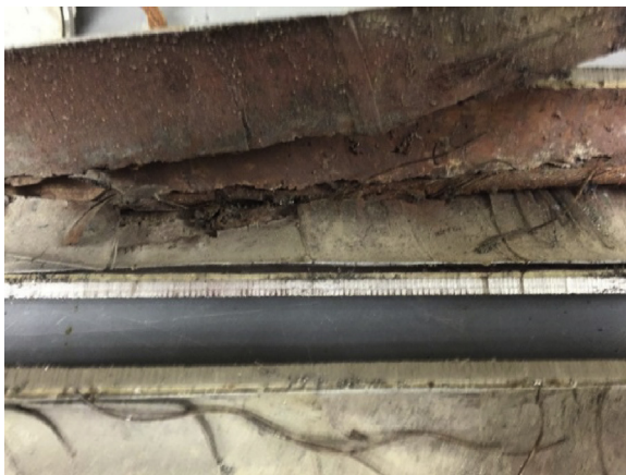
Figure 27.6 Example of failed fiber-reinforced plastic liner in downhole tubing.
