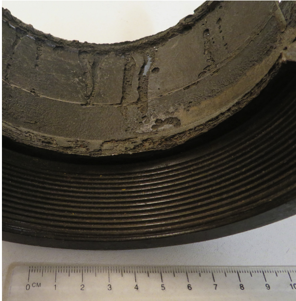
Figure 4.3 Flow enhanced corrosion, L-80 carbon steel, gas condensate well. Photograph © Hollybeach Corrosion Management. Used with permission. All rights reserved.
