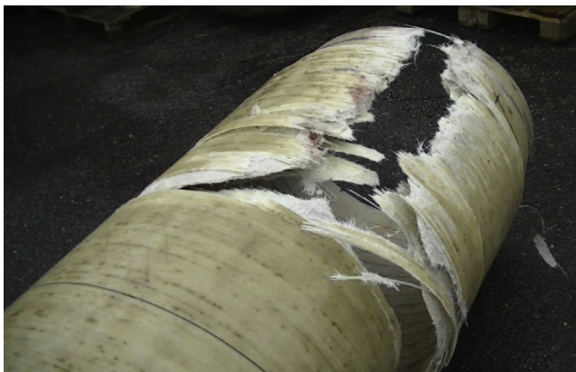
Figure 33.8 Detail of the failure zone.
