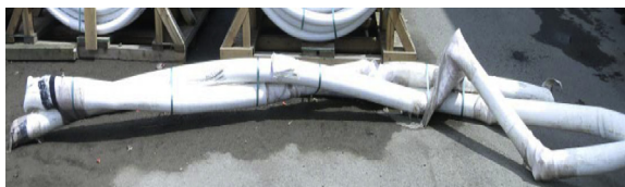
Figure 27.10 Example of reinforced thermoplastic pipe line failure due to kinking.
