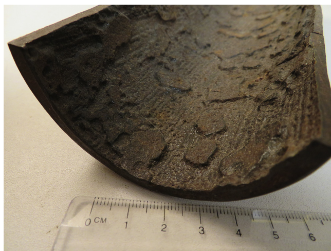
Figure 4.2 Mesa corrosion of flow line.
