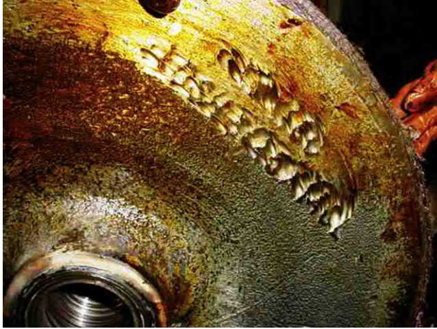
Fig. J.54 Discontinuities on an impeller shroud surface can create Kamm type vortices. Here cast identification lettering has generated substantial damage. Elsewhere the original cast surface shows little if any damage [see also Fig. J.130 ].
