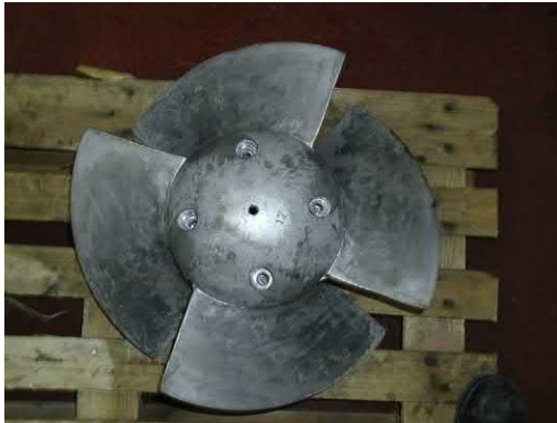
Fig. 3.34 Above, say, 8000 specific speed are called axial flow, or propeller pumps.
