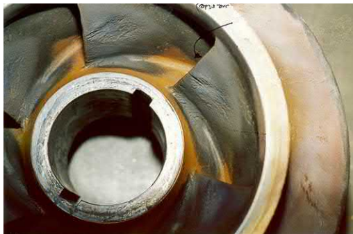
Fig. J.30 Heavy off design flow damage.
