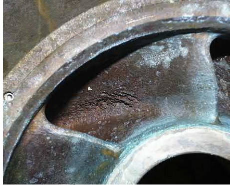
Fig. J.28 Heavy cavitation damage at passage inlet throat. Again implies high cavitation intensity.
