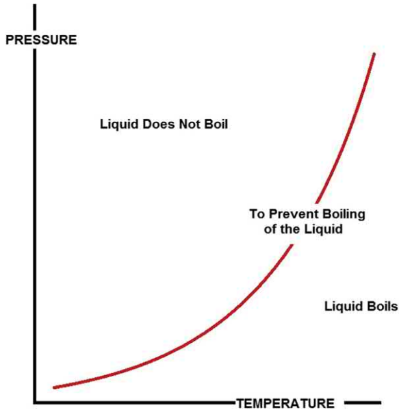
Fig. 5.20 Typical vapour pressure curve.
