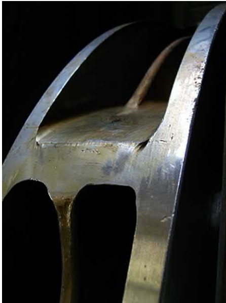
Fig. J.57 More developed twin vortex damage on this double entry impeller river water pump. Elsewhere little damage is visible. This indicates the high damage potential of vortices in the flow.
