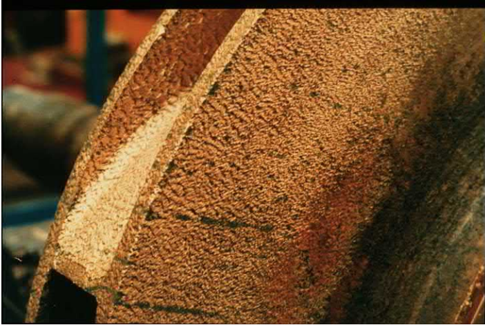
Fig. J.52 Low impact angle attack on the bronze impeller shrouded a pump handling very fine river water silt. The damage rate increase with distance from the shaft – in conjunction with increased velocity.
