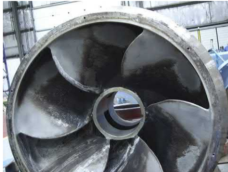
Fig. J.29 Light 'off-design' —low flow damage. Note damage intensity is related to radius from shaft i.e., peripheral velocity.
