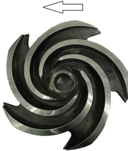
Fig. 3.20 Modern impellers utilise backward curved blades for more efficient liquid guidance. This impeller blade surface has only two dimensional curvature-unlike Fig. 3.18.
