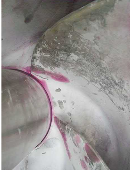
Fig. J.38 Micro cracking at the vane intersection with the hub disk is here revealed by dye penetrant. [C K Verma].
