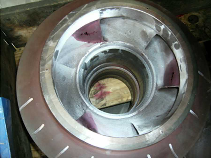
Fig. J.37 Only Alternate vanes show cavitation damage. This is quite unusual. Obviously it will only occur in impellers with even vane number.
