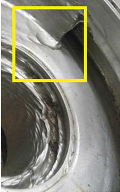
Fig. J.110 This hydrocarbon process pump shows HSV damage near the cutwater lip, as well as ring-type vortex attack.
