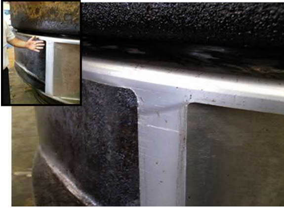
Fig. J.56 Stains on this large cooling water impeller indicate early stage of twin vortex erosion.
