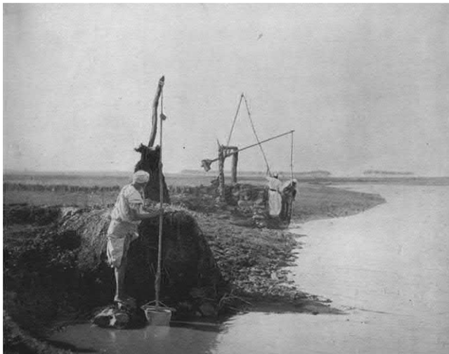
Fig. 2.1 The Shadoof. This is probably the first widely used pumping machine. Its origins are lost in time, but the device became prolific in the Middle East. The suspended bag is periodically dipped into the river. When full, the counter-weighted swivel arm helps lift the bag over and above an irrigation canal. ( Reproduced from Wikipedia. )
