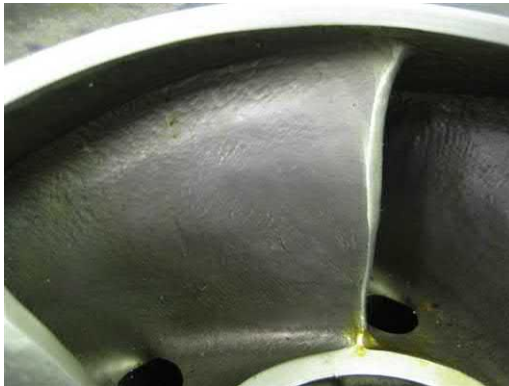
Fig. J.70 Further example of high impact angle damage. The sharp inlet edge shape has been largely destroyed.
