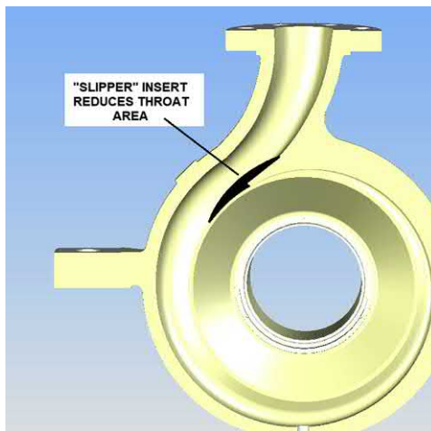
Fig. K.16 Attaching pre-formed insert to the volute casing is an efficient and effective approach to area reduction.
