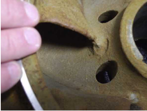
Fig. J.22 Horseshoe Vortex at junction of vane leading edge with impeller hub. There is little evidence of any other significant erosion from other causes. Even the cast passage surface appears largely intact. This illustrates the damage potential of vortices.
