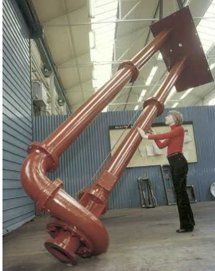
Fig. 8.30 Vertical sump pump with continuously lubricated grease journal line shaft bearings.
