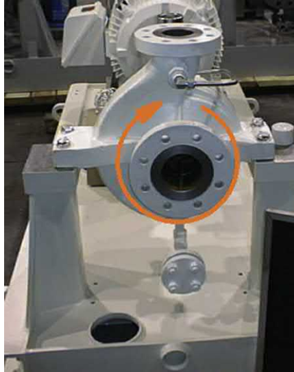
Fig. 8.36 Single suction overhung impeller pump.
