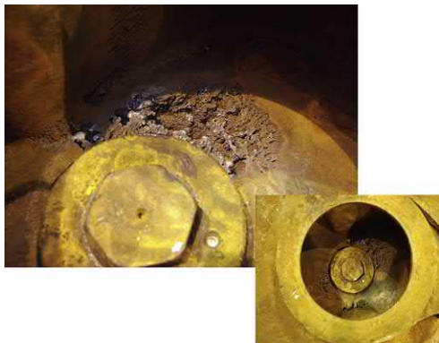
Fig. J.18 In this Sewage pump impeller, the damage is not caused by particle erosion, but by cavitation. Sewage pump impeller profiles are often severely compromised from the ideal in order to better handle a very wide range of suspended items. This can result in poor cavitation resistance.
