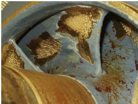
Fig. J.26 Intense low flow cavitation damage on concave [visible] face, plus damage in area of passage inlet throat. This pump has probably been operating over a range of flow conditions in order to experience these two different damage patterns.
