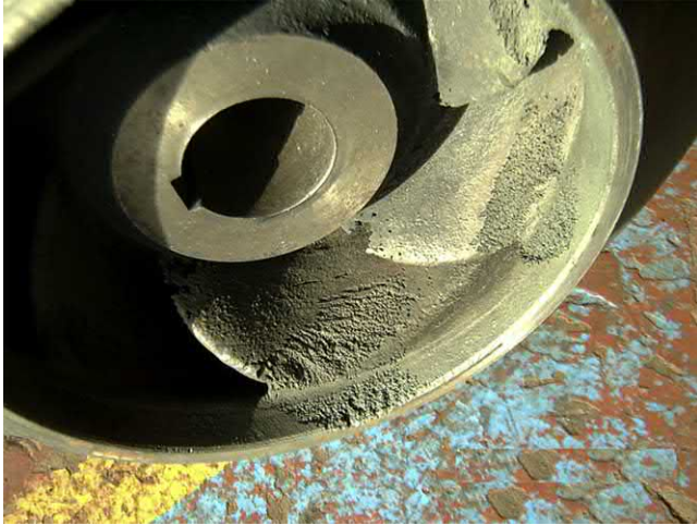
Fig. J.24 Cavitation damage ahead of the impeller vane leading edge is usually evidence that the impeller has been operating inside the Backflow Regime. Cavitation can form in the filamentary vortex cores created along the interface between the incoming and outgoing liquid masses. It is then swept out ahead of the impeller before collapsing. [See also Fig. D.9].
