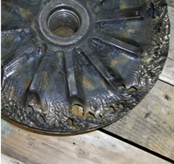
Fig. J.80 This shows the damage that Von Karman type vortices can cause if the back pump out vanes does not extend to the maximum diameter.
