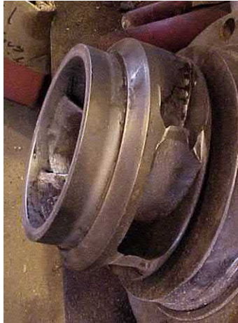
Fig. J.58 Advance twin vortex damage to this single suction API 610 Process pump handling Catalyst fines. [ Union Pumps ].
