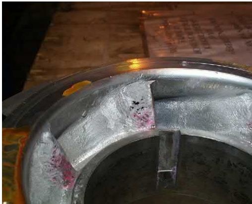
Fig. J.35 As before, little pitting on the visible face. Great amount of pitting on the reverse side, ultimately penetrating through to the front.
