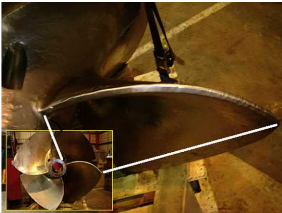
Fig. J.72 On this example, the edge has not been eroded to a flat shape. Instead, a wedge profile has developed on this axial flow impeller inlet edge. As before the ridge is evident. [ Sulzer Pumps ].
