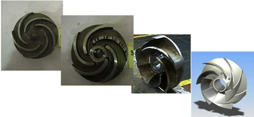
Fig. 4.17 Semi-open impeller designs are also available in a wide range of Specific Speeds, ranging from Low [ narrow relative to diameter ] to High [ wide relative to diameter ]. Because very Low Specific Speed closed impeller are very narrow relative to diameter, they can be difficult to cast, so semi open designs are the only practical option.
