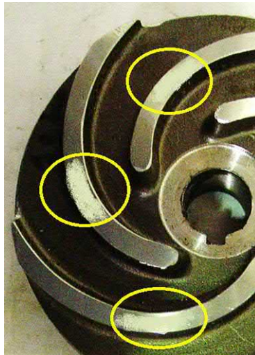
Fig. J.83 In some conditions, this gap flow will result in cavitation. Localised damage will be evident on the machined face of the impeller vanes. The cavitation cell rotates with the impeller and cause corresponding damage over 360 degrees of the casing. See Fig. J.129 .
