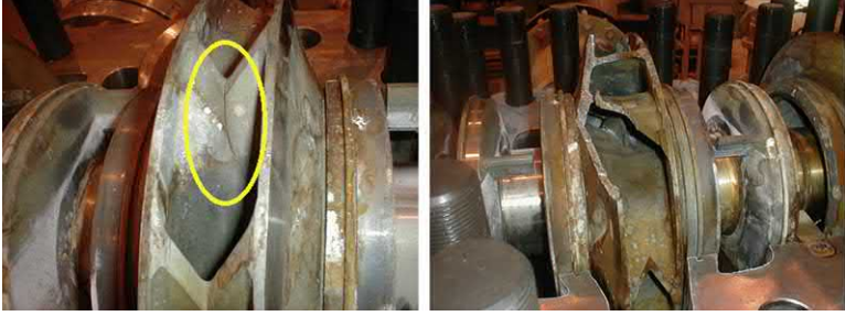
Fig. K.37 The notch formed by a conic trim on a double suction impeller can be the source of fatigue cracks. The pressure pulsations resulting from impeller – collector flow interactions will propagate these cracks.
