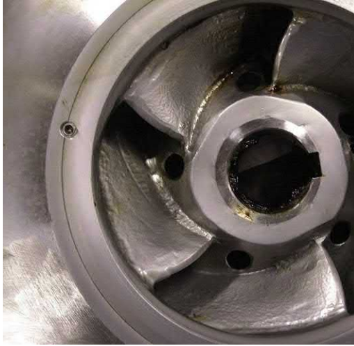
Fig. J.69 An example where the inlet edge has lost its smooth profile due to high impact angle erosion.
