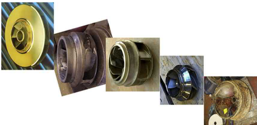
Fig. 4.16 Closed or Shrouded impeller designs are available in a wide range of Specific Speeds, ranging from Low [narrow relative to diameter] to High [wide relative to diameter].
