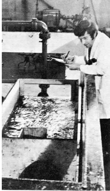
Fig. 10.30 Sumps model testing can help eliminate air-entraining vortices [The author in his younger days]. Photograph: Sigmund Pumps.
