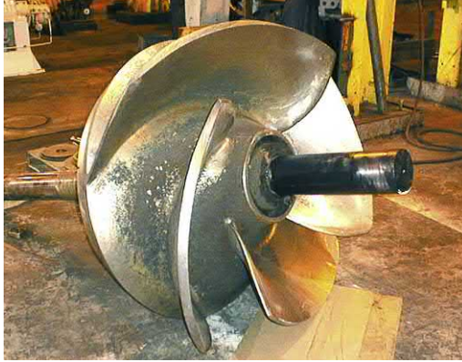
Fig. 3.33 Between specific speed of 4000 and 8000, the inlet and outlet diameter are becoming similar.
