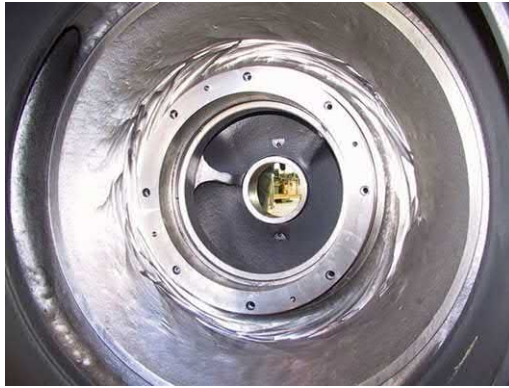
Fig. J.115 This 'between bearings' double suction pump suffered localised damage to both the casing and its cover. The rest of the casing has only suffered slight low impact angle damage.
