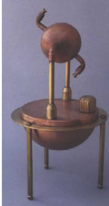
Fig. 2.2 The Aeolipile of HERO. Liquid was stored in the hemispherical base. When this was heated, steam rose up the hollow supporting legs and into the spherical section. Steam then issuing from both the jets caused the sphere to rotate. (Reproduced from Wikipedia.)
