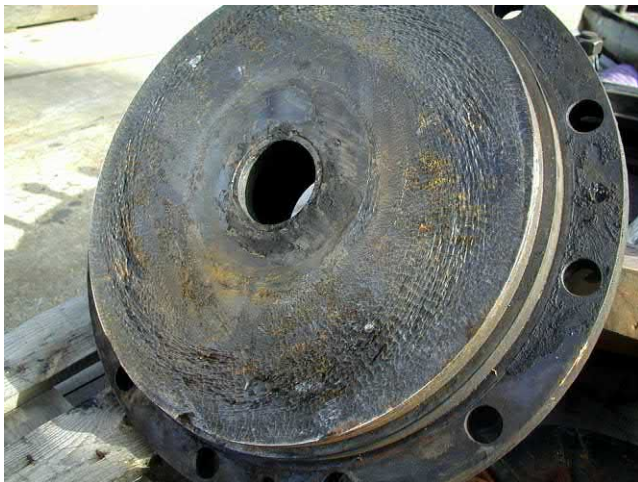
Fig. J.98 Further example of low impact angle damage. [David Brown Pumps].
