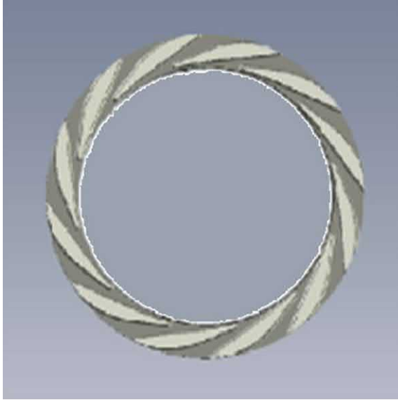
Fig. 3.10 Multiblade diffuser design. Blades are set to match the fluid angle leaving the impeller at the pump's design flow.
