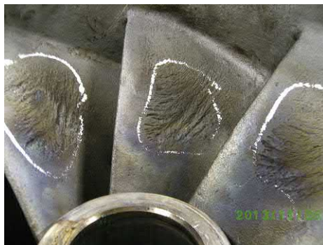
Fig. J.27 Heavy centralised cavitation damage implies that pump has been operating at significantly off-design at low flow.
