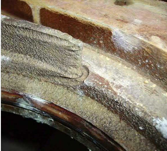
Fig. J.121 Classic horseshoe vortex wear and undercutting at junction of vane and hub disk.
