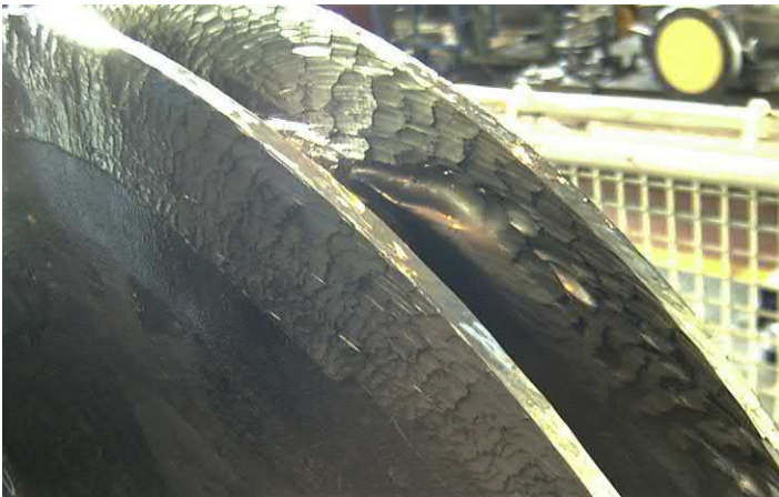
Fig. J.53 This process pump impeller has suffered low impact angle attack from suspended fine coke particles. [David Brown Pumps].
