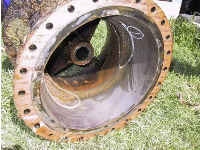
Fig. J.126 Casing damage from tip leakage cavitation of mixed flow semi-open impeller. [ Weir Engineering Services ].
