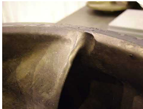
Fig. J.20 Another example of significant horseshoe vortex damage attacking the vane inlet tip junction.
