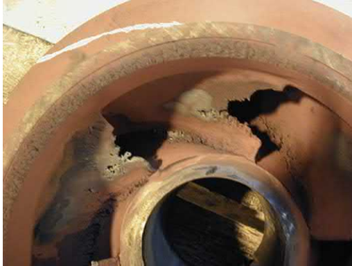
Fig. J.34 There is a lack of pitting around the damage area and this suggests that the penetration is taking place from the rear convex less visible vane surface – hence high flow operation. [ A J Semple ].
