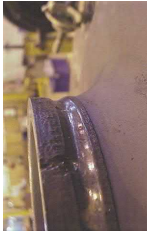
Fig. J.47 Another example of vena contracta vortex wears. Note similar helical wear pattern.
