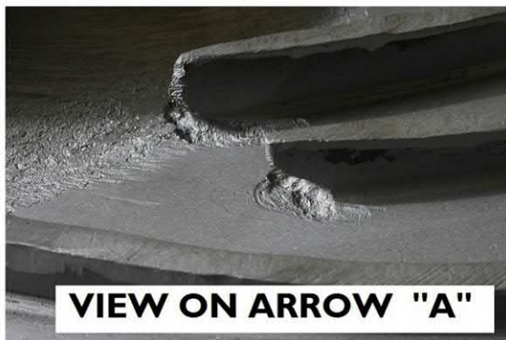
Fig. J.23 Here is a compressor impeller inlet [see also Fig. J.17 ] that shows well developed HSV damage at the vane-to -hub intersection. [Barry Hall].
