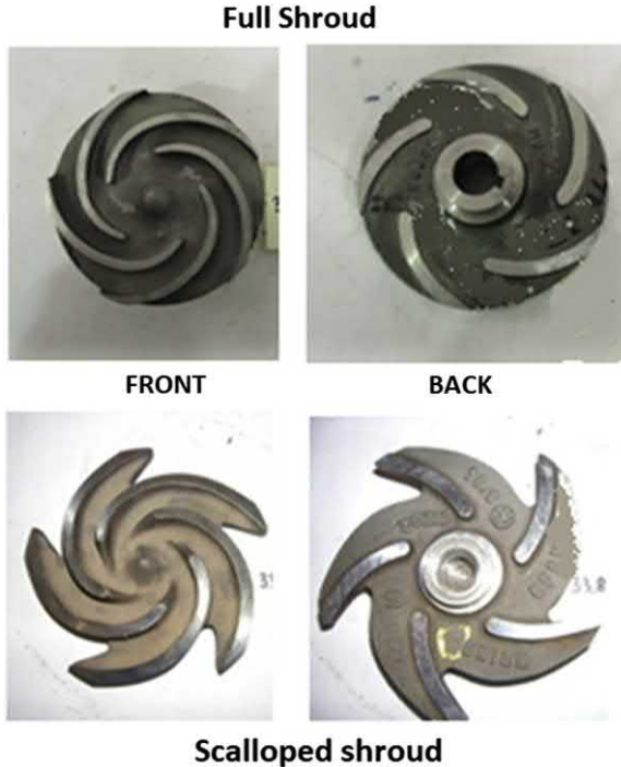
Fig. 4.15 Reducing the projected area of the back shroud by ‘scalloping’ can help to reduce axial thrust load levels.
