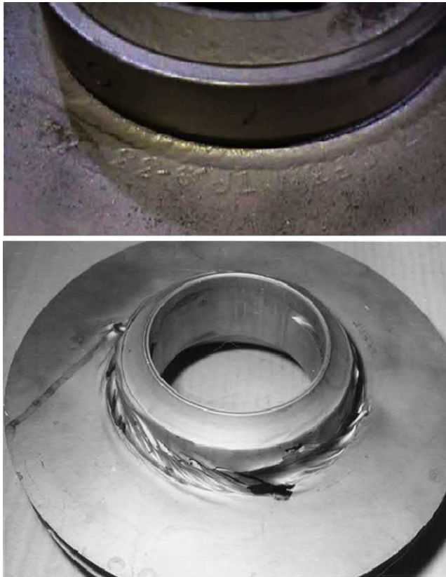
Fig. J.87 Flow exiting from the back bush clearance of larger multistage pumps can generate a stable corner vortex and hence an erosion potential.
