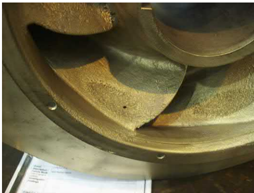
Fig. J.33 Here the cavitation damage on the front/concave visible surface has begun to penetrate through the vane thickness.
