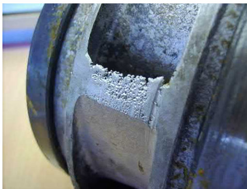
Fig. J.63 Similar cavitation-like markings to this impeller vane tip.
