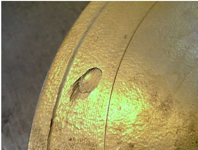
Fig. J.55 Flow erosion marks on this impeller shroud casting defect disclose outward flow of shroud boundary layer.
