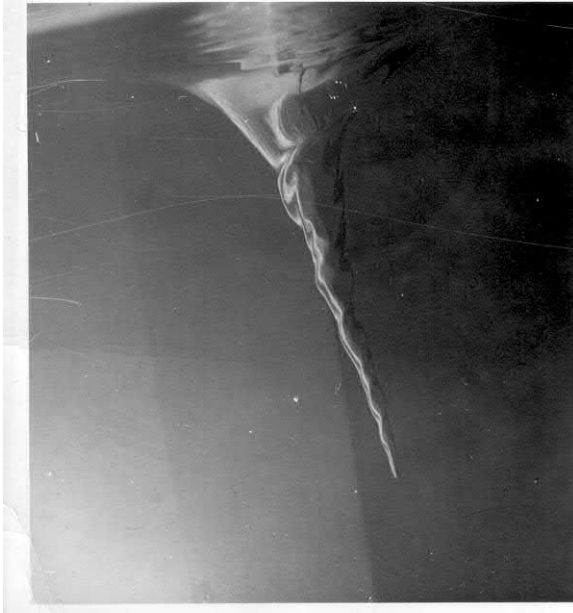
Fig. 10.29 Underwater view of air-entraining vortex forming at liquid surface. When fully developed, such a vortex allows air direct entry to the suction bell mouth [out of camera and to the right]. Photograph: SPP.
