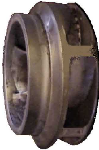
Fig. 4.19 This Single Entry impeller is near the limit for High Specific Speed radial flow designs. The radial space available [between inlet diameter D1 and outlet diameter D2 ] for efficient vane design is restricted.
