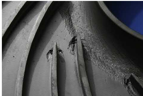
Fig. J.17 This cut away compressor impeller shows similar damage pattern on the hub surface [horseshoe vortex damage is evident at the blade root, and is discussed later — see Fig. J.23 ]. [ Barry Hall ].
