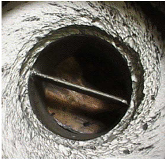
Fig. J.100 Further example of front wearing gap ring type vortex damage. Also corner vortex erosive wear at interface of casing and wear ring.
