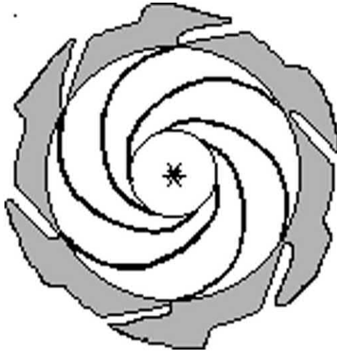
Fig. 10.20 Conceptualized velocity distribution leaving an impeller at its best efficiency flow.
