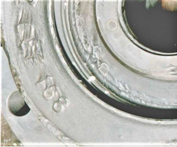
Fig. J.127 Kamm type vortex damage induced by raised cast lettering in sidewall space, between impeller and casing [see also Fig. J.56 ]. [ Sigmund Pulsometer Pumps ].
