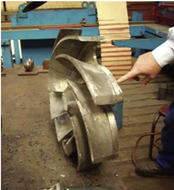
Fig. 4.11 In semi open impellers, the front shroud does not exist. Nor does the front wear ring.
