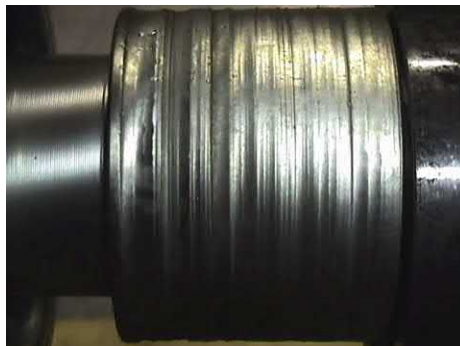
Fig. J.130 Similar throttle bush, exhibiting mixture of two body and three body wear.
