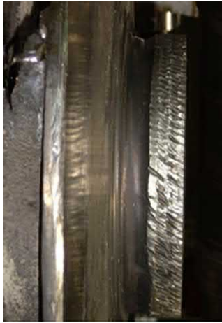
Fig. J.46 The entry vortex, resulting from a vena contracta inflicts substantial damage on the early section of the flow path. Once the flow pattern stabilise, the damage reverts to mild two body wear. The helical pattern is a result of the axial motion of the particles and peripheral motion of the wear ring surface. See also Fig. J.129 .
