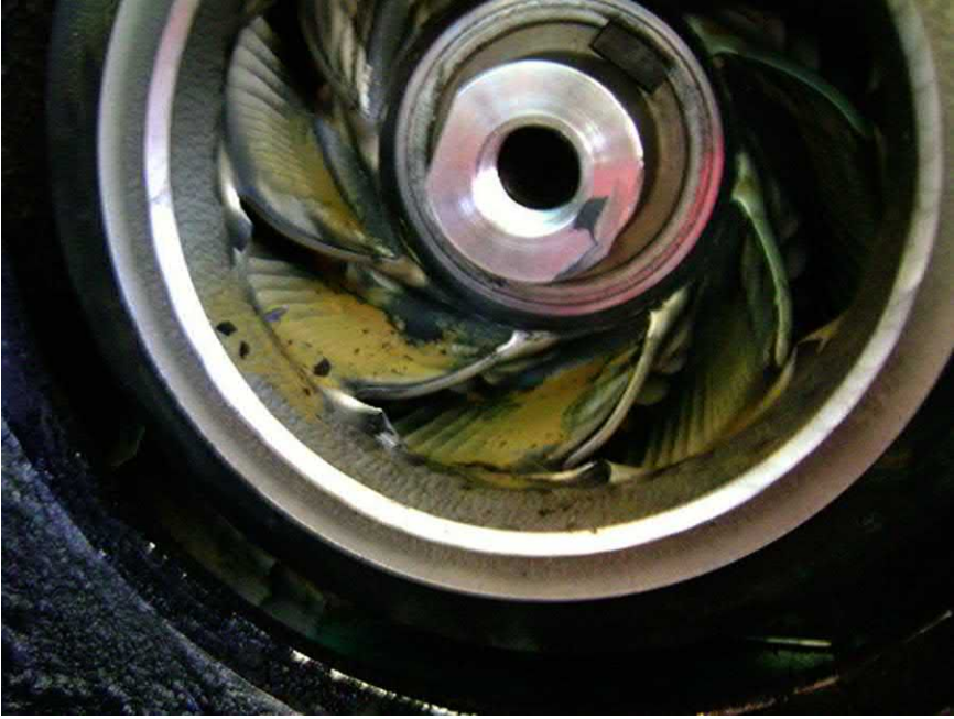
Fig. J.73 Vortices originating from the vane inlet edge [that has lost its profile due to high impact angle damage] corrugate the downstream vane surface. This constitutes low impact angle damage.
