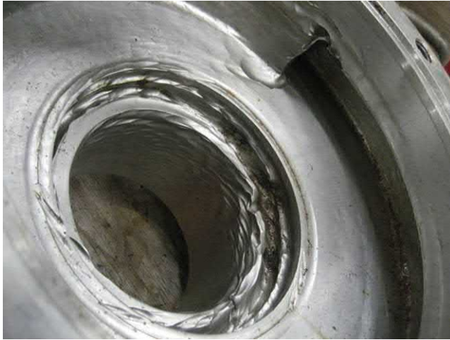
Fig. J.99 Classic Taylor—type ring vortex damage patterns related to front wear ring. Note also Horse-Shoe Vortex damage around casing cutwater/lip. The impeller has been operating on the boundary of its Backflow regime. Consequently, particles emerging from the impeller wear ring have been carried upstream a little. Finally, see that there is corner vortex damage to the casing at its interface with its wear ring outer diameter. This is because the wear ring was not flush with the casing wall [see also Fig. J.49 ].
