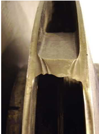
Fig. J.59 Advance twin vortex damage to this single suction API 610 Process pump handling Catalyst fines.
