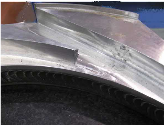
Fig. J.124 Bend fatigue failure induced, by low flow pressure pulsations in this process pump.
