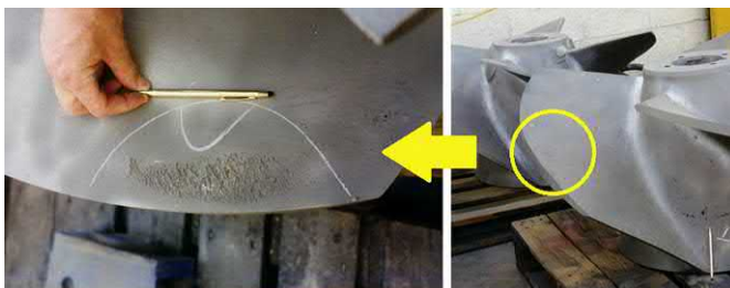
Fig. J.84 Equivalent gap flow damage on a mixed flow impeller.
