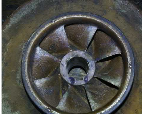
Fig. J.25 Light cavitation marks on concave [visible] vane surface indicate classic off-design flow damage. This image shows how, in a pump operating near to its design flow, cavitation damage decreases with radius from the shaft. It is disclosed by the wedge-shaped pattern. This is principally because the peripheral velocity also decreases with radius.
