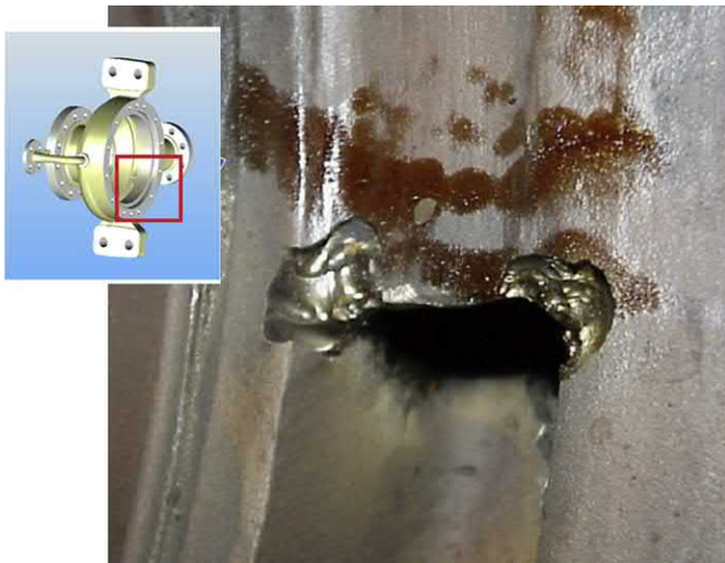
Fig. J.9 View of a volute cutwater [lip] subject to Horse Shoe Vortex [HSV] wear at the junctions with the casing sidewalls. It is clear that the general casing surface has been otherwise largely unaffected by the suspended solids [The original casting surface finish is still visible.]. There is little if any evidence of low impact angle damage on the other parts of the wetted surface.
