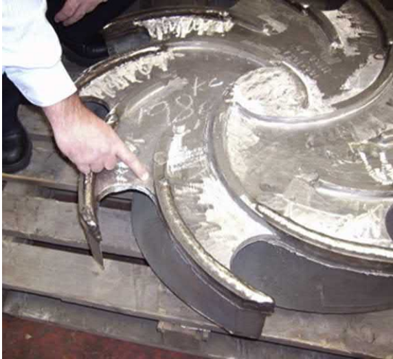
Fig. 4.14 Back pump-out vanes are more efficient if they somewhat follow the spiral shape of the main vanes. Simple radial paddle vanes are sometimes used instead, but they may promote accelerated erosion effect if dirty liquids are being pumped.
