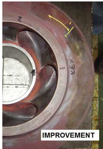
Fig. J.21 Another example of improved resistance to Horseshoe Vortex. Note how the intersection angle between vane leading edge and both hub/shroud disk is now very much less than 90 degrees. In most cases the intersection with the shroud disk is more important than with the hub, because the liquid velocities are higher there. [Weir Engineering Services].
