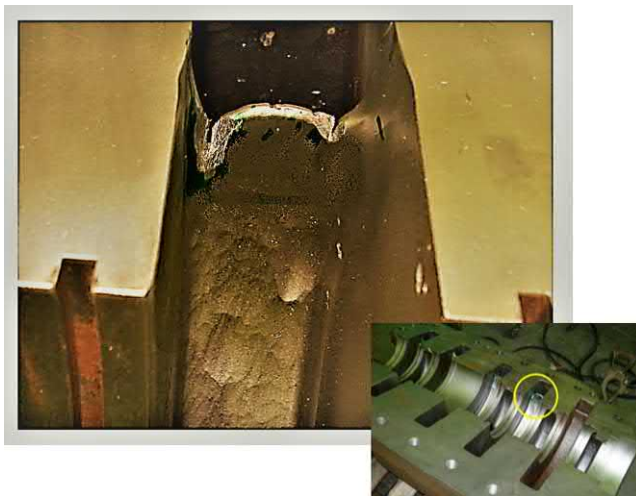
Fig. J.108 View of the volute casing cutwater lip on an axially split case pump. Again notice the horse shoe vortex damage near the junction point.
