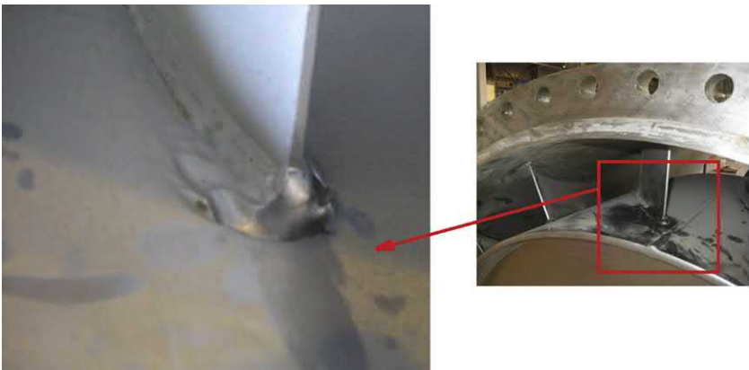
Fig. J.122 Similar Horse Shoe Vortex damage; this time in a mixed/axial flow diffuser intersection with hub.
