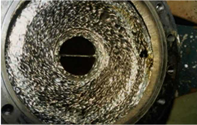
Fig. J.97 This is a classic example of low impact angle damage. [David Brown Pumps].
