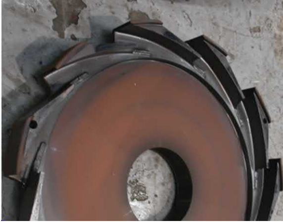
Fig. J.123 Flow and pressure pulsation caused by the typically saw-tooth exit distribution [see Fig. J.63 ] induce fluctuating forces on the collector vanes. The intensity of these forces increase as the flow departs from its design condition. The forces apply a bending moment, which is a maximum at the hub-disk intersection. This is where fatigue failure most often occurs, resulting in this sort of breakage.
