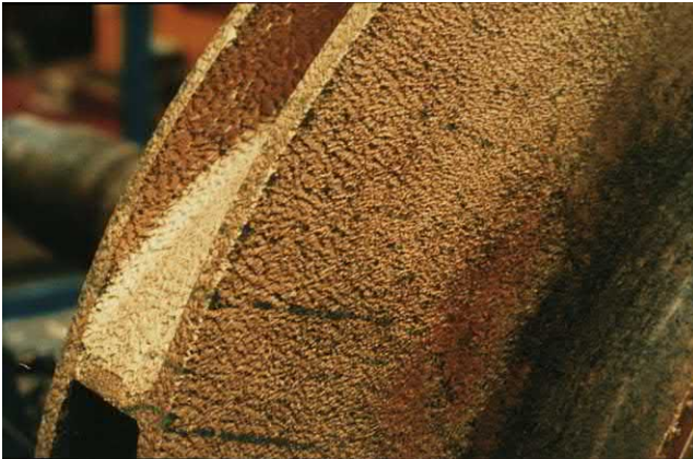
Fig. J.7 This shows corresponding low impact angle damage to the outer shroud wall of an impeller. Note that the damage rates appear to increase with radius from the shaft axis. This is because the impeller angular velocity also increases with radius.
