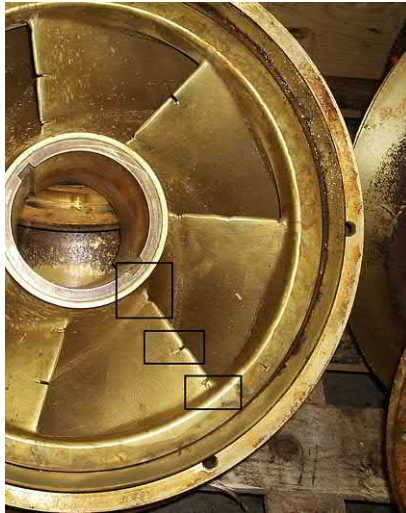
Fig. J.41 Tensile shrinkage forces in the cooling casting can induce micro cracks on the vane edge. These can be the centre, as here, for high impact angle erosion damage. [Andrew Percy] .
