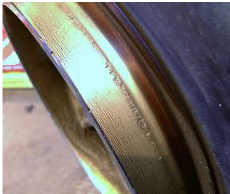
Fig. J.48 Less severe vena contracta vortex wear. Little sign of helical wear means that the particles have been small relative to the flowpath gap and so only two-body wear has occurred.
