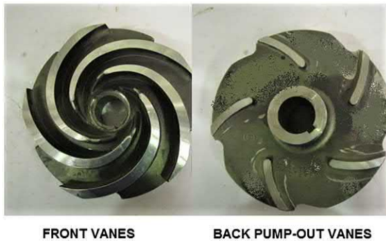
Fig. J.76 View of Front and Back vanes of Radial flow semi open and open impellers. The back vanes shown here more or less mirror the shape of the front vane spiral and extend out to the same maximum diameter. In some case, the back vanes are simply straight and radial. Occasionally, vanes of either type do not extend right to the same maximum diameter.
