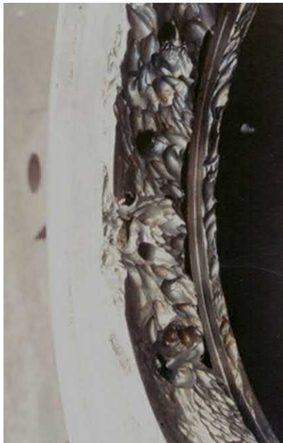
Fig. J.51 This flushed wear ring shows how the injection disturbance is profound and is likely to create many cases of high impact angle contact within the flowpath gap.
