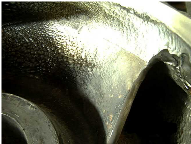
Fig. J.8 This image shows high impact angle damage to the leading edge of an impeller vane. It has lost its streamlined shape and become rather blunt. It has also taken on a typical polished appearance. [David Brown Pumps].
