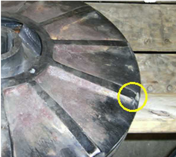
Fig. J.79 Even if the downstream shape of the back pump out vanes is streamlined in an attempt to suppress Kamm type vortices [as here], a form of Von Karman type vortex can form at the very tip. If these vanes do not extend to the maximum, then this can cause significant damage — see next image.
