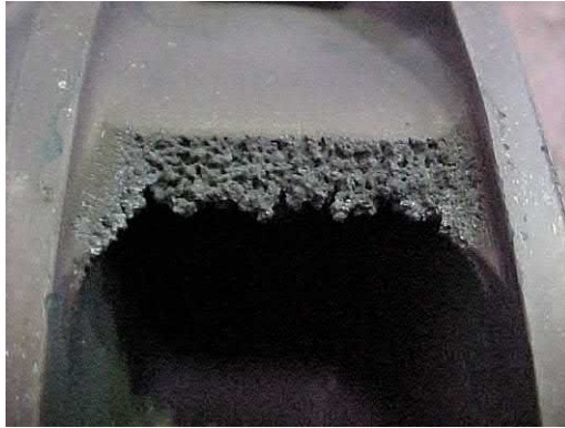
Fig. J.62 Cavitation-like markings on outlet edge of impeller vane of this single suction booster pump.
