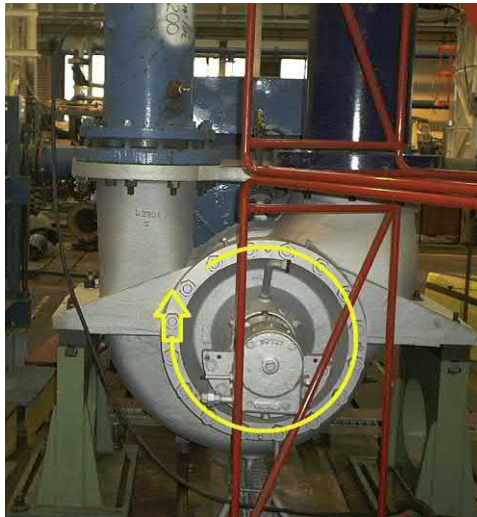
Fig. 8.37 Double suction between-bearings process pump.
