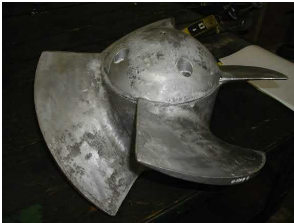
Fig. 10.8 The correct rotation for this impeller is clockwise as viewed. Generally, the convex blade surface faces the approaching flow.
