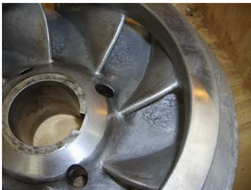
Fig. J.36 Damage on the reverse vane side and also the hub disk [see also Fig. J.31 ].
