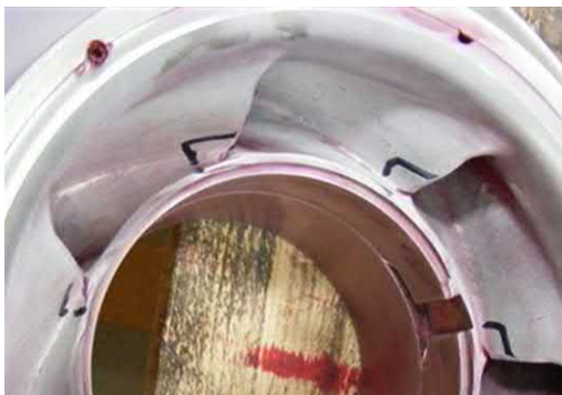
Fig. J.44 The 'nick' in the vane edge at its intersection with the hub is unlikely to be cavitation and more likely to be erosion at the site of a micro crack. The root cause is identical to Fig. J.41 .
