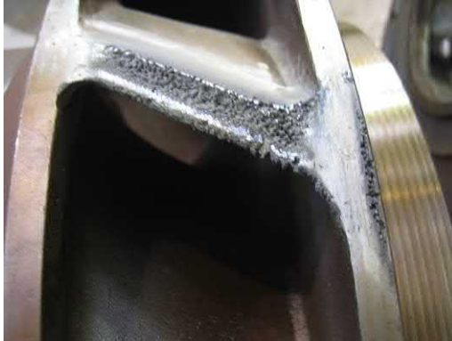
Fig. J.64 Again cavitation-like markings to the vane outlet tip. Unusually, this also exhibits damage to the rear [hub] shroud of this single entry impeller. The pressure distribution in this zone is quite complex.
