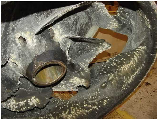
Fig. J.14 This bronze impeller has failed largely due to corrosion. It was successfully replaced by an impeller made of Duplex Stainless Steel. There is little, if any, evidence of particle erosion. [ Weir Pumps ].
