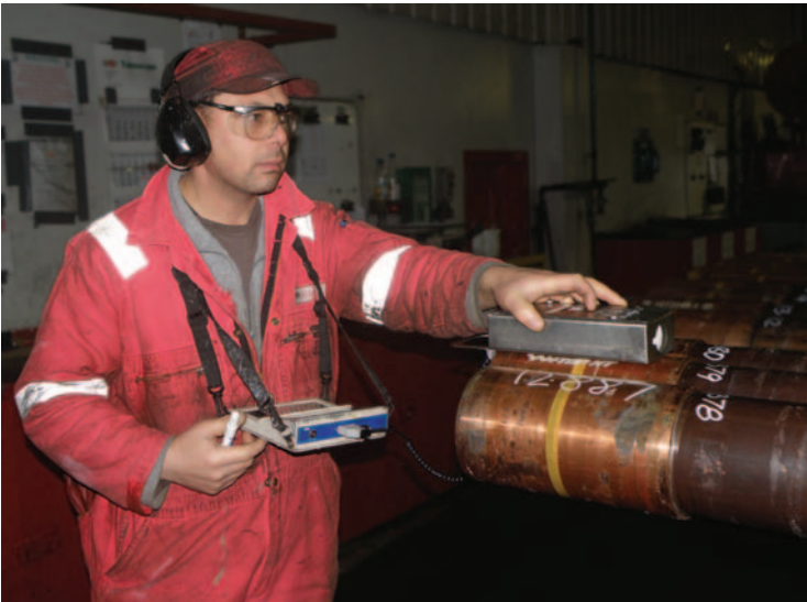
Figure 11.18 Measuring pipe by laser before shipment to the wellsite.
