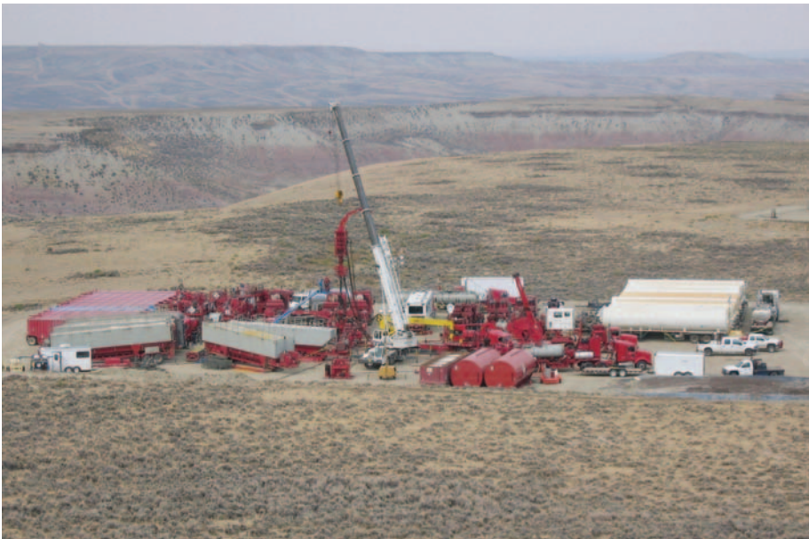
Figure 2.77 Pumping layout for large stimulation treatment, Wyoming, United States (photograph courtesy Michael C. Romer, ExxonMobil).
