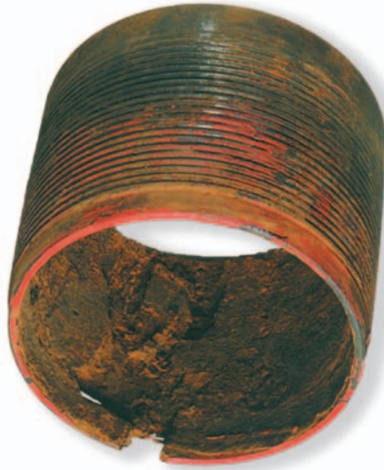
Figure 8.12 Corroded water injection carbon steel tubing.
