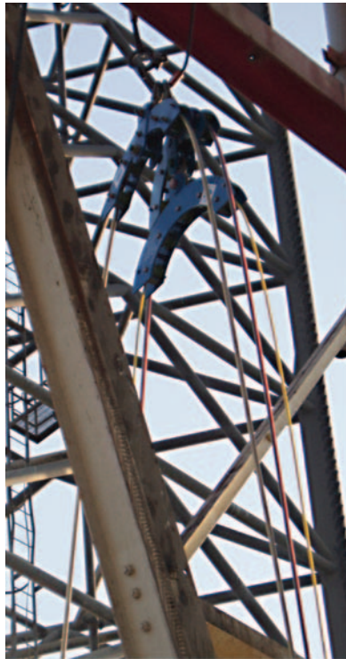
Figure 11.24 Three control lines and sheaves.
