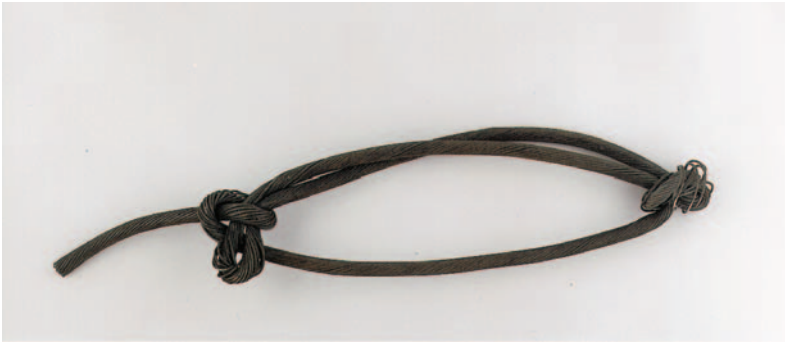
Figure 2.46 Knot in wireline caused by excessive underbalance.
