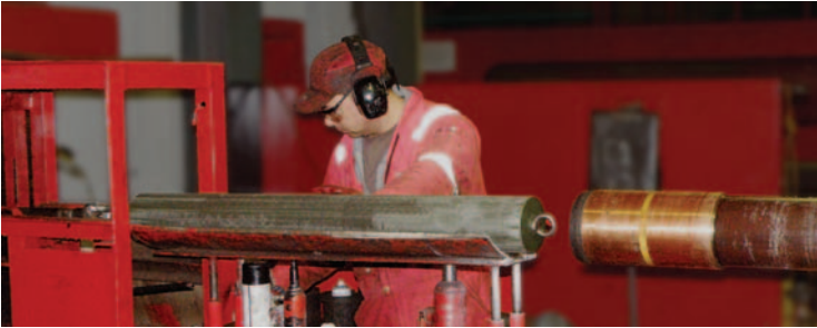
Figure 11.17 Drifting tubing before shipment to the wellsite.
