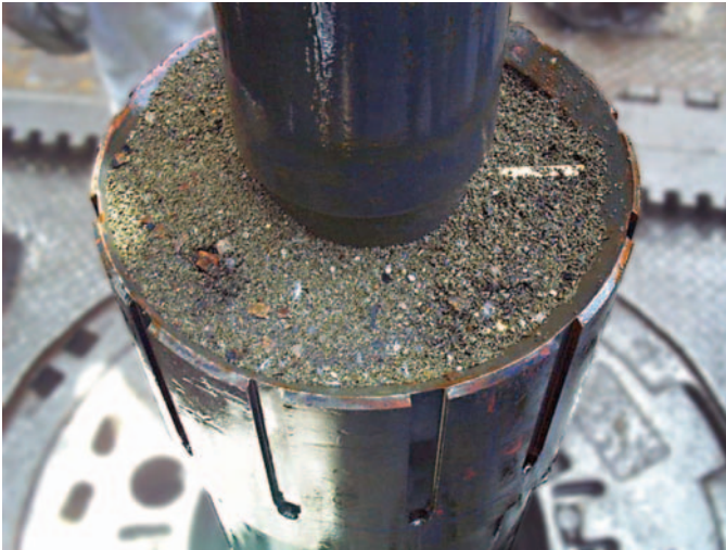
Figure 11.4 Full junk basket assembly (photograph courtesy of Bilco Tools, Inc.).
