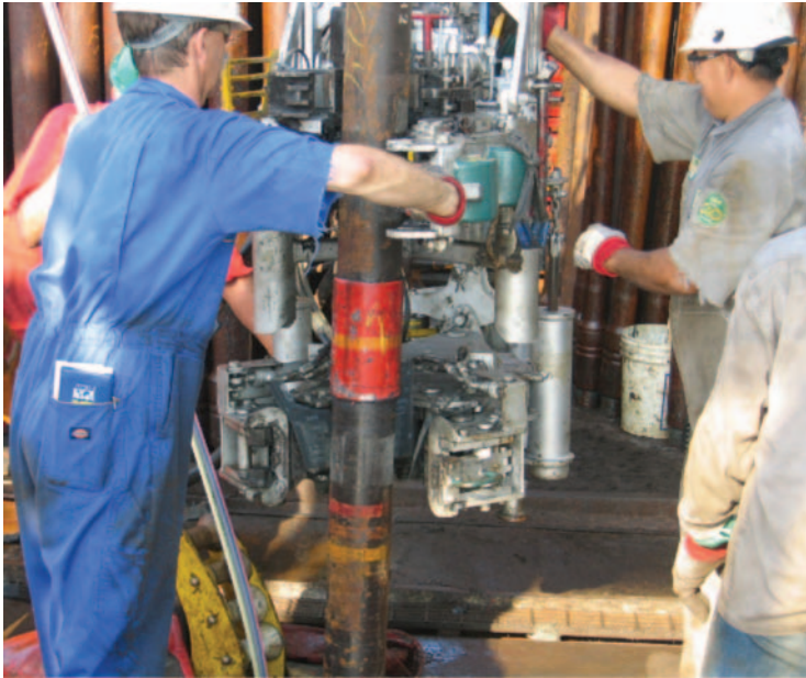
Figure 11.21 Preparing to make-up chrome tubing.
