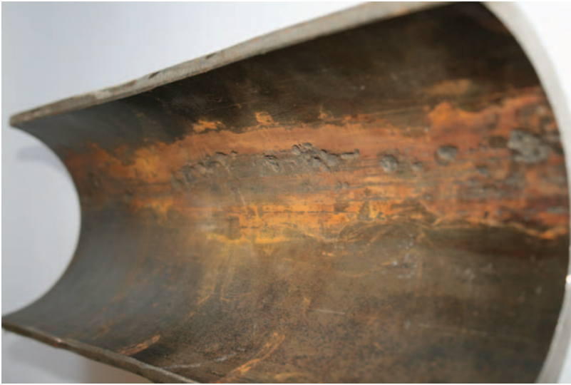
Figure 8.6 Corroded 13Cr tubing.
