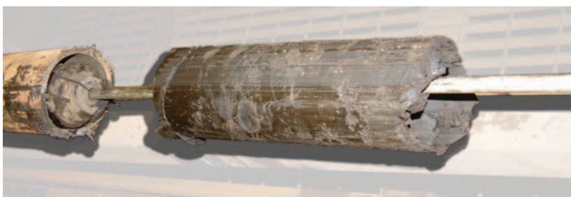
Figure 7.14 Wax recovered with a completion – (photograph courtesy of BP Exploration Ltd.).
