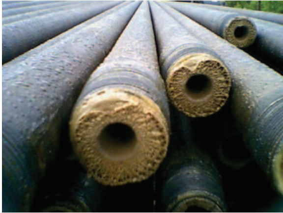
Figure 7.4 Barium sulphate scaled-up tubing example (photograph courtesy of Tom Grant and Johnny Smith, Gaither Petroleum).
