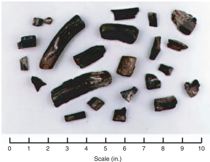
Figure 11.1 Debris from the milling of a packer.
