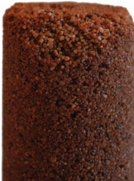
Figure 2.83 Fully cured resin coated proppant.
