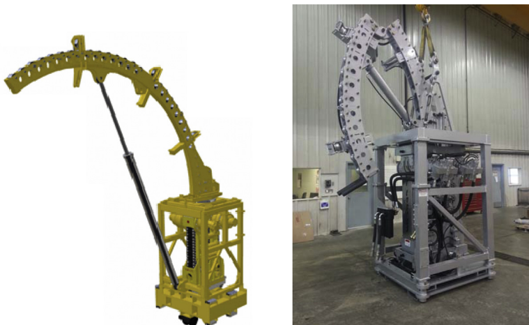
Figure 10.16 Coiled tubing injector heads (with guide arch). Source: Image courtesy of CT Logics.
