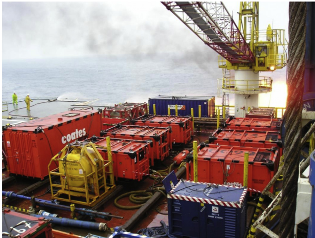
Figure 12.15 This well test required six air compressors.
