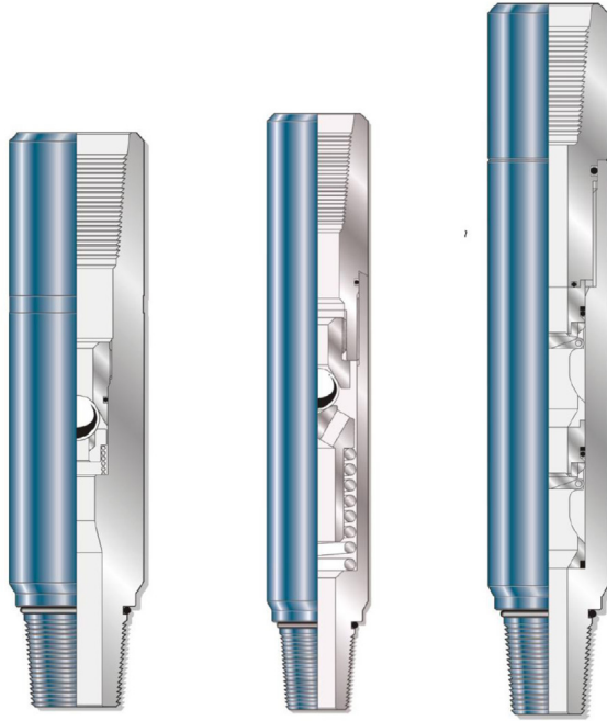
Figure 11.19 Ball check (left) ball and seat BPV (center) and dual flapper valve (right).
