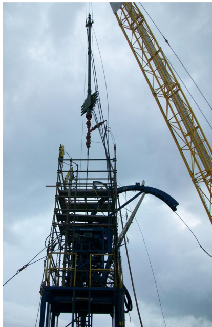
Figure 10.45 Rigging up above cut stuck coiled tubing. A perfect illustration of why it is better not to get stuck in the first place—think well control!
