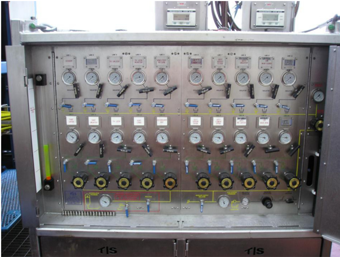
Figure 13.27 Workover control system for a direct hydraulic control THROT/SSTT umbilical during a well completion.
