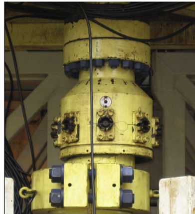
Figure 15.11 Helix quick makeup connection bore selection spool. Photographs courtesy of Helix Well Ops.
