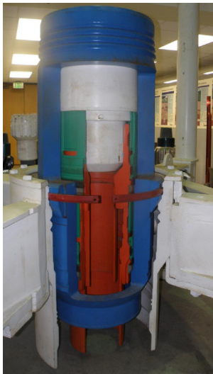
Figure 13.9 10,000 psi 18 3/4 in. wellhead cutaway to shows the casing hangers.
