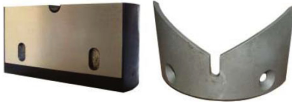
Figure 9.22 Braided cable ram insert and wire guide.
