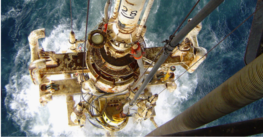
Figure 13.1 Running a subsea blow out preventer.
