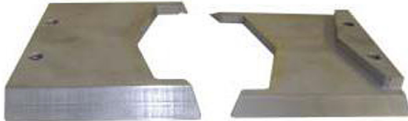
Figure 9.25 Wire cutting blades for a shear seal blow out preventer.
