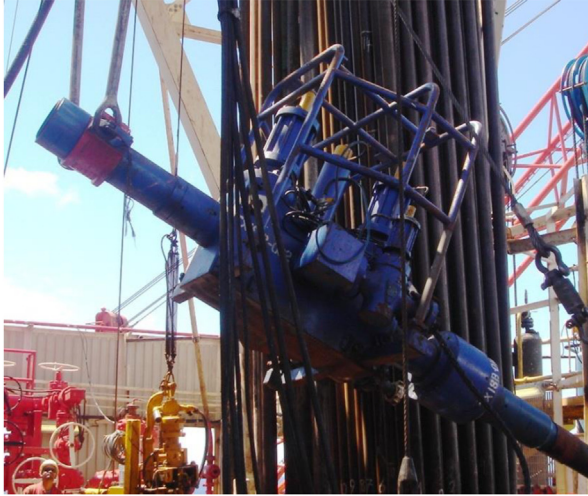
Figure 14.10 Picking the Surface Test Tree. The bails and elevator seen in the picture are connected to the base of the lift frame.
