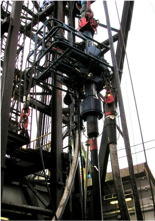
Figure 12.3 A surface test tree (flowhead) and coflex hose in use on a semisubmersible rig.
