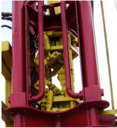
Figure 11.4 Inverted (top) and conventional (lower) stationary slips.
