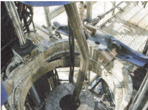
Figure 11.6 Buckled tubing—the result of not using a guide tube. Photo reproduced with permission of the SPE (from SPE paper 115534).
