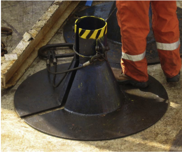
Figure 15.15 The “Witches Hat”—used for assembling the wireline tool string. Photograph courtesy of Helix Well Ops.
