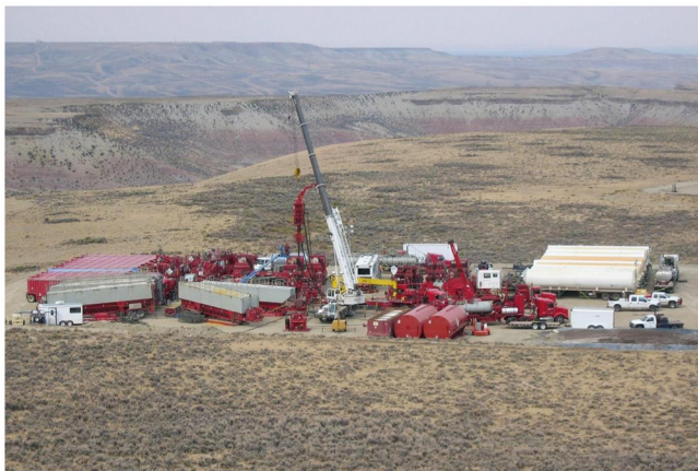
Figure 8.1 Some pumping operations require a large amount of equipment. Propped frac in progress, Wyoming, USA.
