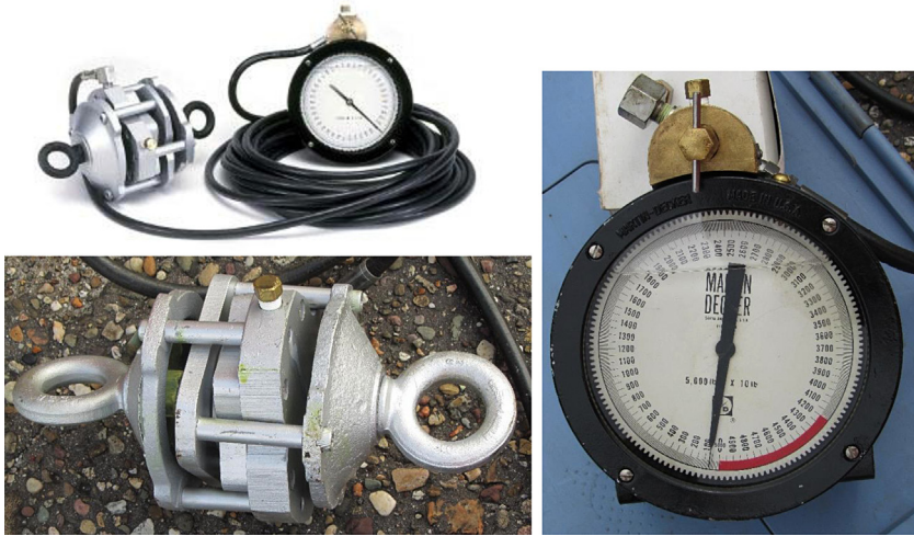
Figure 9.8 Martin Decker type weight indicator. Photograph courtesy of Bob Baister.
