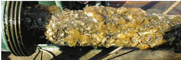
Figure 5.5 Partially hydrated polymer (fish eyes). Very damaging. Source: Image courtesy of George King.
