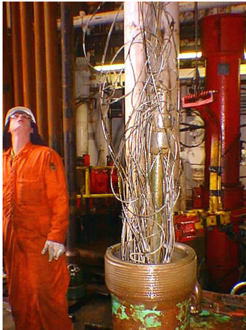
Figure 9.56 What you hope not to see. Multiple wire strands compromise the blow out preventer and complicate the fishing operation.
