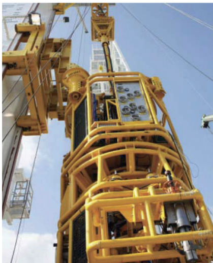
Figure 15.13 7 3/8 in. Subsea intervention lubricator. Source: Image and photograph courtesy of Helix Well Ops.
