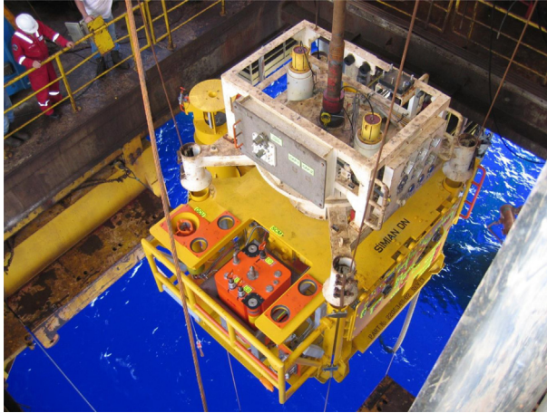
Figure 13.23 Running a horizontal tree on drill pipe. Photo courtesy of Danny Thomas.
