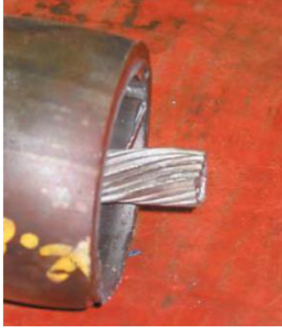
Figure 10.10 After the cut. This reel was run with internal e-line (smart coil).
