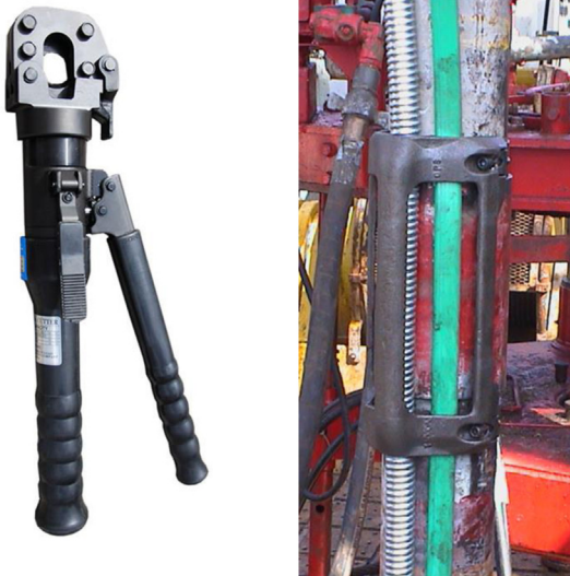
Figure 7.32 Self-contained hydraulic cutter (left) and multiple flat-packs (right).
