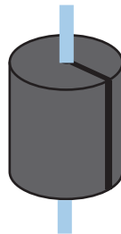
Figure 9.48 Packing is cut along its length through half the diameter and pushed onto the wire.
