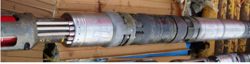
Figure 3.23 Permanent releasable packers ready for deployment in an intelligent completion. Note the various feed-through conduits serving hydraulic and instrument cables.
