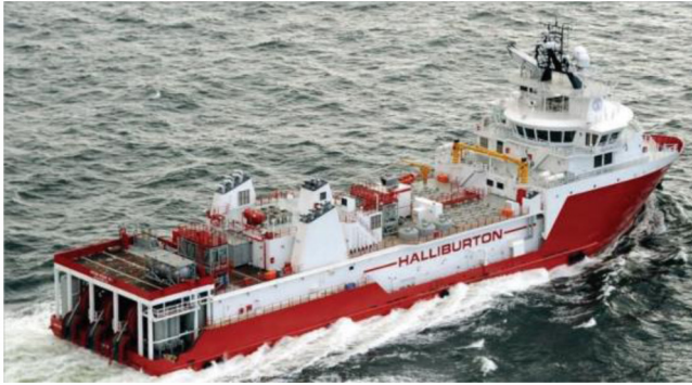
Figure 8.15 Coflex hose reels clearly visible on the stern (back) of a frac boat.
