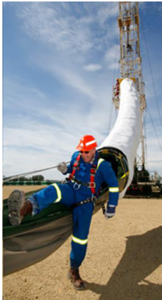
Figure 11.8 Fireproof escape chute—used where the work basket is high above ground level. Image courtesy of Foxxhole™ Escape Sytems.
