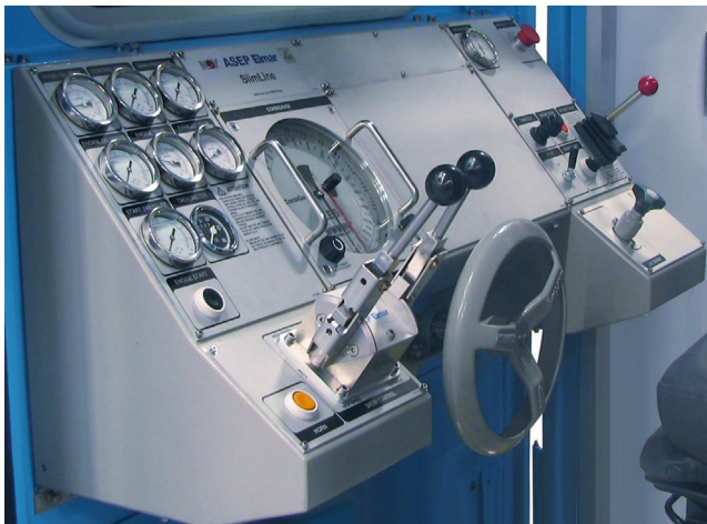
Figure 9.6 Wireline unit control panel (double drum unit). Image courtesy of NOV Elmar.
