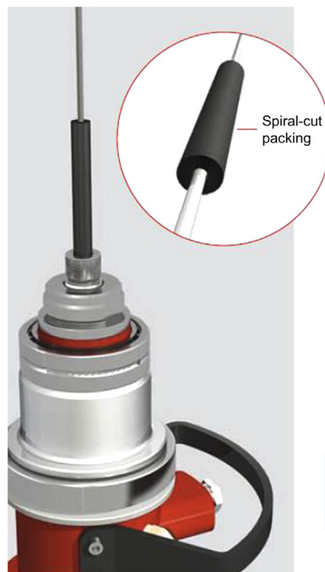
Figure 9.49 NOV Elmar spiral cut packing is a safer alternative—allowing packing to be replaced whilst wire is still in the well. Image courtesy of NOV Elmar.
