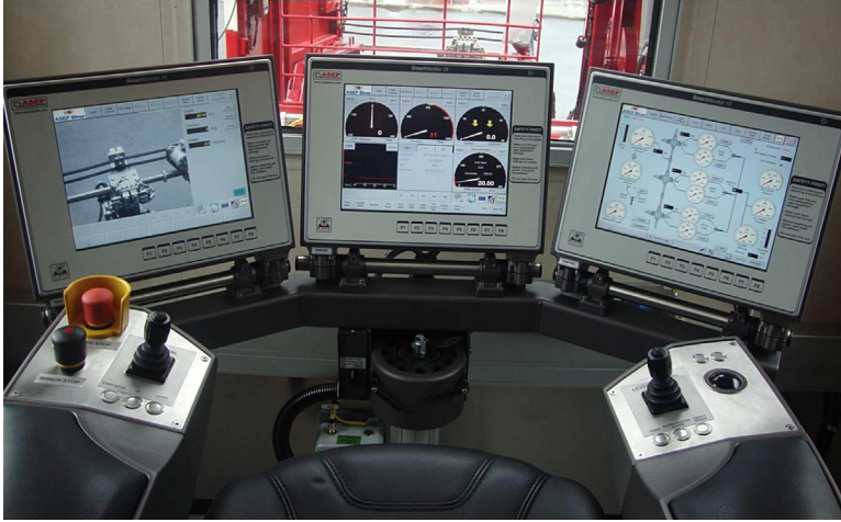
Figure 9.7 Modern wireline units have touch screen displays that control multiple functions including the winch, power pack, pressure control equipment, and in some cases well monitoring. Image courtesy of NOV Elmar.
