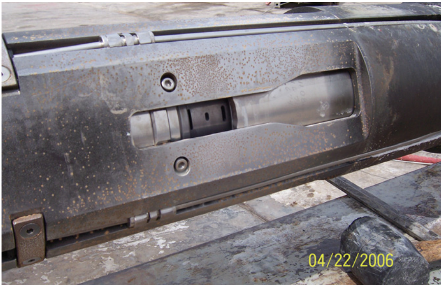
Figure 8–12 Down-hole control valve at fixed-open position. (Courtesy WellDynamics)
