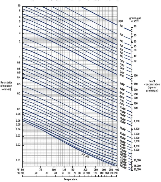
Conversion approximated by  $R_2 = R_1 [(T_1 + 6.77)/(T_2 + 6.77)]^\circ F$  or  $R_2 = R_1 [(T_1 + 21.5)/(T_2 + 21.5)]^\circ C$
