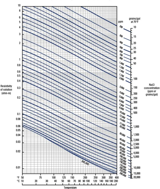
Conversion approximated by  $R_2 = R_1 [(T_1 + 6.77)/(T_2 + 6.77)]^\circ F$  or  $R_2 = R_1 [(T_1 + 21.5)/(T_2 + 21.5)]^\circ C$
