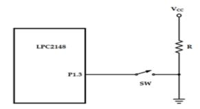
Identify the mistakes if any, that Mr. Vivek has done in this arrangement. Produce the correct diagram of the interfacing and light an LED to identify whether the switch is pressed. If the switch is pressed, the LED should glow. Write the C code for the same. (C.O.No. 4) [Application]
