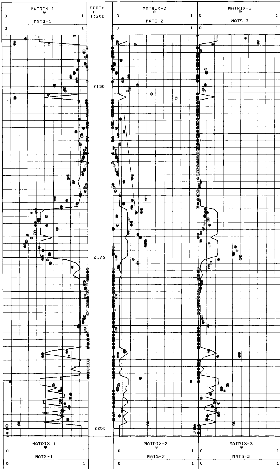
Fig. 2. Single BPNN output compared to core data.
