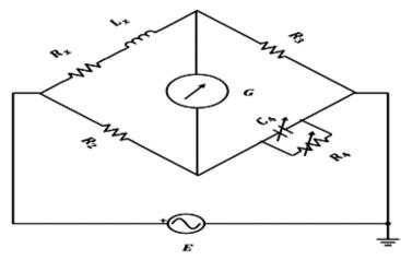
b) A Maxwell bridge is a modification to a Wheatstone bridge used to measure an unknown inductance in terms of calibrated resistance and inductance or resistance and capacitance. Explain the types of Maxwell's bridge, which are used to determine the self-inductance of the circuit.
